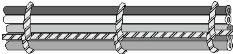
Figure 2-39.—Conductor lacing.
