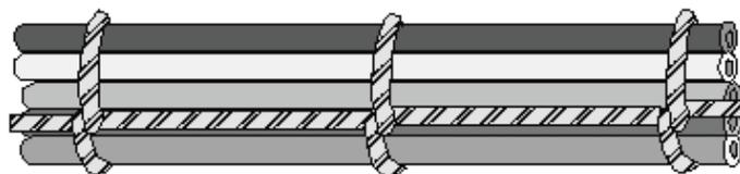
**Spot Ties**—Spot ties are used when cable supports are used that are more than 12 inches apart.
