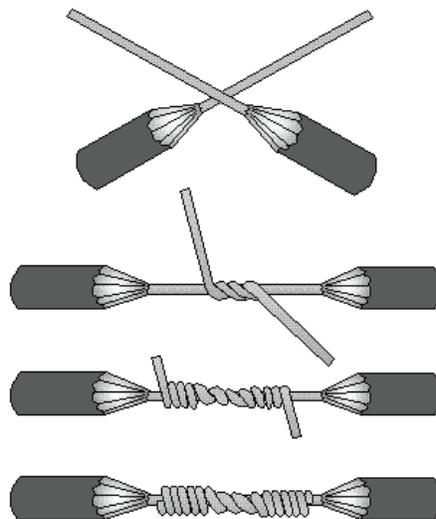
**Staggered Splice**—The staggered splice is used on multiconductor cables to prevent the joint from being bulky.
