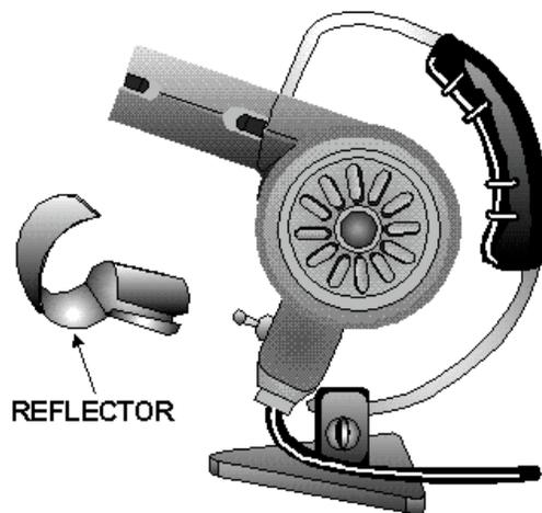
Figure 2-15.—Typical hot-air gun.
