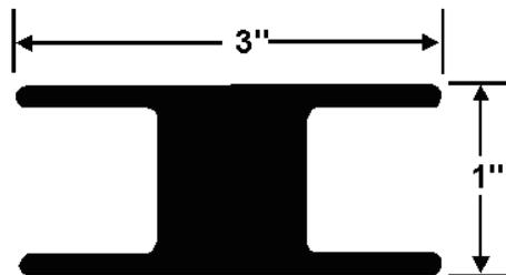
Figure 2-40.—Lacing shuttle.
