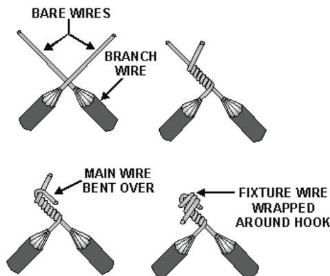
Figure 2-8.—Fixture joint.
