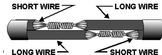
Figure 2-6.—Staggering splices.
