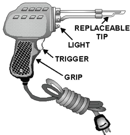
Figure 2-31.—Soldering gun.
