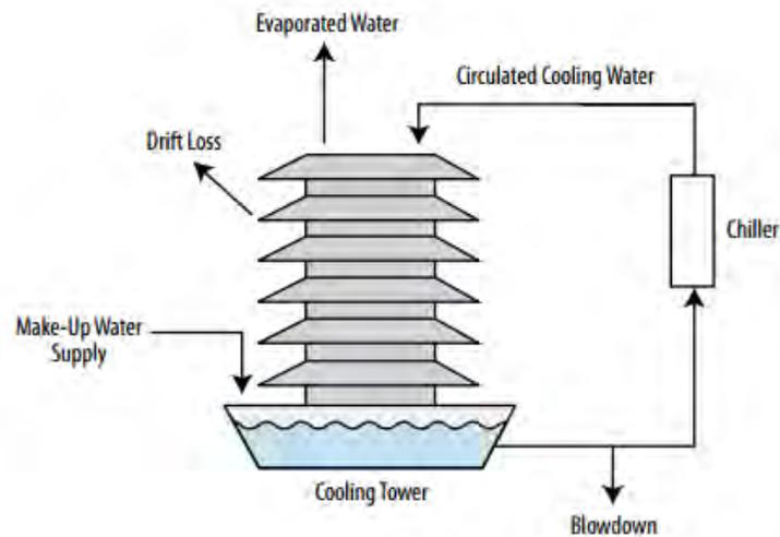
Efficient drift eliminators and effective leak/overflow detection should minimize water losses from drift and leaks. If that is the case, make-up water for a well-managed cooling tower is essentially only based on evaporation and blowdown rates.
