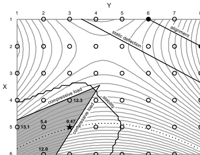
**Figure 26 Design space cross section showing unconstrained objective, discrete grid, contour lines, constraint boundaries, feasible domain (shaded), and feasible discrete designs with their transmissibilities; the ★ shows the discrete optimum.**
