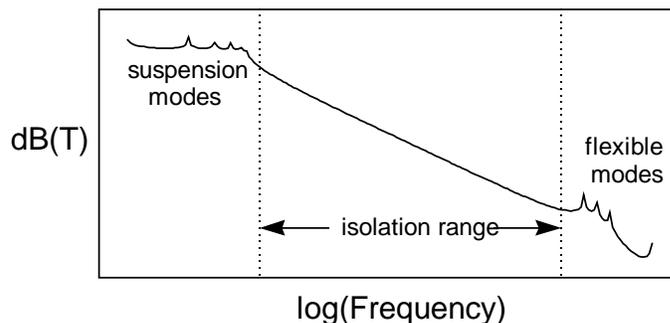
Figure 2 Typical transmission characteristics of isolation system.
