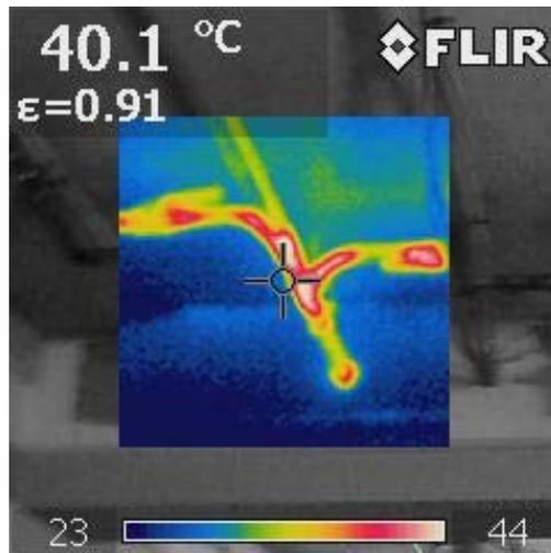
**Fig. 6 - Image of a Domestic Hot Water Pipe**
