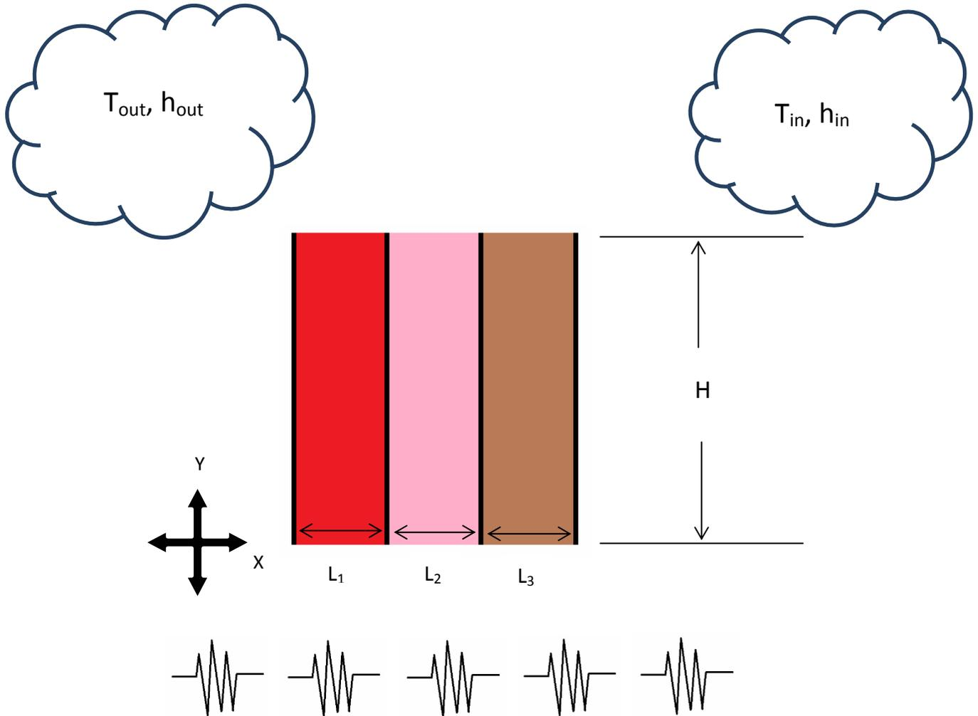
The resistance of this wall is a combination of three materials in series and can simply be added up for a total R-Value. If there was a window or some other fenestration, then the R-value of that would be in parallel with the materials making up the wall and will be calculated by:
