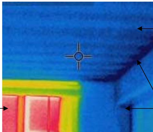
Dark blues lines represent the reduced thermal resistance of the ceiling frame construction.
