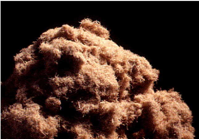
Figure 10–9. Fibers can be made from many lignocellulosics and form the raw materials for many composites, most notably fiberboard. Fibers are typically produced by the refining process.
