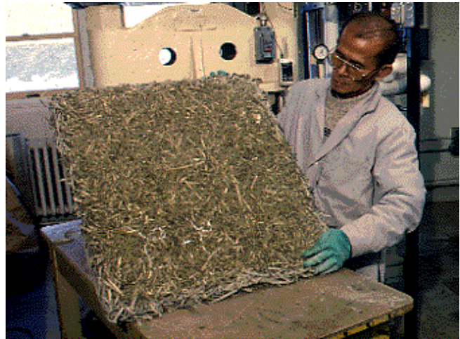
Figure 10–15. Laboratory-produced low-density, cement-bonded composite panel. Full-scale panels such as these are used in construction.
