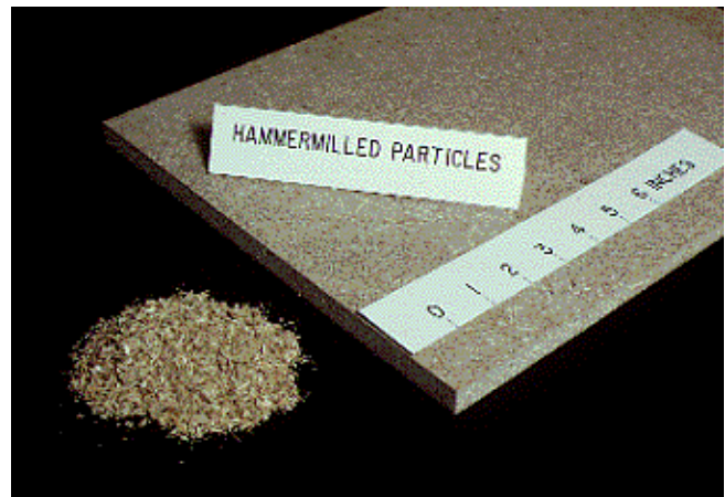
Figure 10–7. Particles, which are sometimes produced by hammermilling, are used to produce composites such as particleboard.
