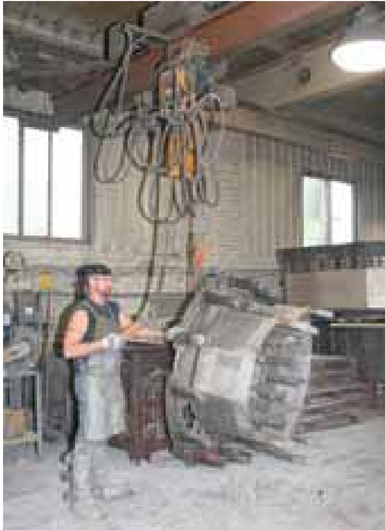
Figure 9. Large Castings Being Removed from Mold 1
