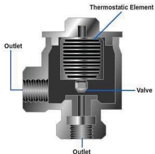
**Figure 10-13 – Thermostatic trap.**
