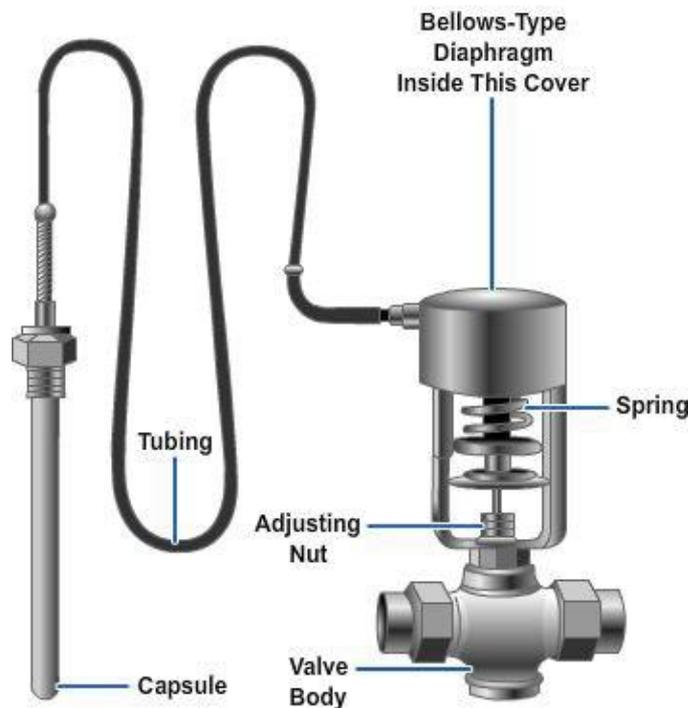
**Figure 10-22 - Temperature-regulating valve.**
