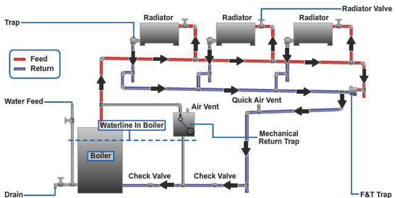
Figure 10-6 – Two-pipe vapor system with a return trap.
