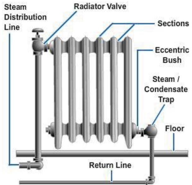
Figure 10-9 – Cast-iron radiator.
