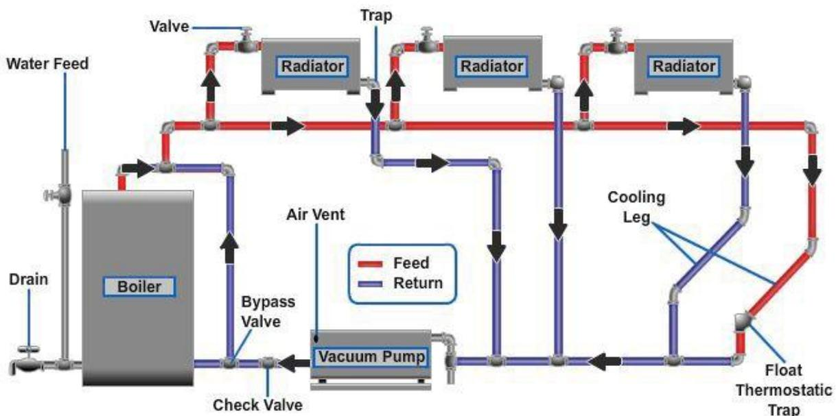
Figure 10-8 – Two-pipe vapor system with a vacuum pump.
