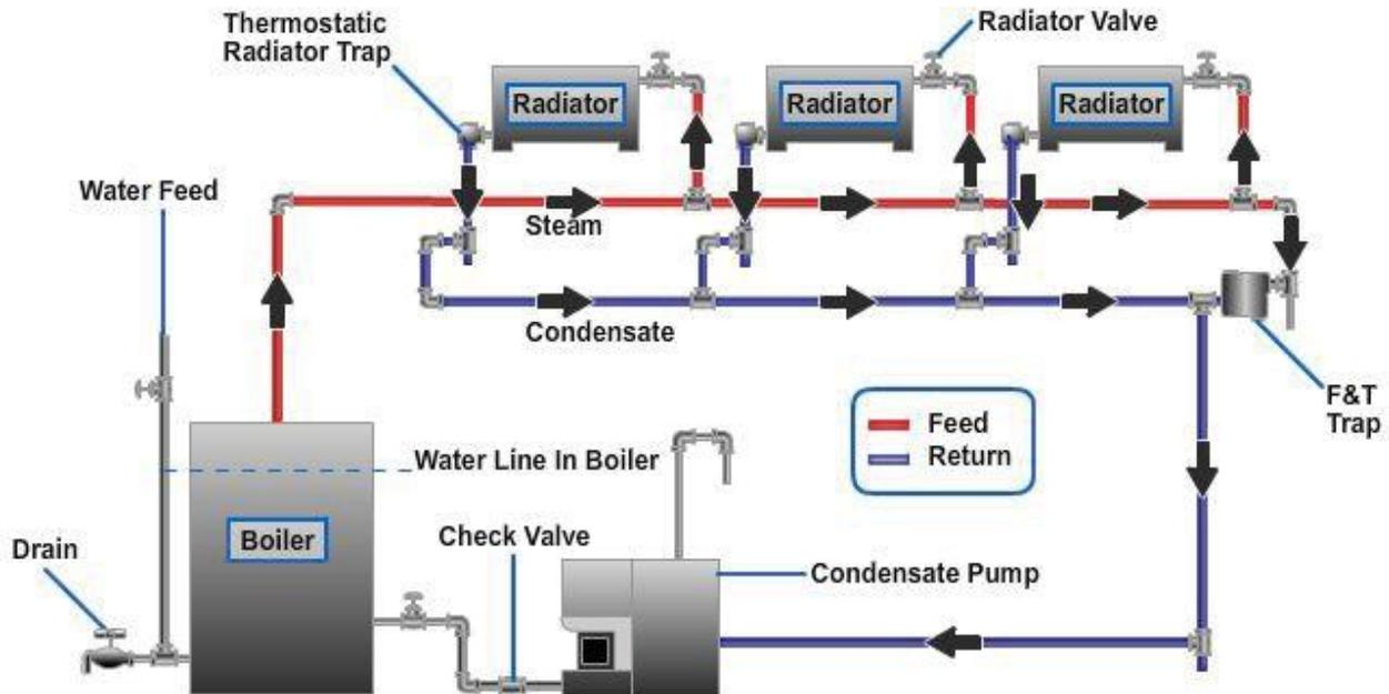
**Figure 10-7 – Two-pipe vapor system with a condensate pump.**
