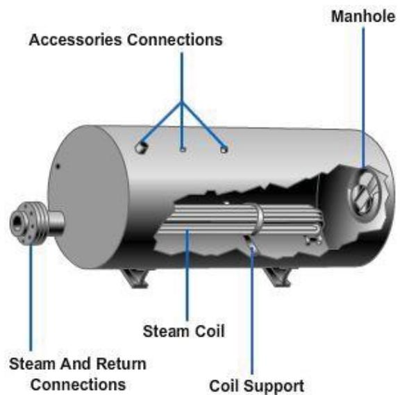
**Figure 10-20—Storage-type water heater.**
