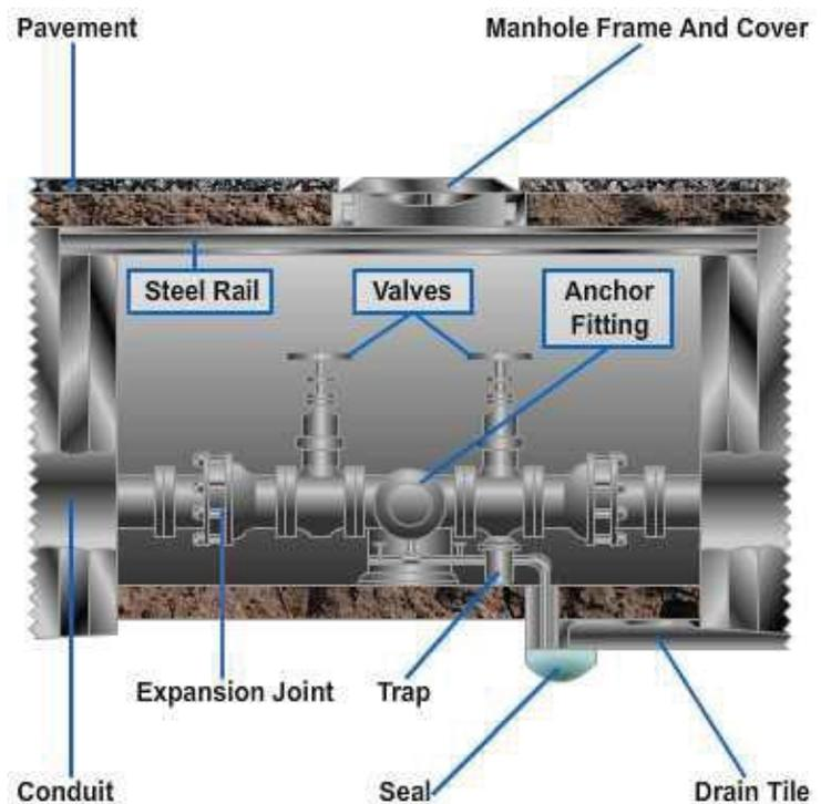
Figure 10-2 — Typical manhole for distribution system.
