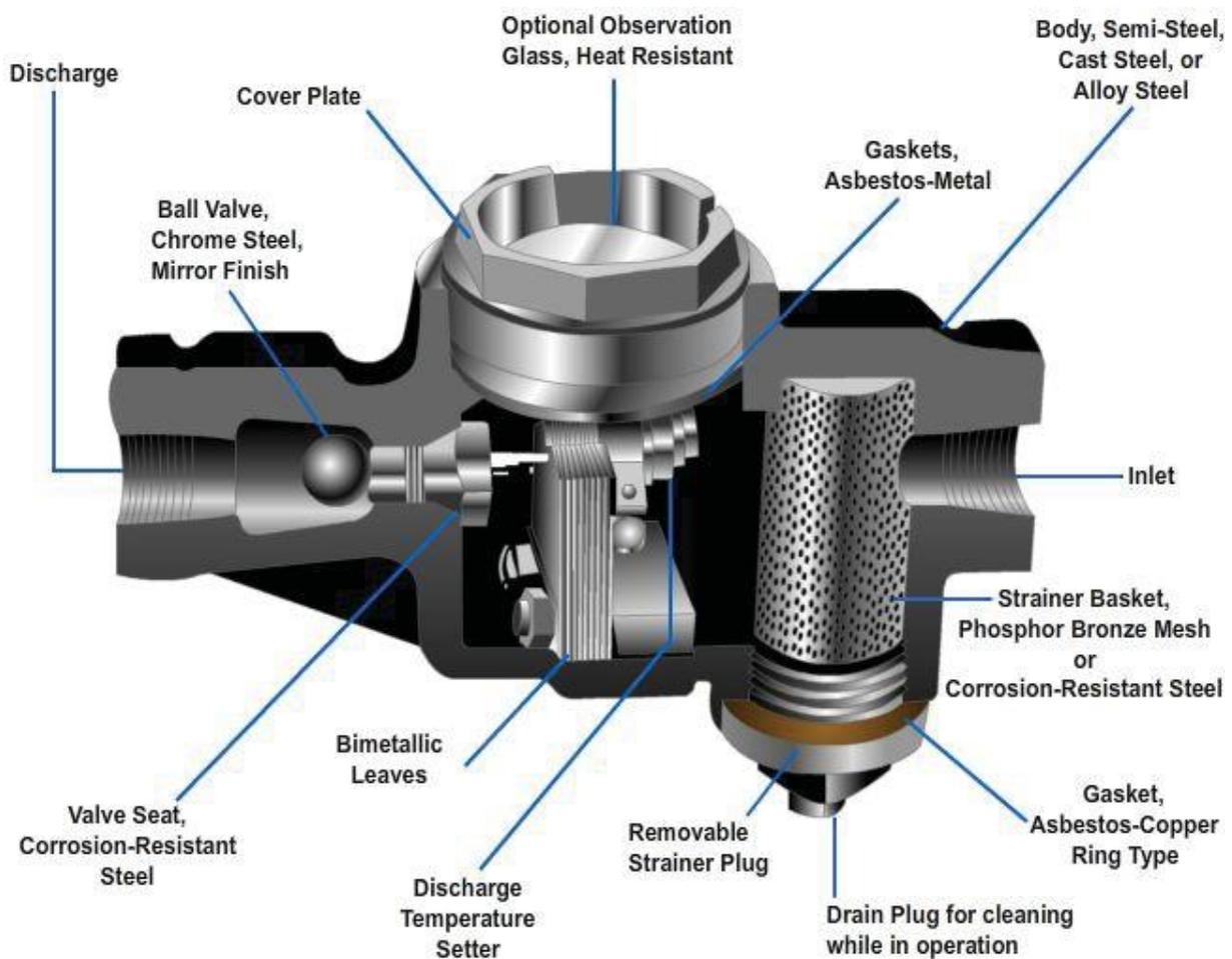
**Figure 10-18-Bimetallic-element steam trap.**
