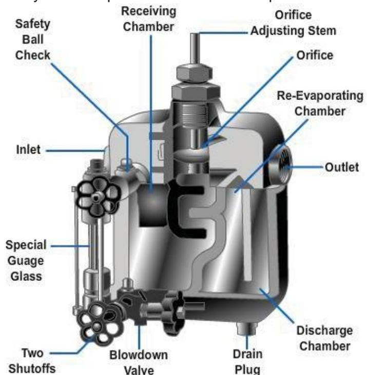
**Figure 10-17 – Throttling trap.**
