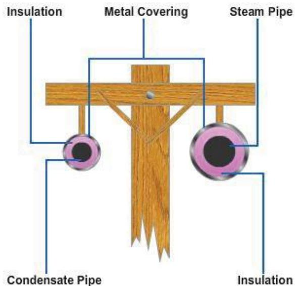
**Figure 10-4 – Steam and condensate lines supported by poles.**
