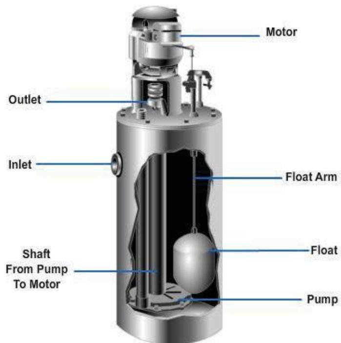
**Figure 10-23 – Condensate return pump.**
