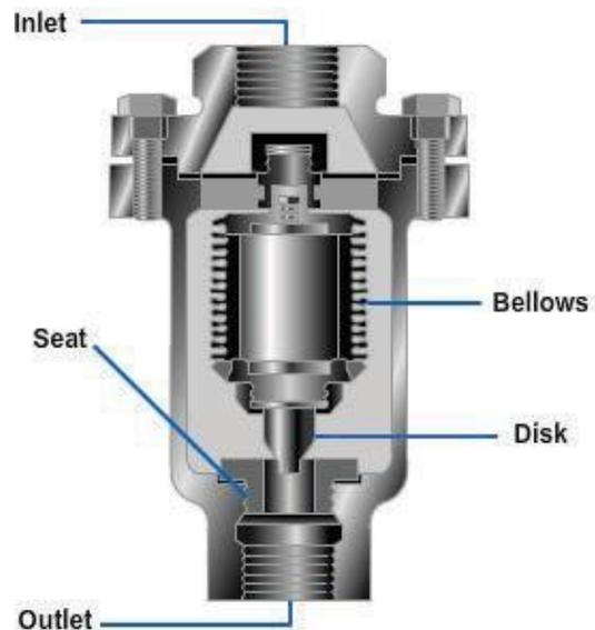
Figure 10-10 – Automatic air vent.
