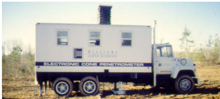
Figure 3-29. Cone penetration testing from cone truck.
