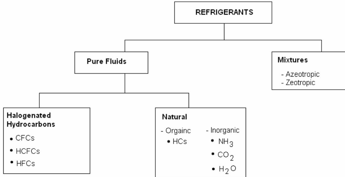
Early refrigerants used in vapor compression refrigeration applications were Halogenated Hydrocarbons predominately made up of chlorofluorocarbons (CFCs), Hydrochloro-fluorocarbons (HCFCs) and Hydrofluorocarbon (HFCs).
