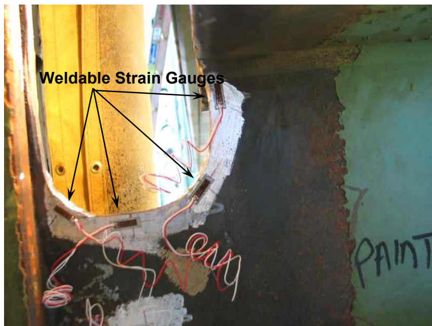
Figure 59. Photo. Weldable strain gauges applied near free edge of retrofit on Girard Point Bridge, Philadelphia, Pennsylvania. Taken from Mahmoud and Connor. (88)
