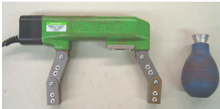
Figure 9. Photo. Mag particle yoke (left). Powder bulb for sprinkling iron powder (right).
