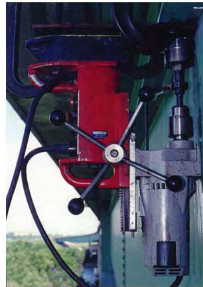
Figure 81. Photo. Completed core of longitudinal stiffener butt weld (left) and picture of magnetic-base drill coring out longitudinal butt weld (right). Photo courtesy of Wiss, Janney, Elstner Associates.
