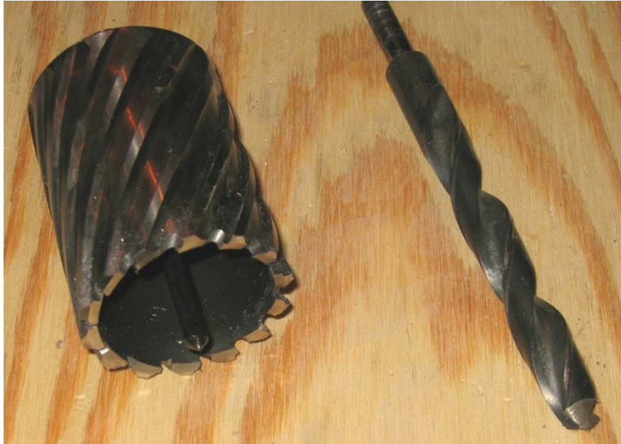
Figure 22. Photo. Annular cutter (left). Twist bit (right).
