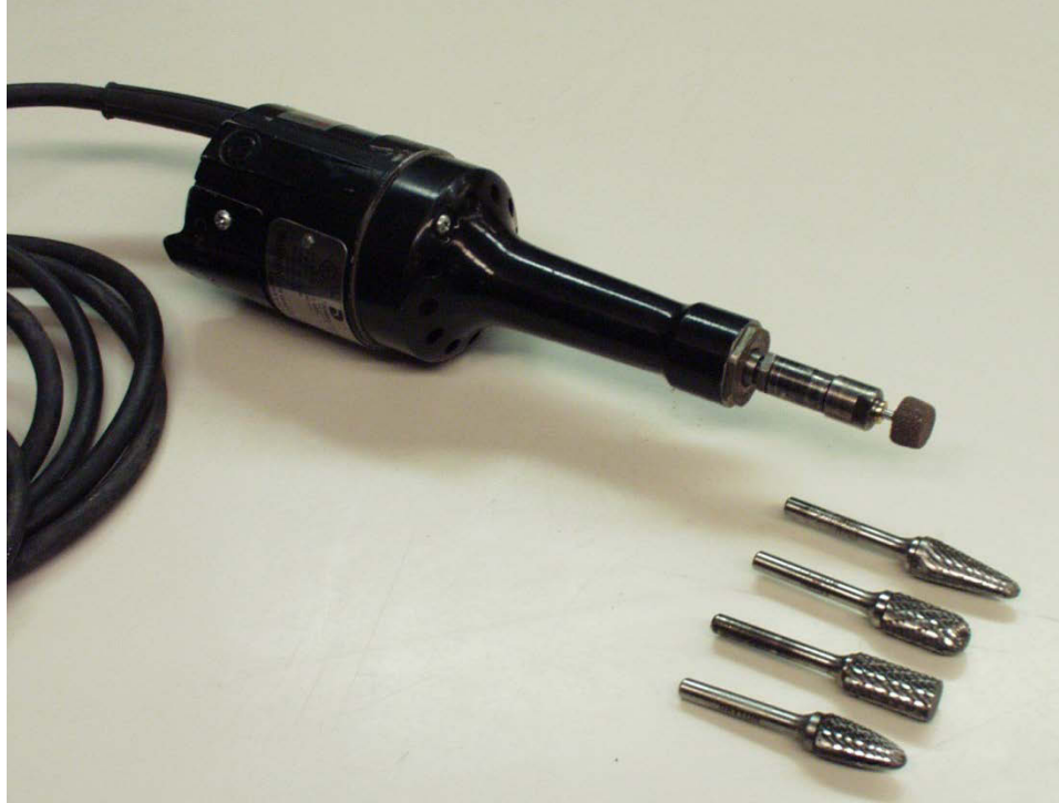
Figure 14. Photo. Typical burr grinder and carbide burr tips.
