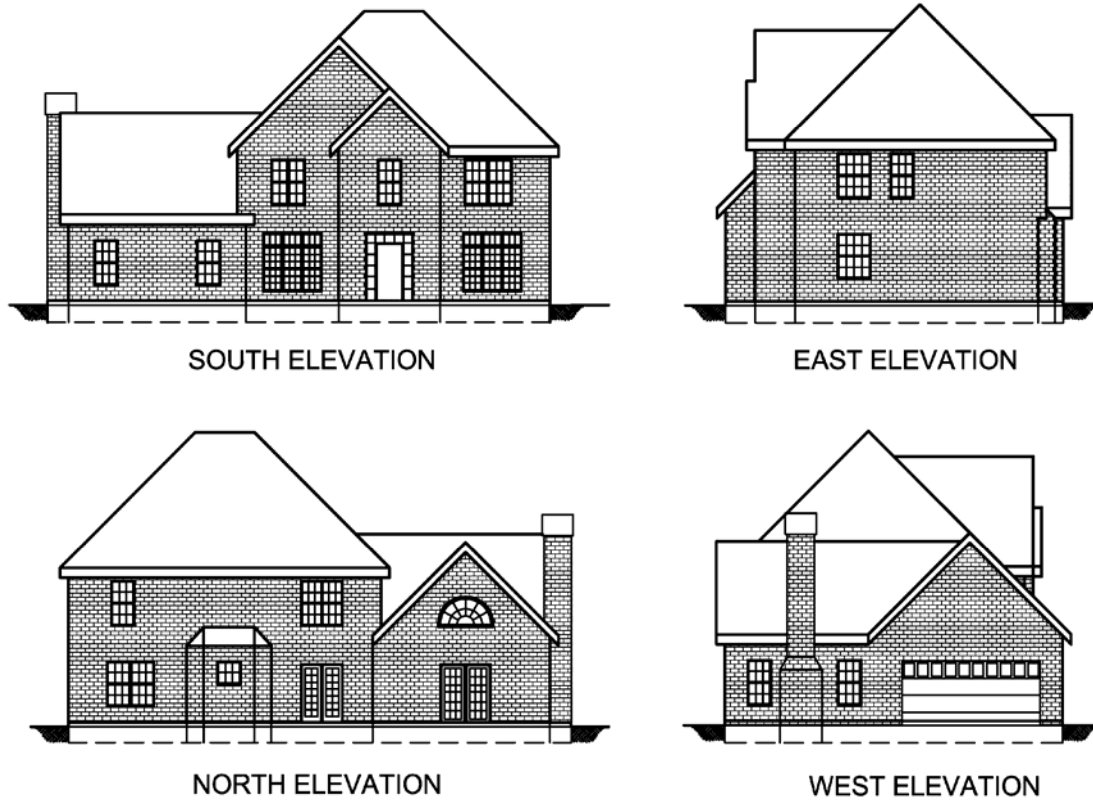
Figure 1-8 Elevations of the model house used as an example for this guide.
