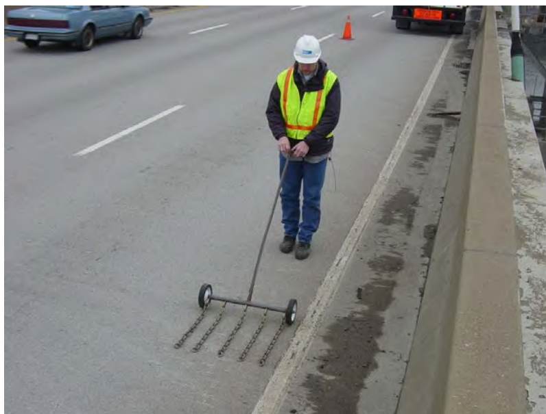
Figure 7.2.7 Sounding for Delaminated Areas of Concrete
