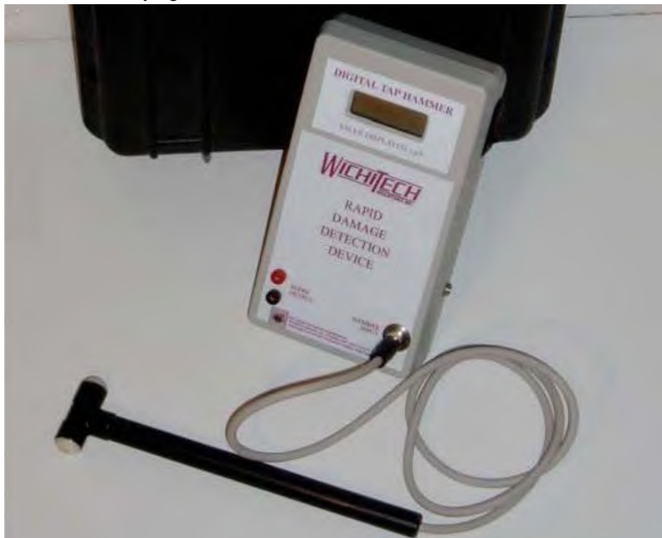
Figure 7.3.6 Electronic Tap Testing Device
