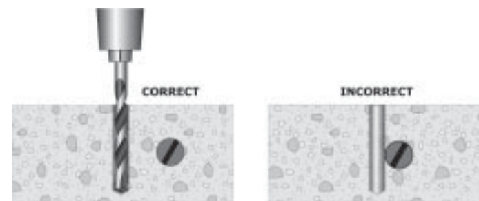
Figure 130: Drilling into concrete with rebar.
