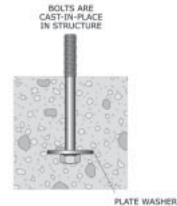
Figure 136: Bolting equipment to cast-in-place anchors.
