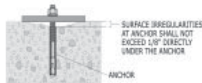
Figure 134: Acceptable gap for grouted plate.
