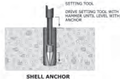
Figure 135: Set shell anchors.
