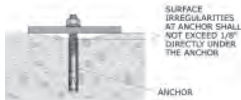
Figure 137: Acceptable gap for grouted plate.
