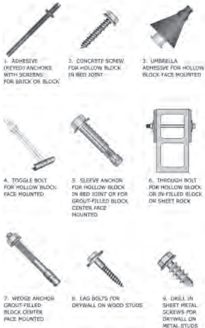
Figure 141: Types of masonry and drywall anchors.
