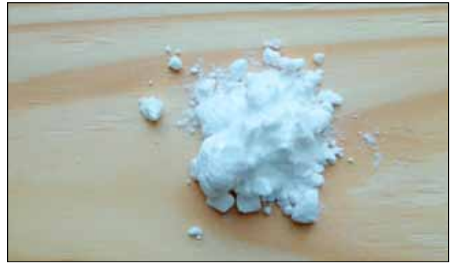
Figure 24. Powdered disodium octaborate tetrahydrate (DOT).
