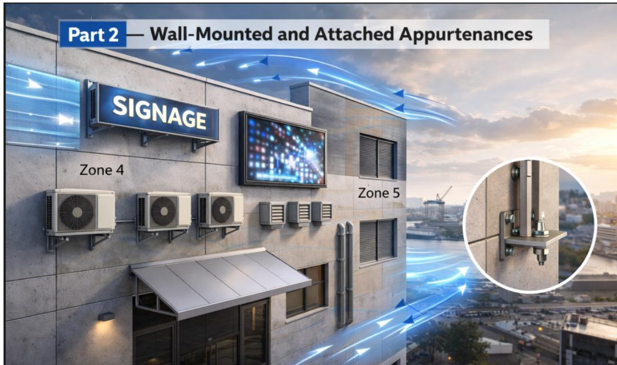
Fig. 2 — Wall-Mounted and Attached Appurtenances Subjected to Components & Cladding Wind Pressures (ASCE 7-22)
