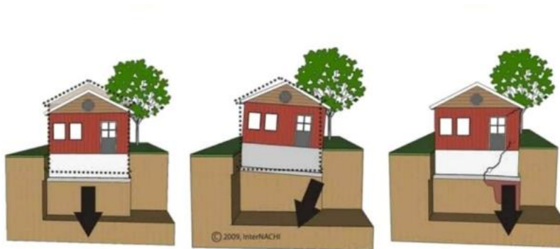
Figure 11. Unequal settlement of masonry
