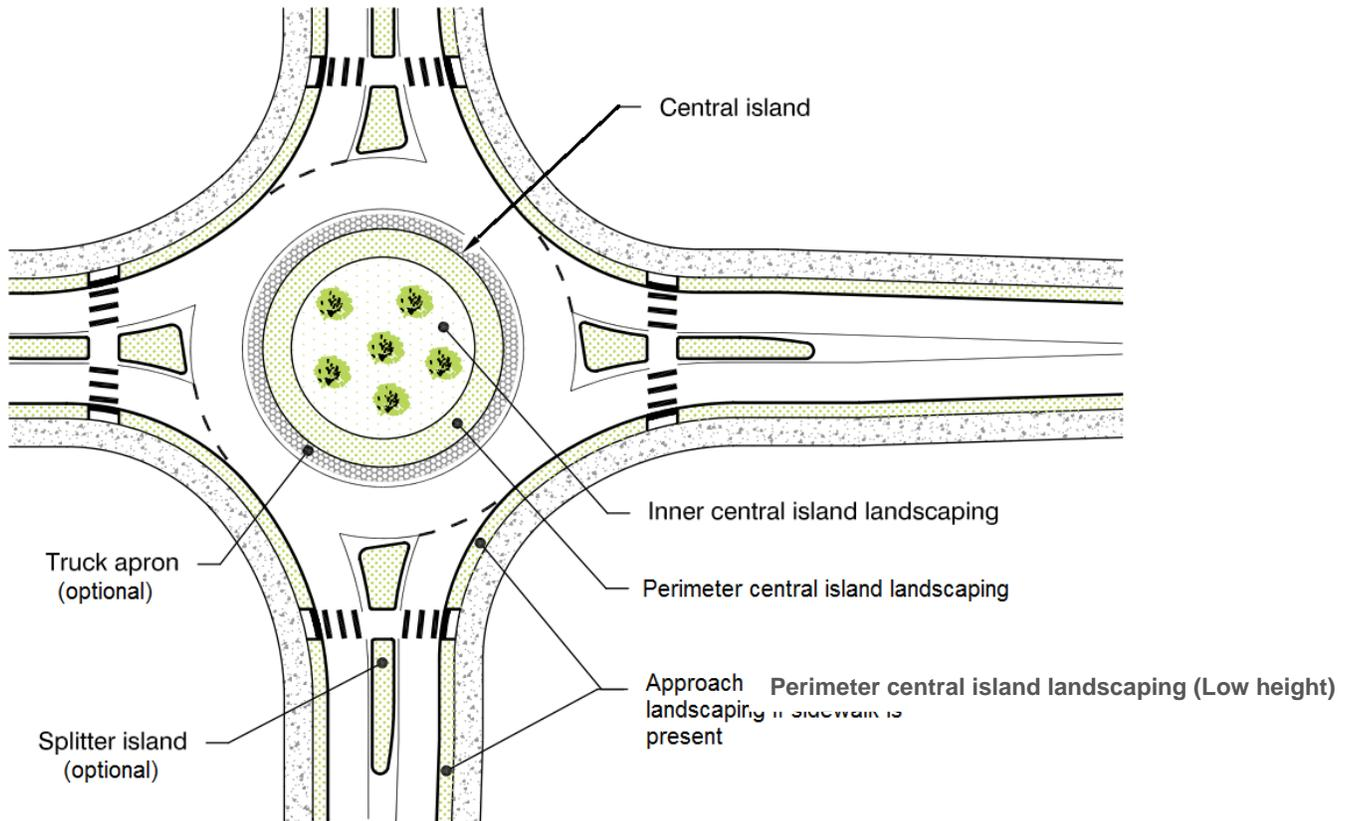
Figure 6.1 – Typical Landscaping Zones within Roundabout (Source: NCHRP 672<sup>1</sup>)
