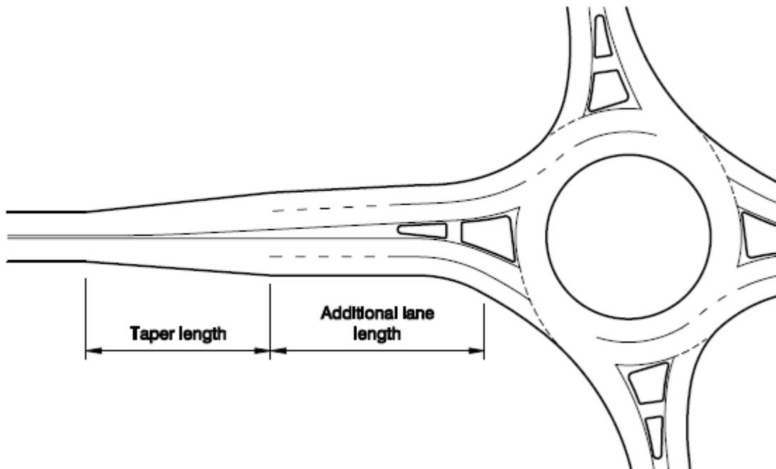
Figure 3.18 – Mid-block Widening by of Approach Lane (Source: NCHRP 672<sup>2</sup>)
