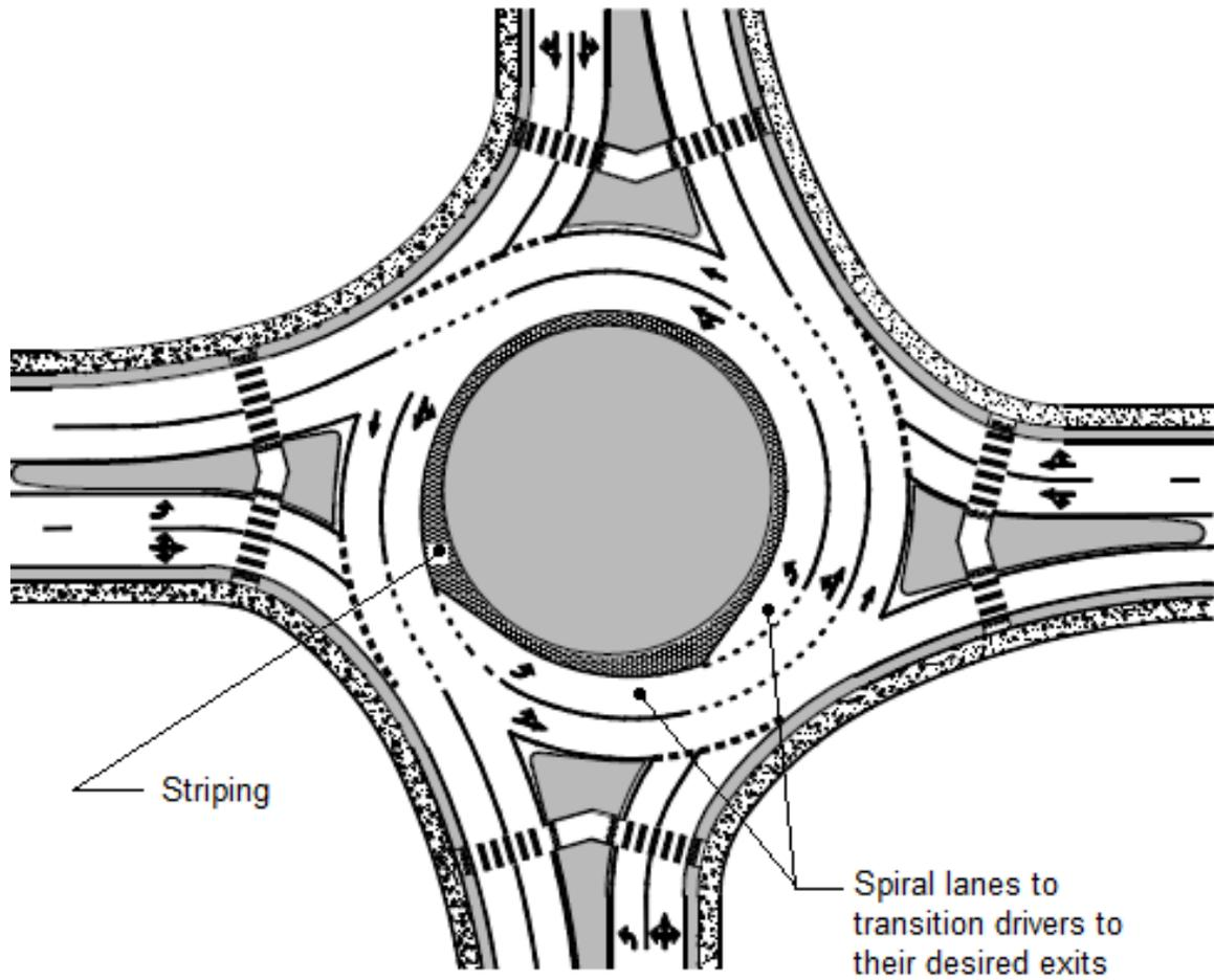
Figure 3.43 – Two-lane Roundabout with Spiral lanes to transition Left-Turn Traffic (Source: NCHRP 672<sup>2</sup>)
