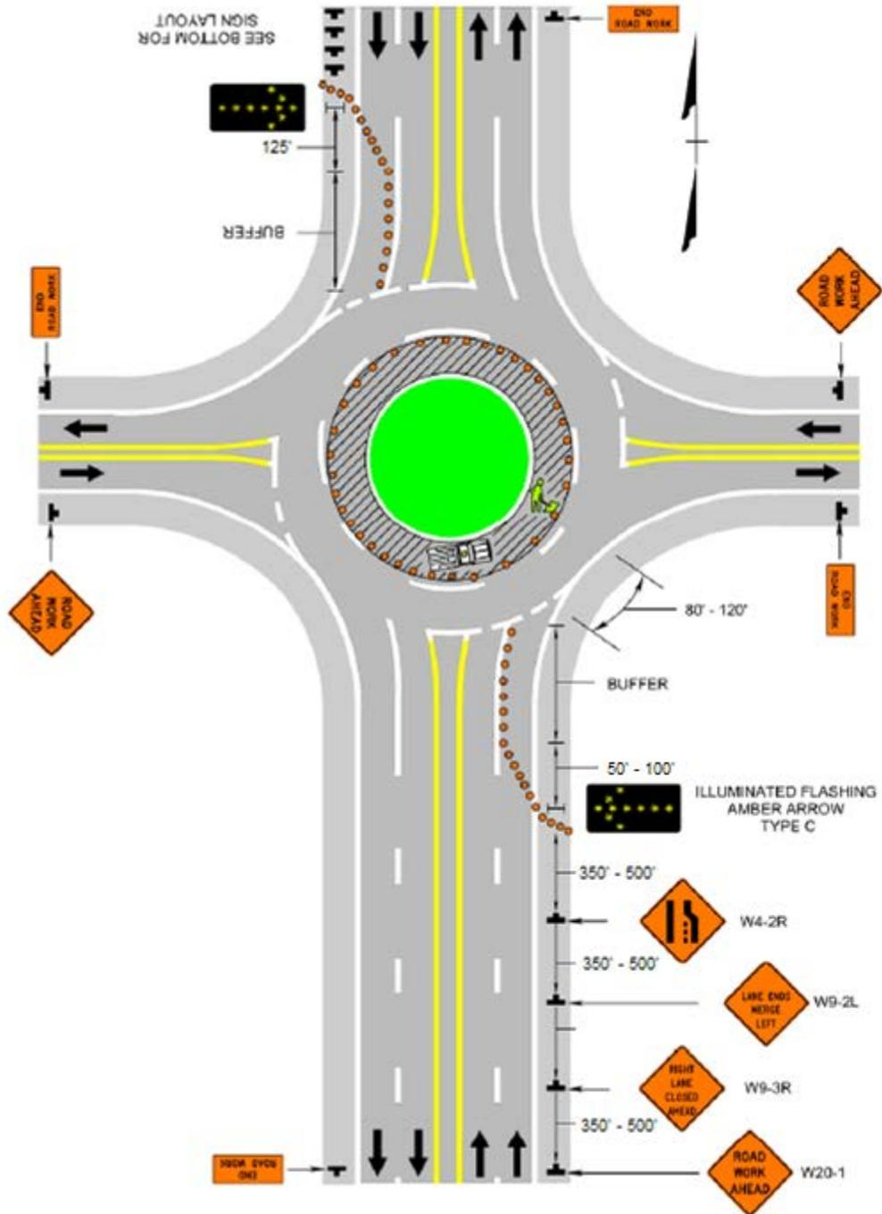
Figure 8.4 – Typical Multi-Lane Roundabout Inside Lane Closure Operation (Source: VDOT<sup>3</sup>)
