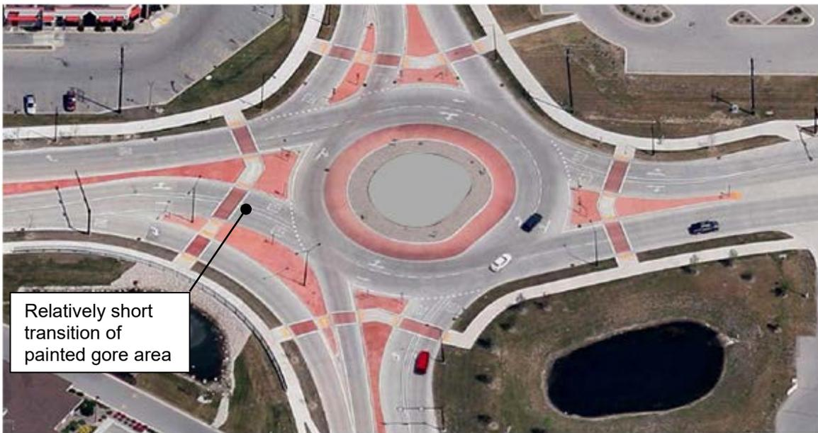
Figure 3.23 – Case 2 Roundabout (Source: RTE<sup>11</sup>)
