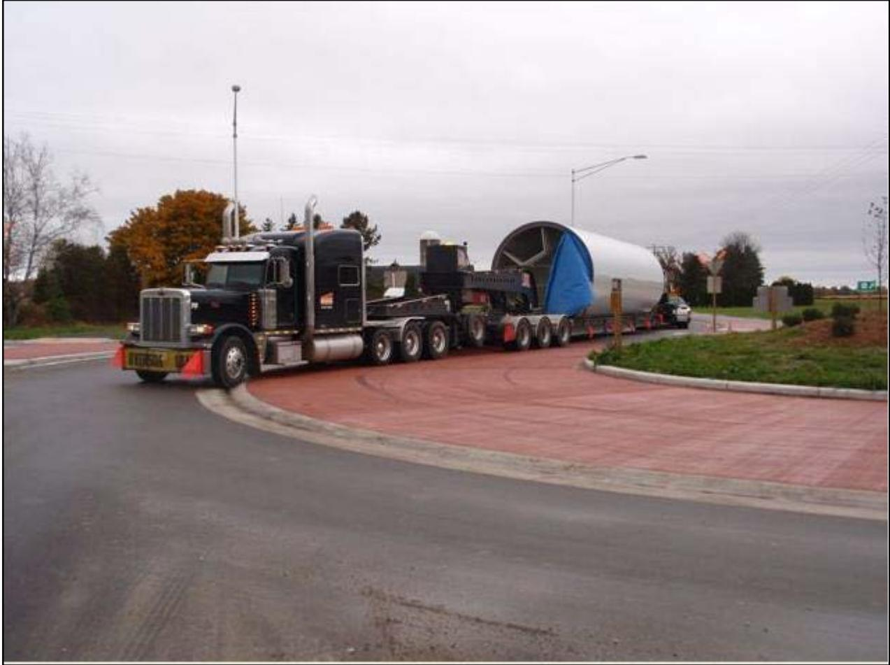
**Figure 3.32 – Wide Truck Apron for OSOW Accommodation (Source: RTE<sup>11</sup>)**
