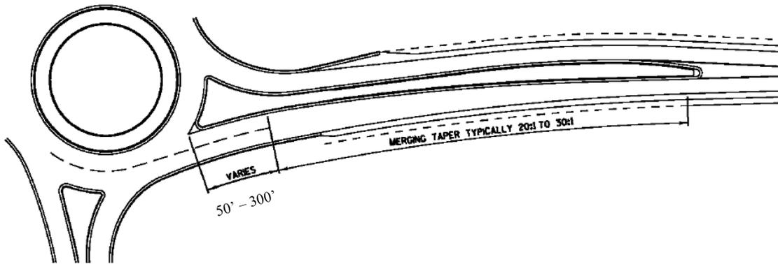
**Figure 3.9 – Exit Lane and Taper (Source: WisDOT<sup>4</sup>)**
