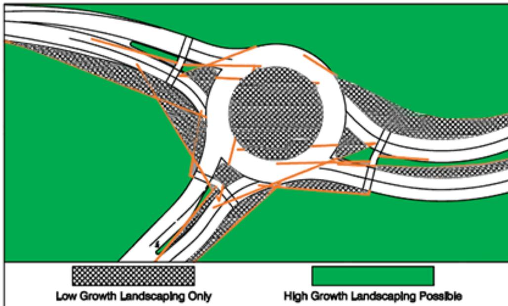
Figure 3.52 – Example Sight Distance Diagram (Source: NCHRP 672<sup>2</sup>)
