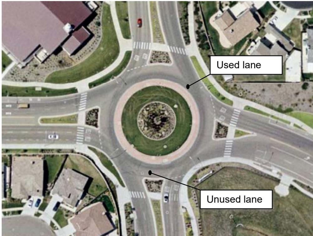
Figure 3.37 – Entry Path Overlap Example (Source: NYSDOT<sup>14</sup>)
