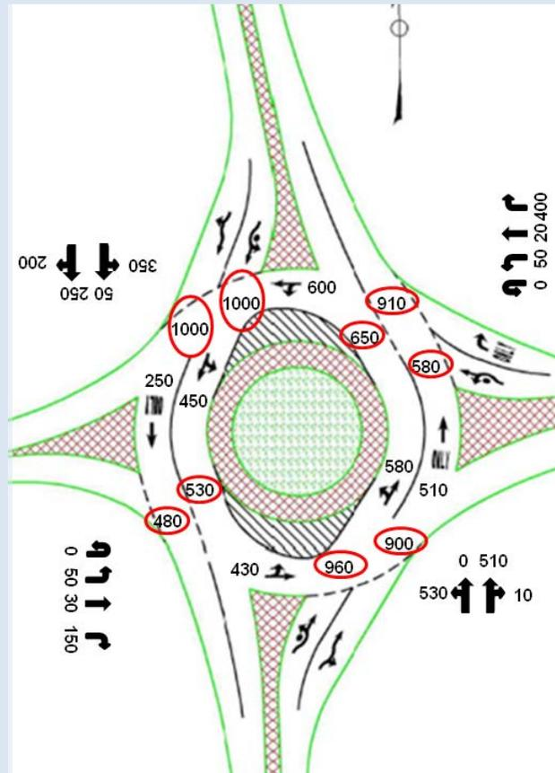
Figure 2.3 (cont.) – Example Calculation on Entry Lanes Determination
