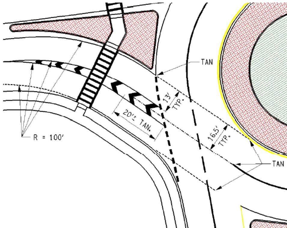
Figure 3.39 – Left Offset Design and Truck Gore Striping (Source: NYSDOT<sup>14</sup>)
