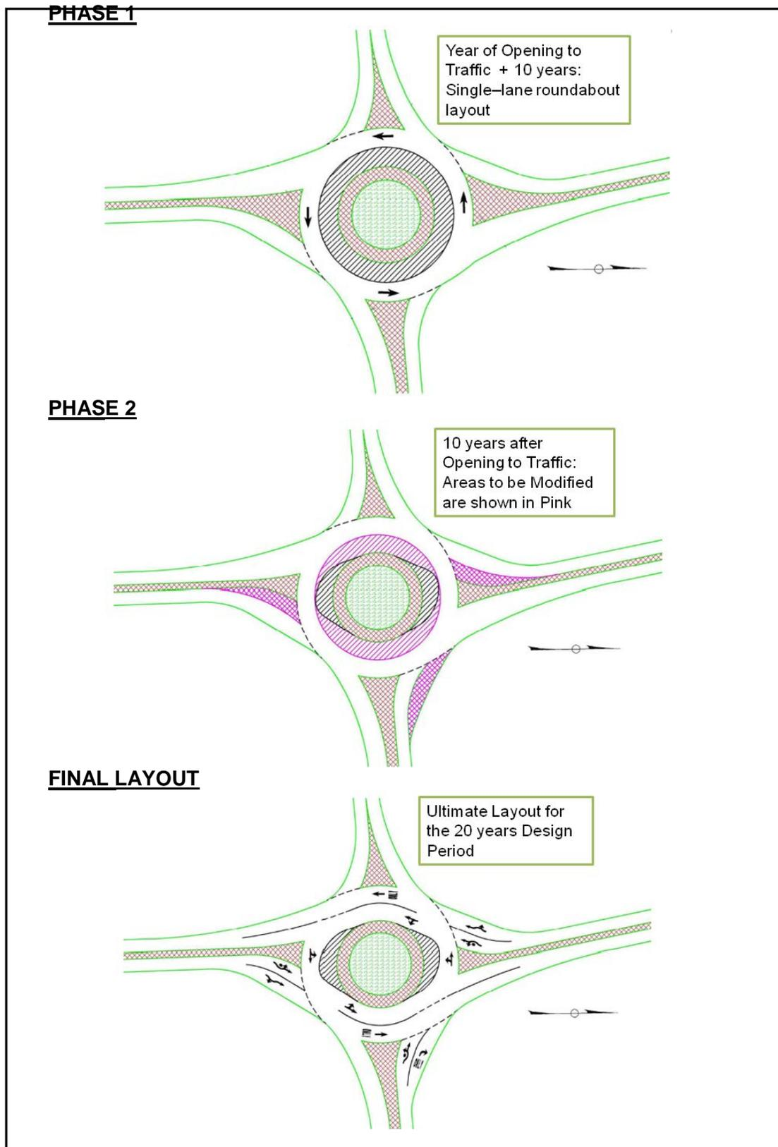
Figure 2.9 Staged Multilane Roundabout (courtesy: Howard McCulloch, NYSDOT<sup>2</sup>)
