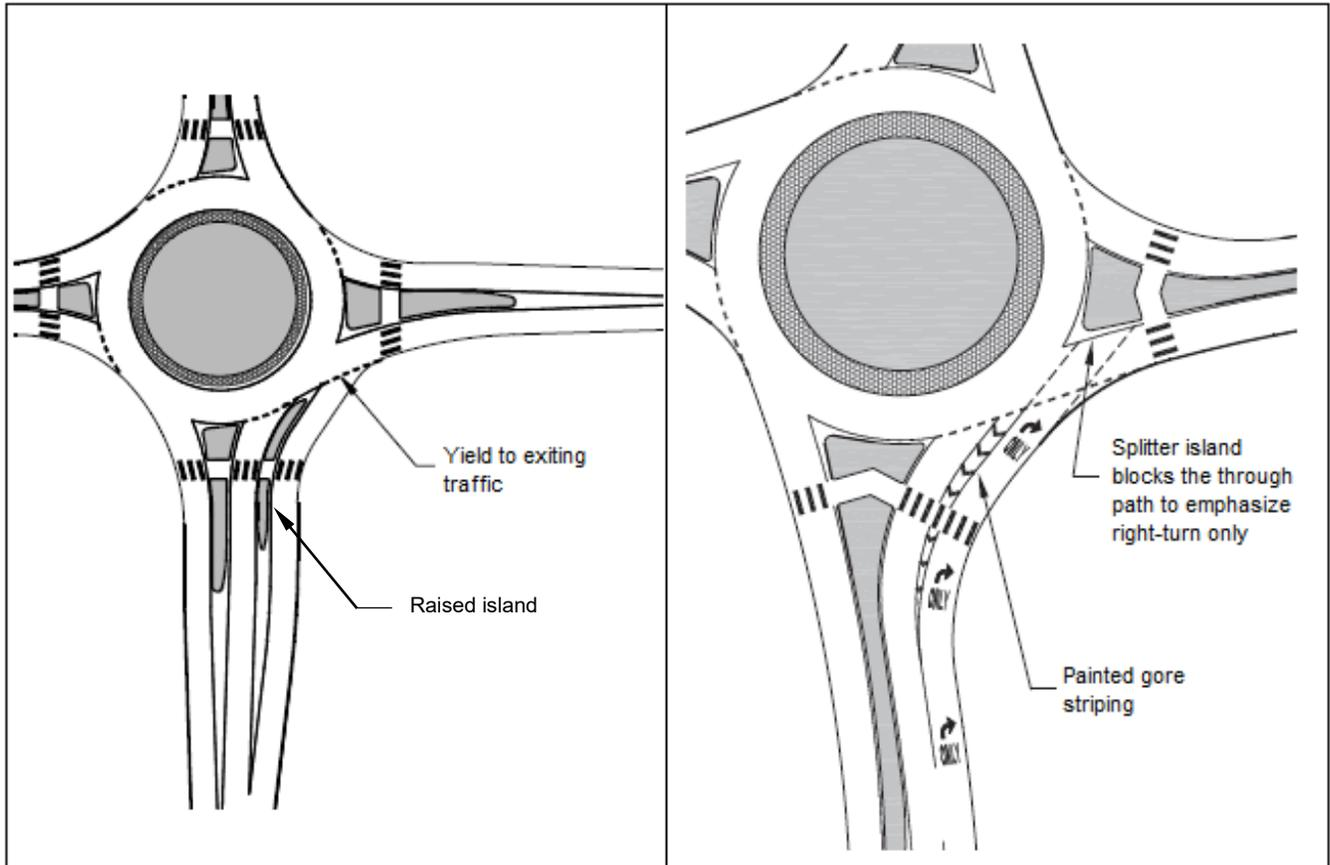
**Figure 3.42 – Right-Turn Bypass Lane with Yield at Exit Leg (Source: NCHRP 672<sup>2</sup>)**
