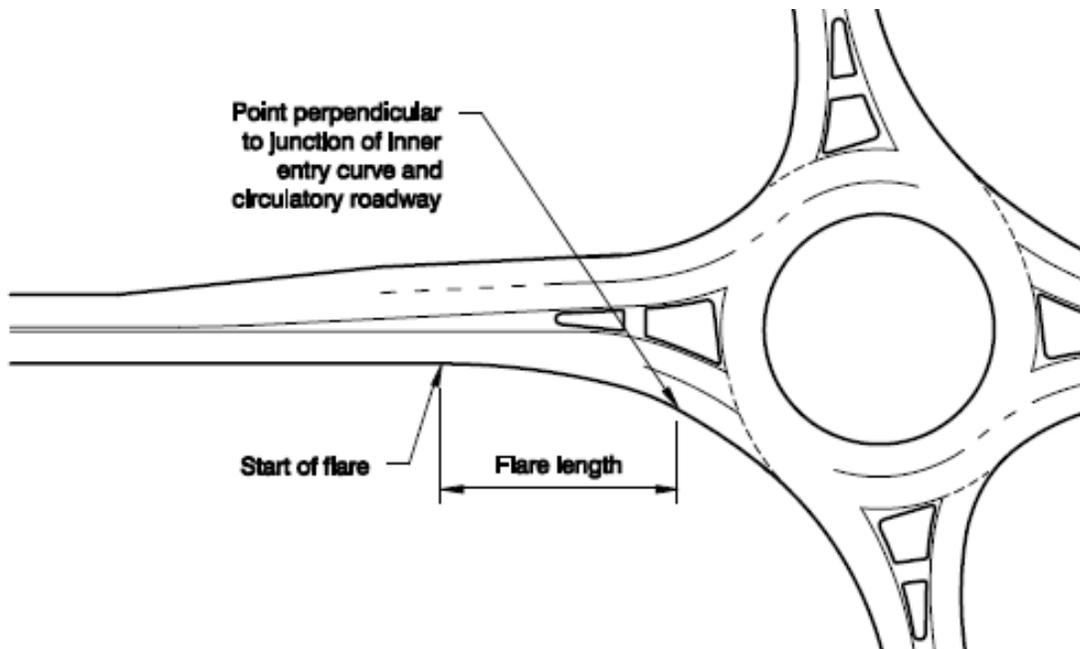
Figure 3.19 – Approach Widening by Entry Flaring (Source: NCHRP 672<sup>2</sup>)
