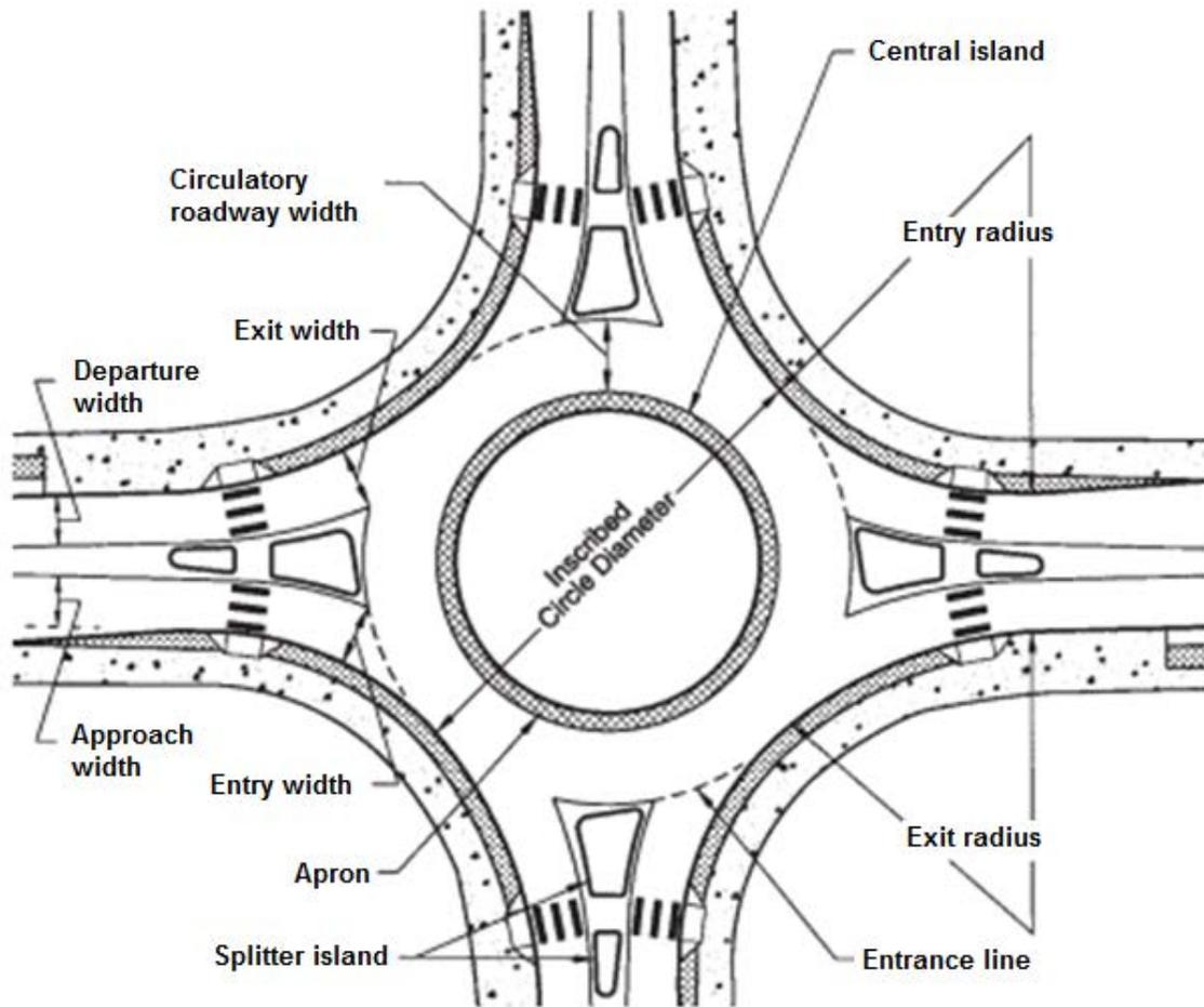
Figure 3.1 – Roundabout Geometric Design Elements (Source: FHWA<sup>1</sup>)
