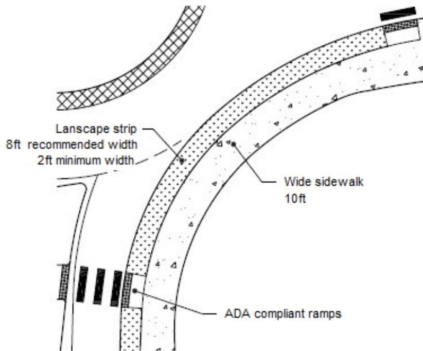
**Figure 3.53 – Typical Sidewalk Treatment (Source: NCHRP 672<sup>2</sup>)**
