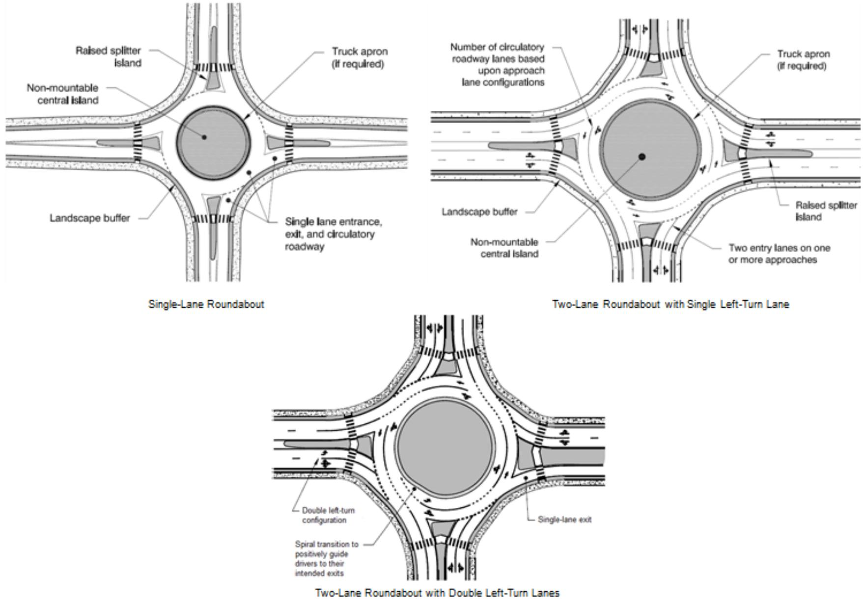
Figure 1.5 – Single-lane and Multilane Roundabout Categories (NCHRP 672<sup>1</sup>)
