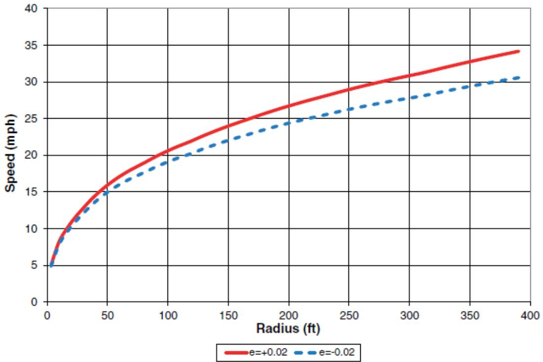
Figure 3.48– Speed-Radius Relationship (Source: NCHRP 672<sup>2</sup>)
