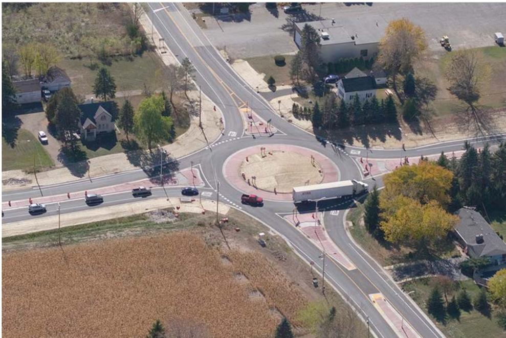
**Figure 3.21 – Example of Single Lane Roundabout, (Source: GHD<sup>10</sup>, Jackson WI)**
