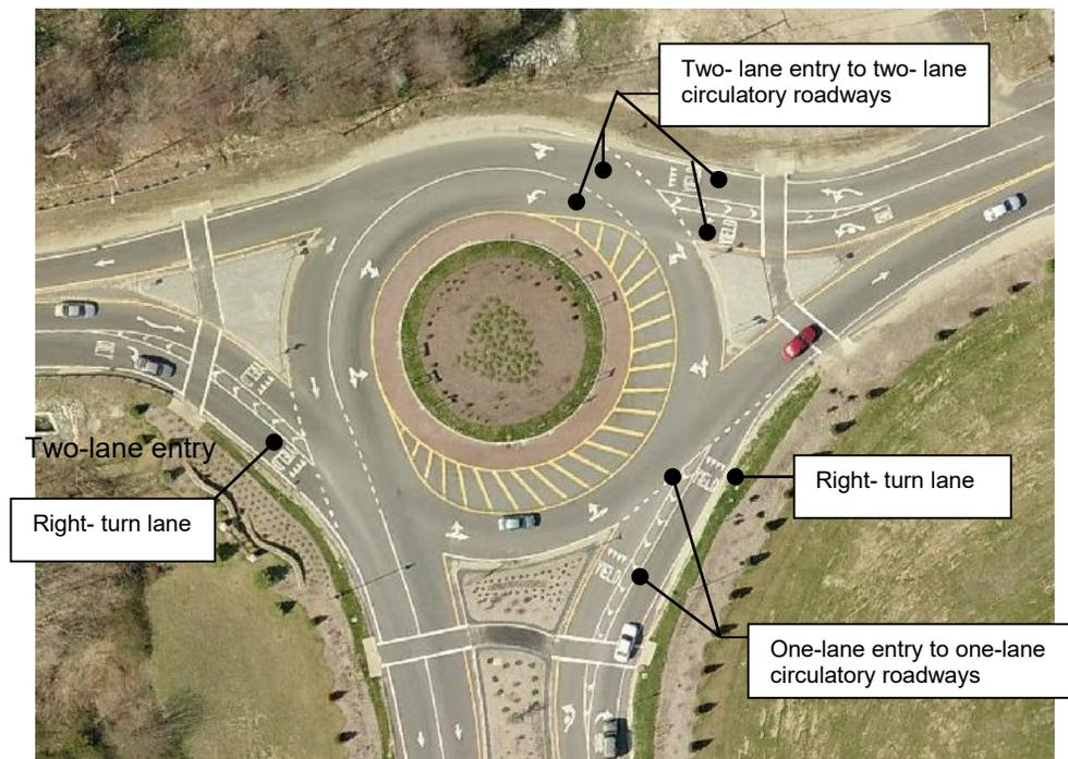
**Figure 3.8– Example of Multilane with Circulatory Roadway Lanes Matching Entry Lanes** (Source: FHWA<sup>1</sup>)
