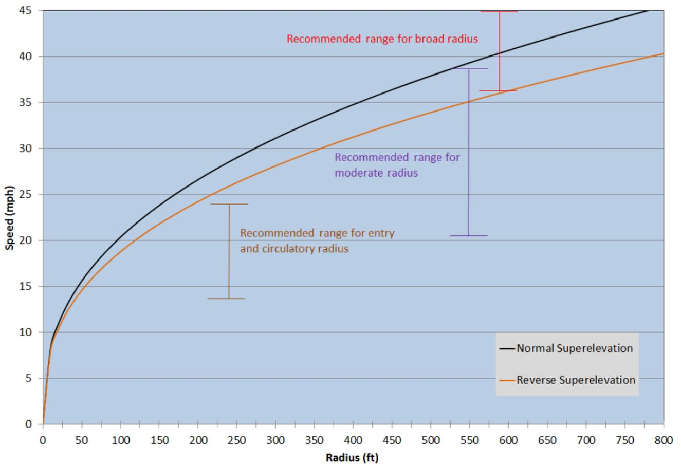
Figure 3.6 – Relationship Between Approach Speeds and Chicane Curves (Source: WSDOT<sup>5</sup>)
