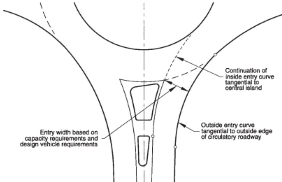
Figure 3.14– Single-Lane Roundabout Entry Design (Source: NCHRP 672<sup>2</sup>)
