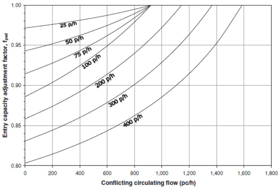
Figure 2.8 – Entry Capacity Adjustment Factor for Pedestrians (Source: HCM 2010<sup>3</sup>)
