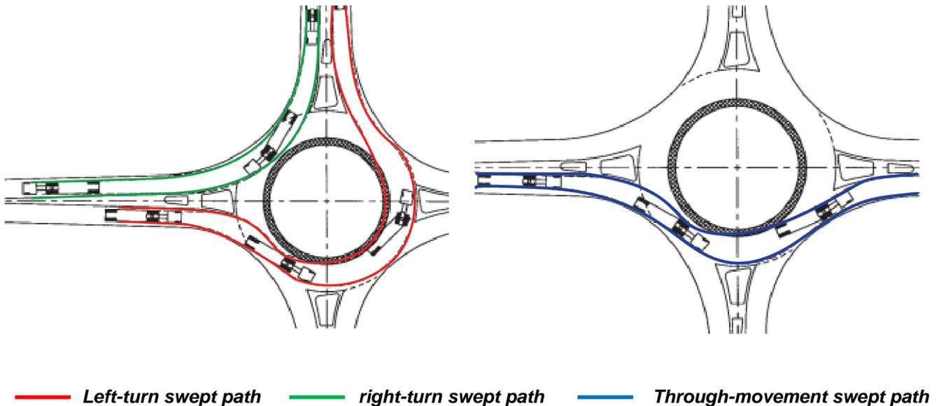
**Figure 3.3– Illustration of Vehicle Swept Path Check (Source: FHWA<sup>1</sup>)**
