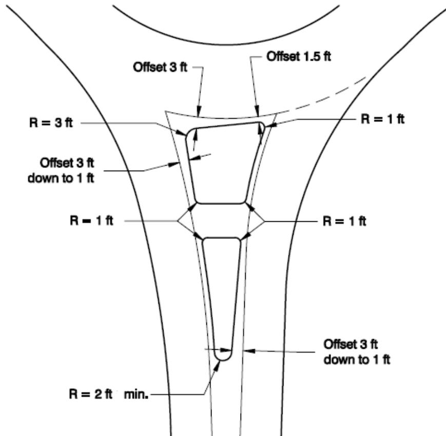
Figure 3.11 – Typical Minimum Splitter Island Nose Radii and Offset Dimensions (Source: NCHRP 672<sup>2</sup>)
