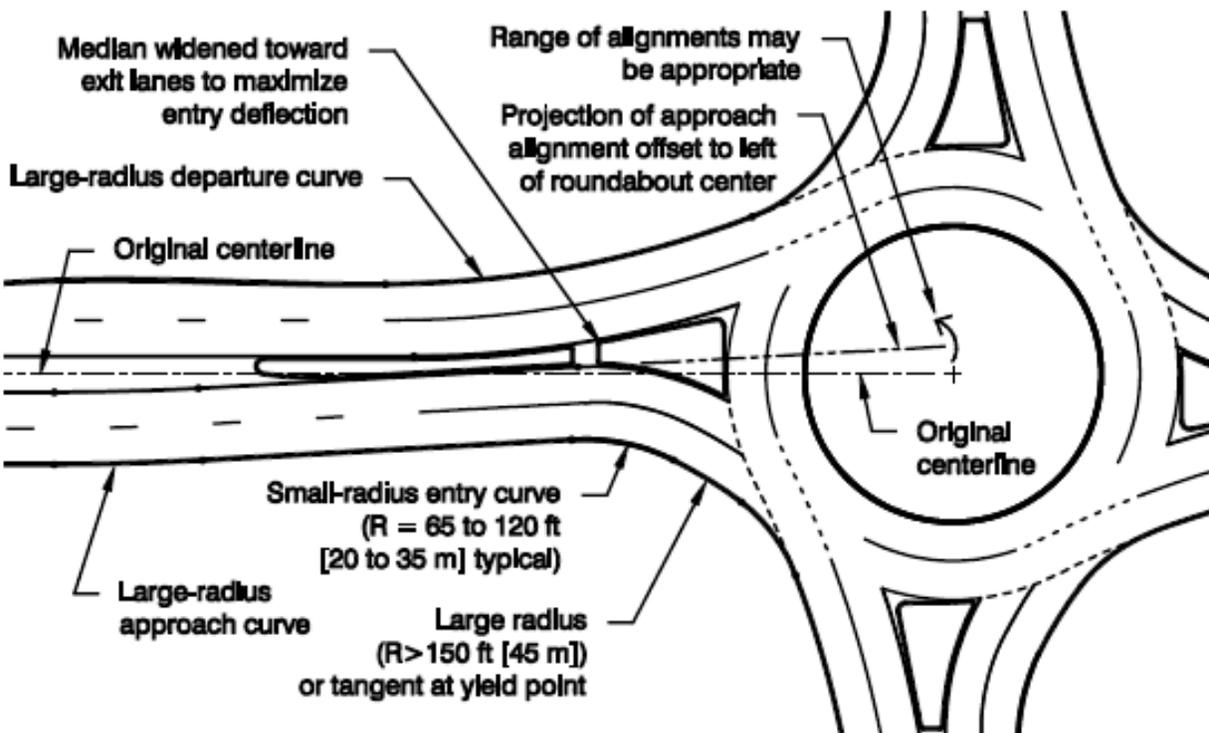
Figure 3.38– Illustration of Left Offset Entry design (Source: NCHRP 672<sup>2</sup>)
