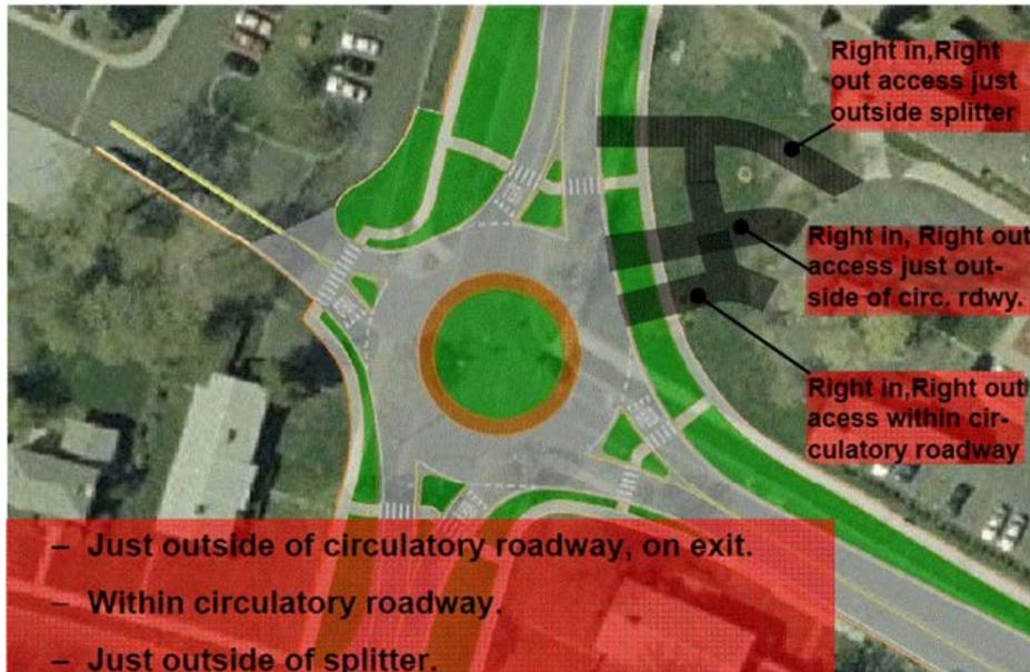
Figure 3.59– Residential Driveways with Right-In/Right-Out Access Control (Source: NYSDOT<sup>14</sup>)
