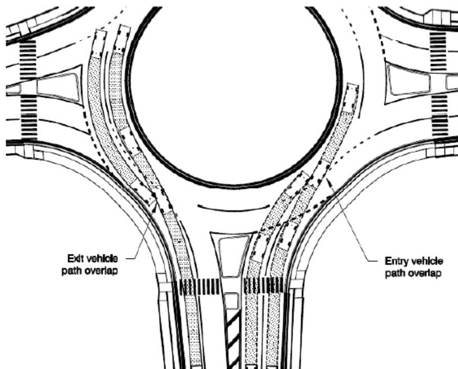
Figure 3.36 – Illustration of Entry Path Overlap (Source: NCHRP 672<sup>2</sup>)
