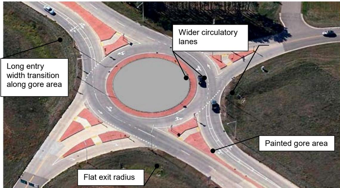
Figure 3.24 – Case 3 Roundabout (Source: RTE<sup>11</sup>)
