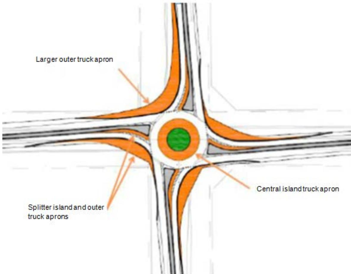
**Figure 3.31 – Design Locations of Truck Apron for OSOW Movement (Source: RTE<sup>11</sup>)**
