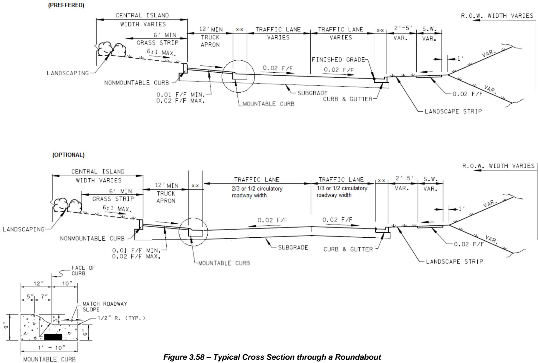
Figure 3.58 – Typical Cross Section through a Roundabout
