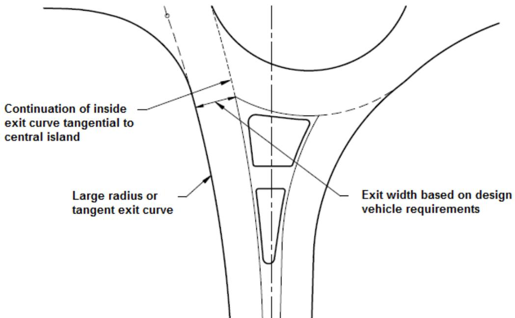
**Figure 3.20 – Single-Lane Roundabout Exit Design (Source: NCHRP 672<sup>2</sup>)**
