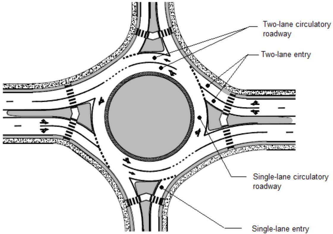
**Figure 3.7 – Multilane Roundabout Partially Reduced to One Lane on Circulatory Roadway**
