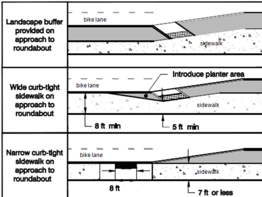
Figure 3.56– Bicycle Ramp Design Options (Source: NCHRP 672<sup>2</sup>)
