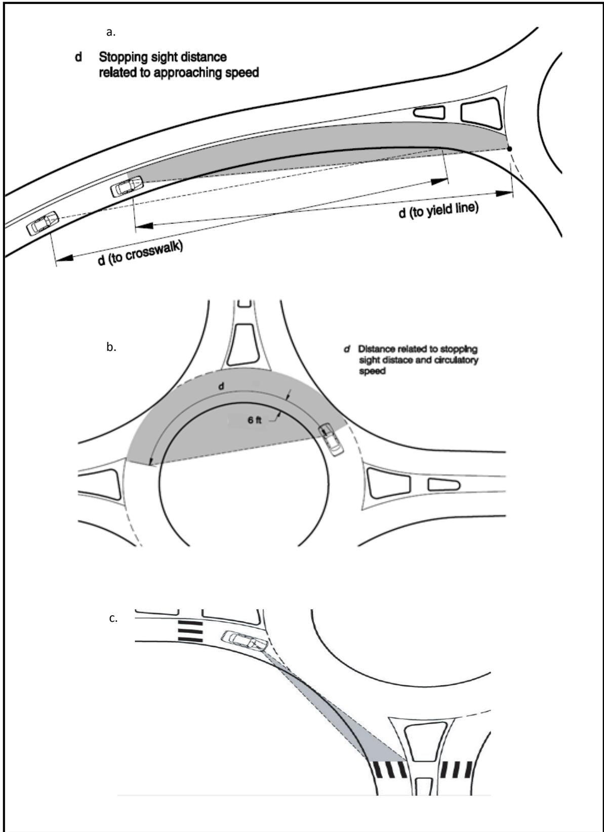
Figure 3.50– Critical Stopping Sight Distance Locations (Source: NCHRP 672<sup>2</sup>)
