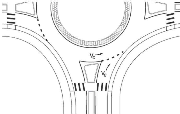
**Figure 2.4 – Typical One-Lane Entry Conflicted by One Circulating Lane (Source: HCM 2010<sup>3</sup>)**
