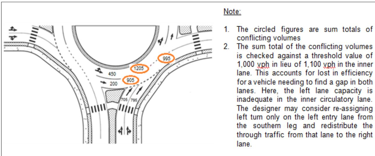
**Figure 2.2 – Lane-by-Lane Checks for Capacity Limits on Two Lane Roundabout Approaches**
