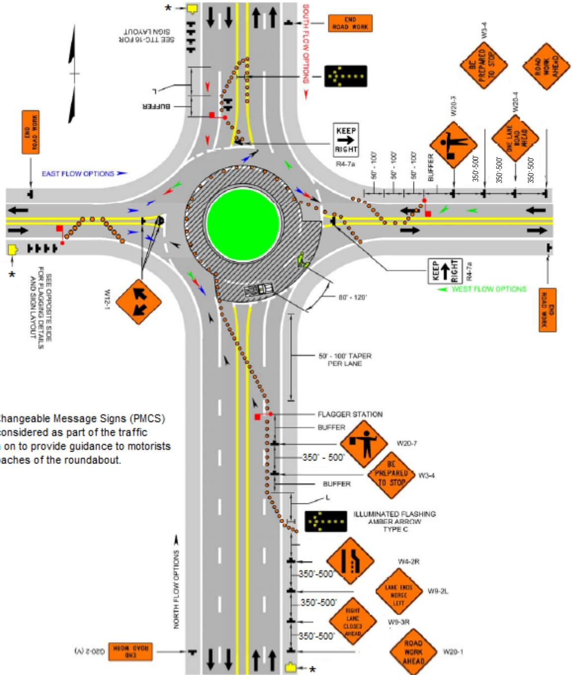
Figure 8.5 – Typical Multi-Lane Roundabout Outside Lane Closure Operation (Source: VDOT<sup>3</sup>)
