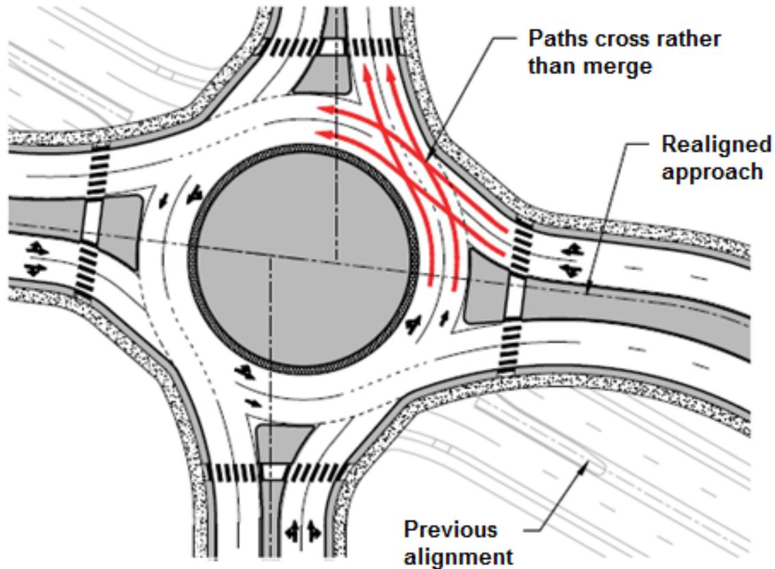
Figure 3.17 – Realignment to Resolve Exit–Circulating Conflicts (Source: NCHRP 672<sup>2</sup>)
