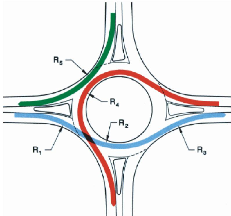
Figure 3.46– Vehicle Path Radii (Source: NCHRP 672<sup>2</sup>)
