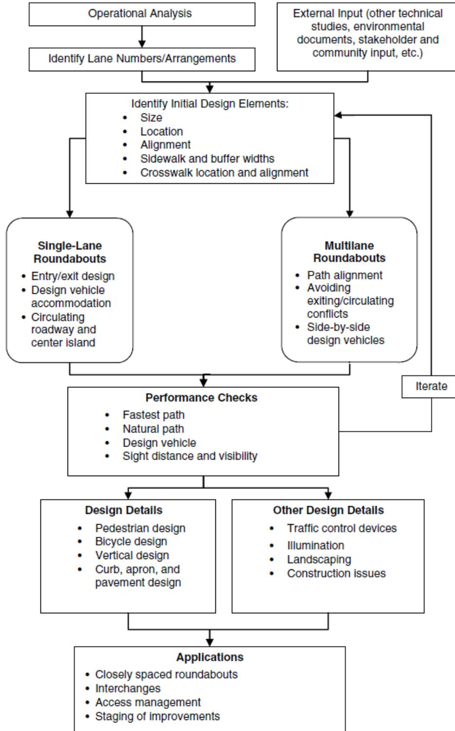
Figure 3.2 – Basic Procedure for the Design of Roundabout Intersection (Source: NCHRP 672<sup>2</sup>)
