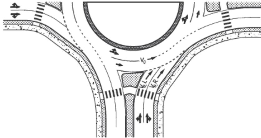
**Figure 2.5 –Typical Two-Lane Entry Conflicted by Two Circulating Lanes (Source: HCM 2010<sup>3</sup>)**
