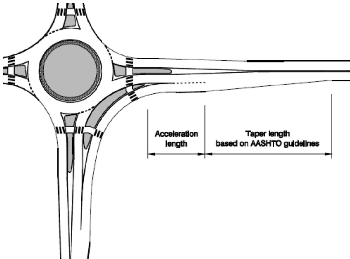
**Figure 3.41 – Right-Turn Bypass Lane with Acceleration Lane and Taper (Source: NCHRP 672<sup>2</sup>)**
