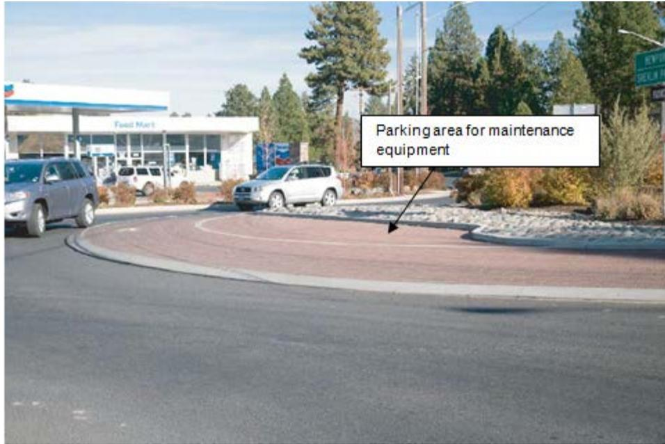
**Figure 8.1 – Parking Area Provision for the Docking of Maintenance Vehicle (Source: NCHRP 672<sup>1</sup>)**
