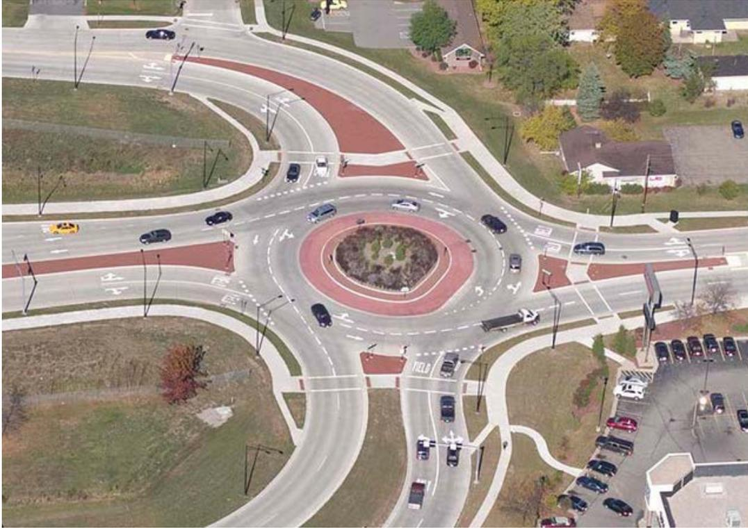
**Figure 3.44 – Example of Two-Lane Roundabout with Spiral Lane to Transition Innermost Left Turn Traffic from Southern Approach Leg to Exit (Source: GHD<sup>10</sup>)**
