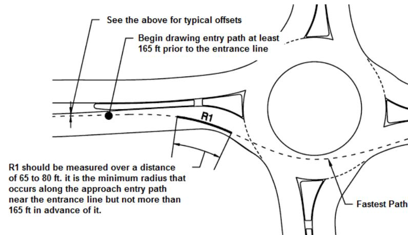
Typical Procedure for Measuring R1 Radius
