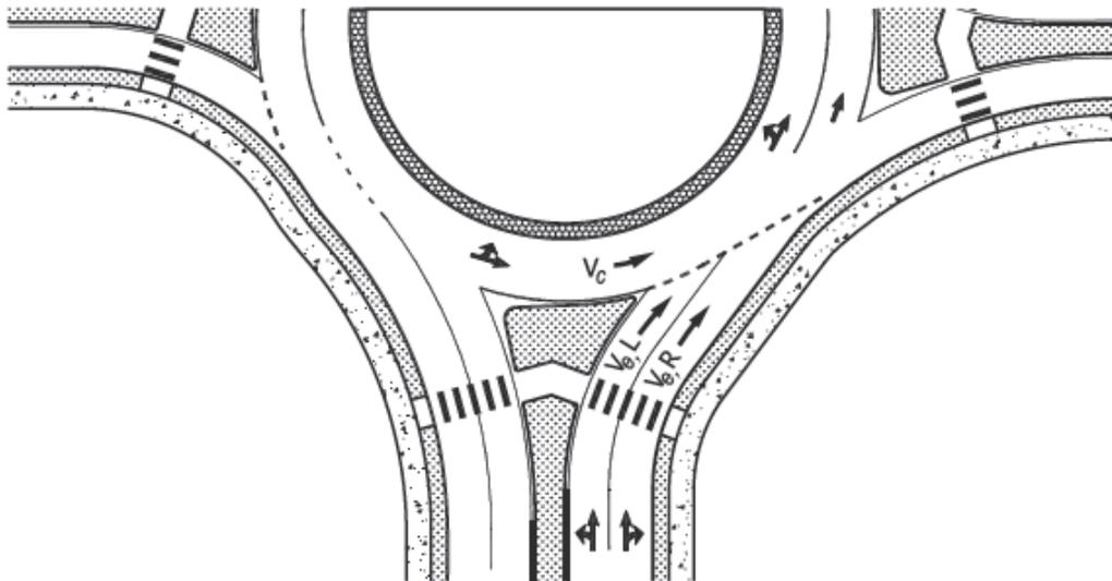
**Figure 2.6 –Typical Two-Lane Entry Conflicted by One Circulating Lane (Source: HCM 2010<sup>3</sup>)**
