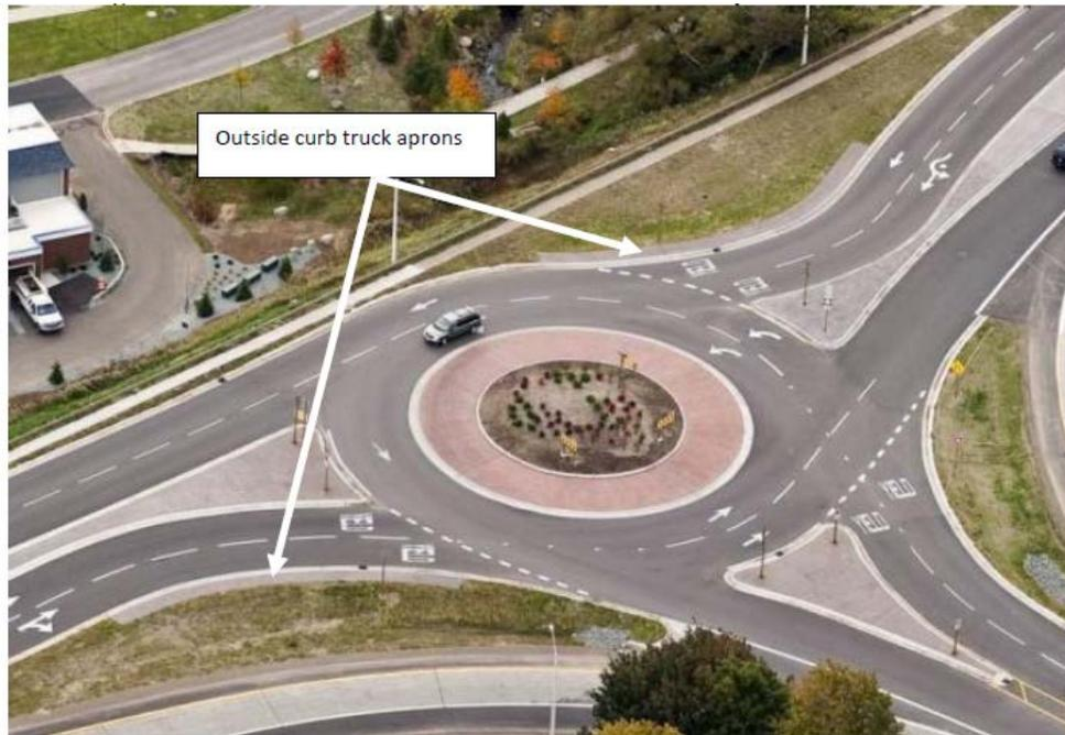
**Figure 3.25 – Case 1 Roundabout with Outside Curb Truck Aprons (Source: MDOT<sup>13</sup>)**
