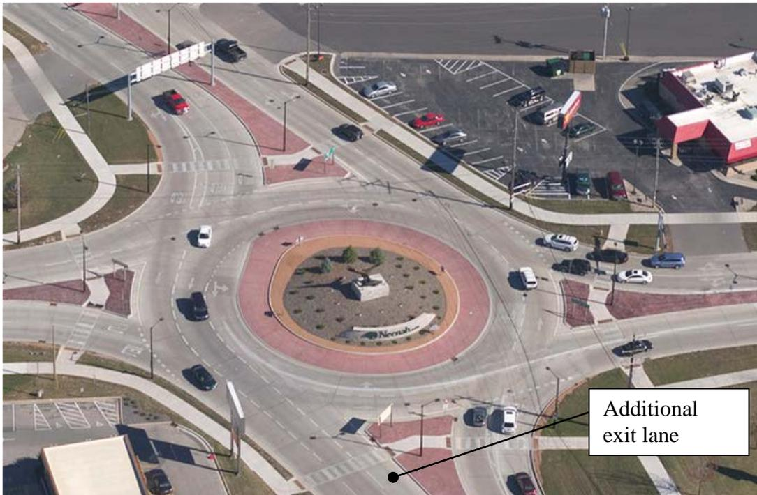
**Figure 3.45 – Example of Two-Lane Roundabout with Spiral Lane and Additional Exit Lane to Transition the Innermost Through/Left Turn to Exit (Source: GHD<sup>10</sup>)**
