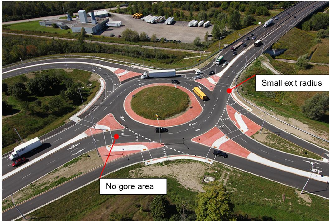
Figure 3.22 – Case 1 Roundabout (Source: GHD<sup>10</sup>, Cambridge ON)
