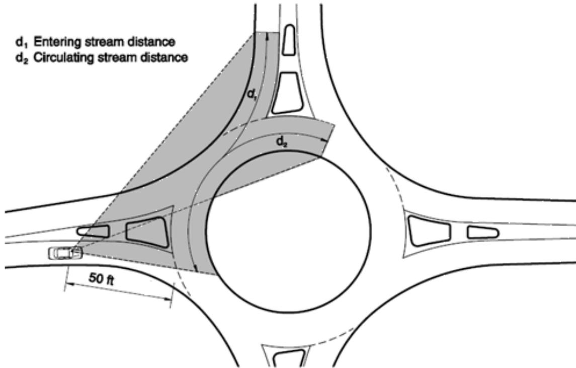
Figure 3.51 – Critical Intersection Sight Triangles (Source: NCHRP 672<sup>2</sup>)
