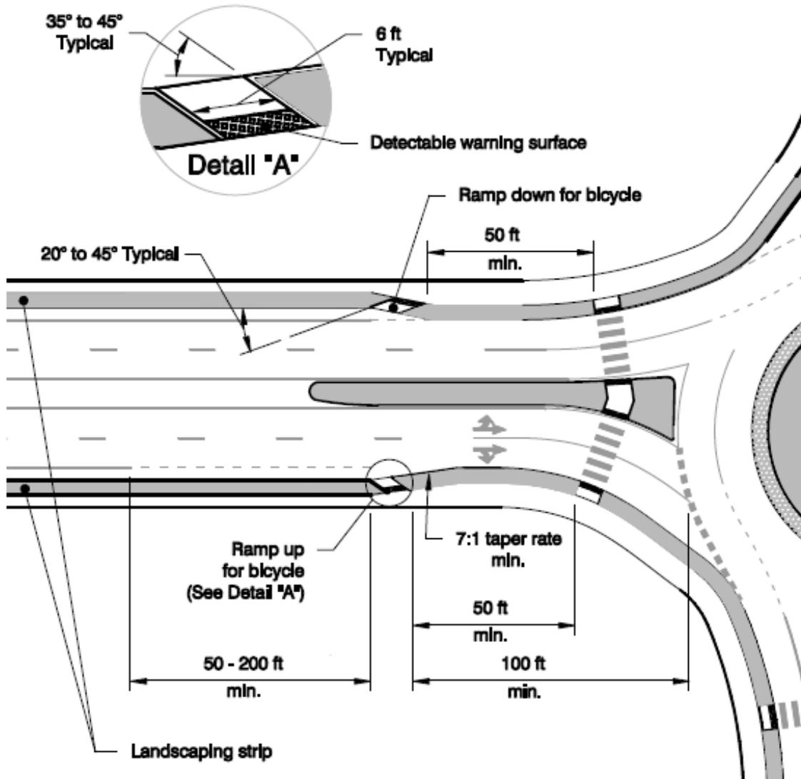
Figure 3.54 – Typical Pedestrian and Cyclist Treatment (Source: NCHRP 672<sup>2</sup>)
