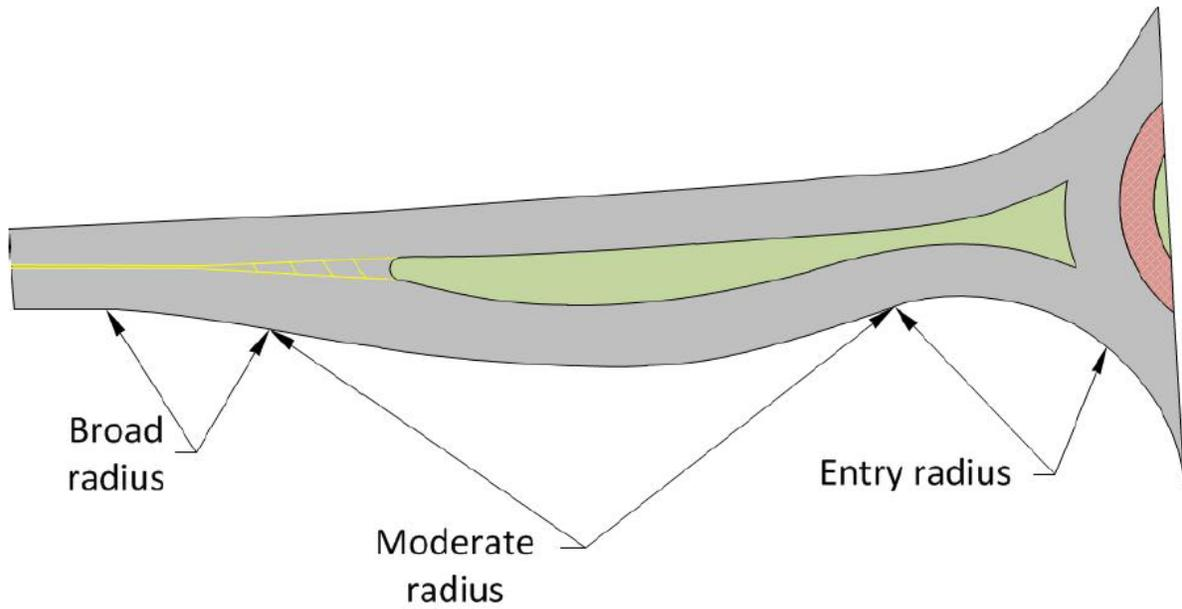
Figure 3.5 – Chicane Schematic (Source: WSDOT<sup>5</sup>)
