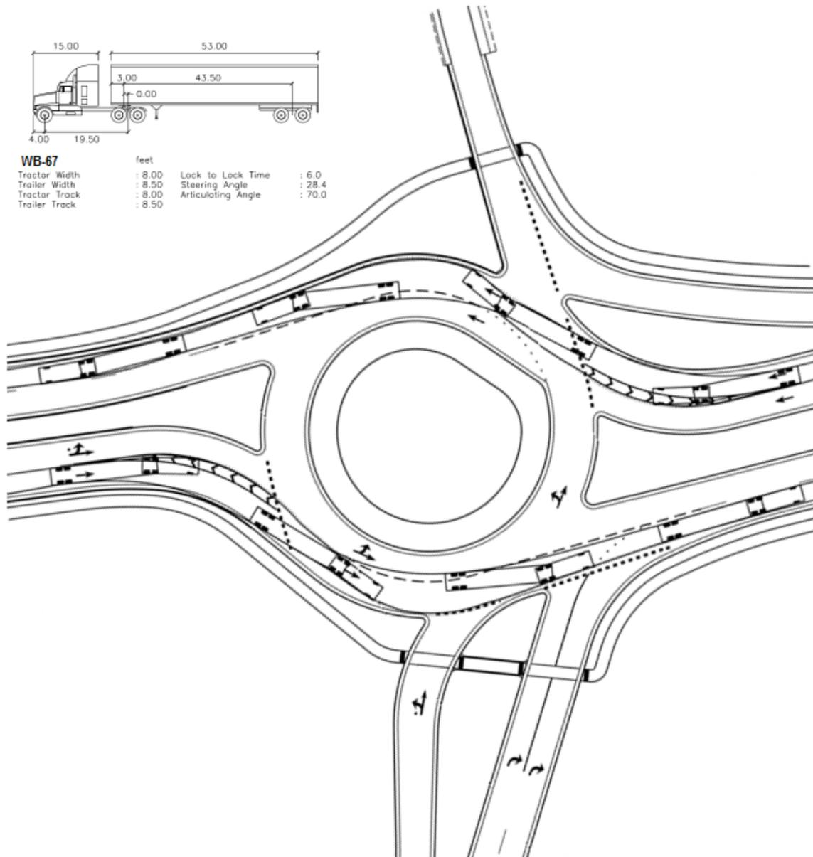
**Figure 3.27 – Case 2 Roundabout Design Characteristics (Source: WisDOT<sup>4</sup>)**
