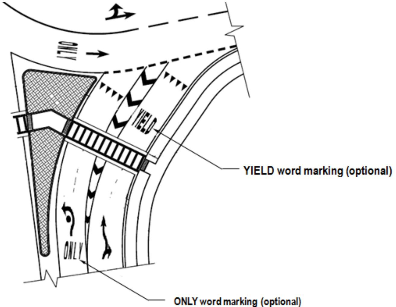
**Figure 4.6 – Pavement Words and Symbols (Source: NCHRP 672<sup>4</sup>)**
