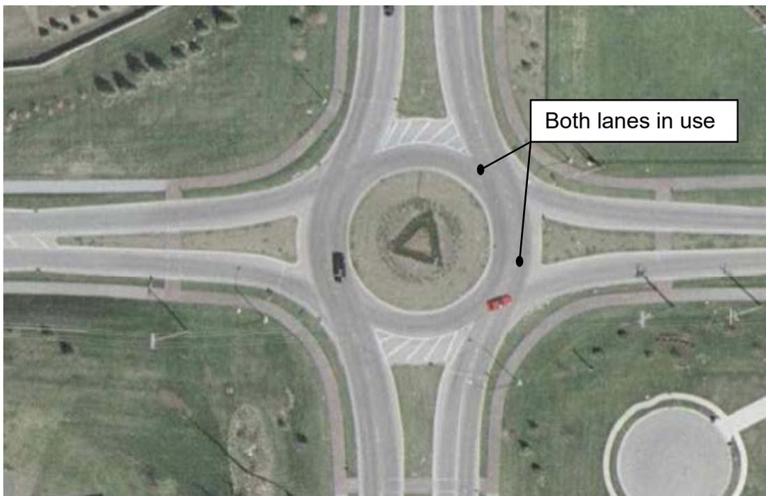
Figure 3.40 – Lane Striping to Eliminate Path Overlap (Source: NYSDOT<sup>14</sup>)
