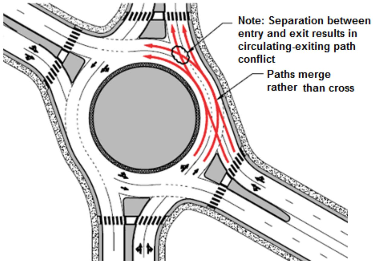
Figure 3.16 – Exit–Circulating Conflict Caused by Large Separation between Legs (Source: NCHRP 672<sup>2</sup>)
