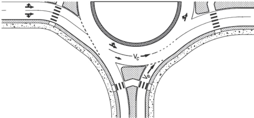
**Figure 2.7 – Typical one-lane entry conflicted by two circulating lanes (Source: HCM 2010<sup>3</sup>)**
