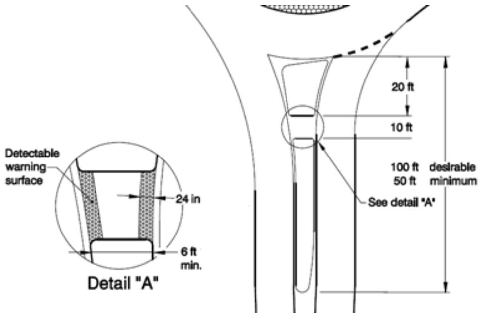
Figure 3.10 – Typical Minimum Splitter Island Dimensions (Source: NCHRP 672<sup>2</sup>)
