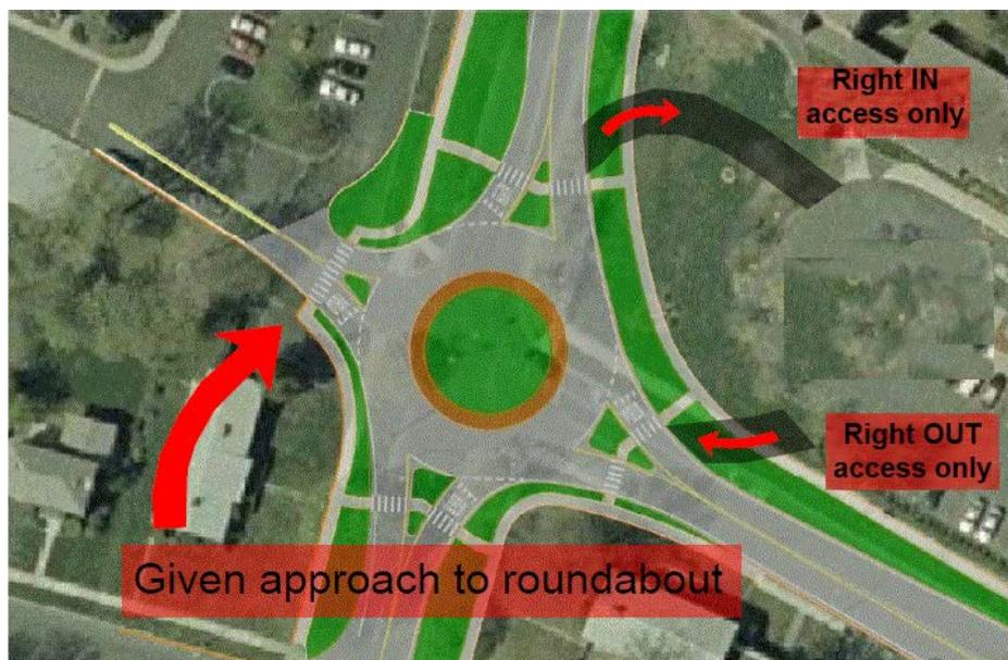
Figure 3.60– Commercial Driveway as Approach Leg to circulatory roadway (Source: NYSDOT<sup>14</sup>)
