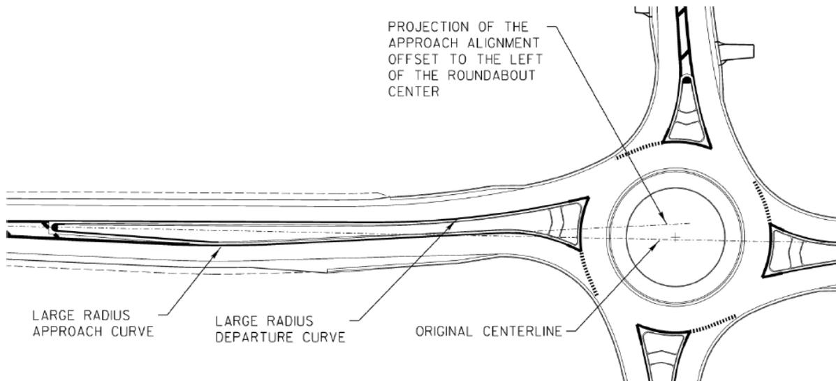
**Figure 3.4 – Roundabout Entry Deflection (Source: WisDOT<sup>4</sup>)**
