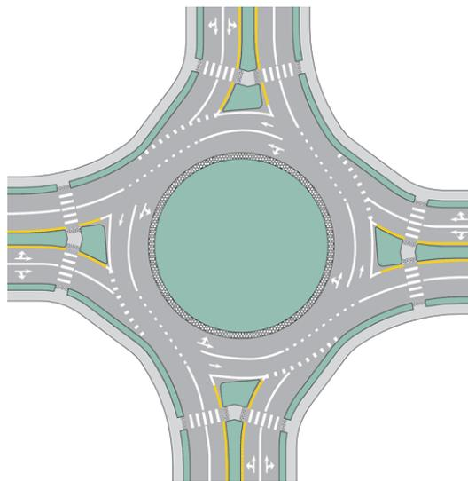
**Figure 4.1 – Typical Pavement Marking Layout for Single Thru/Right lane and Left Turn lane**
