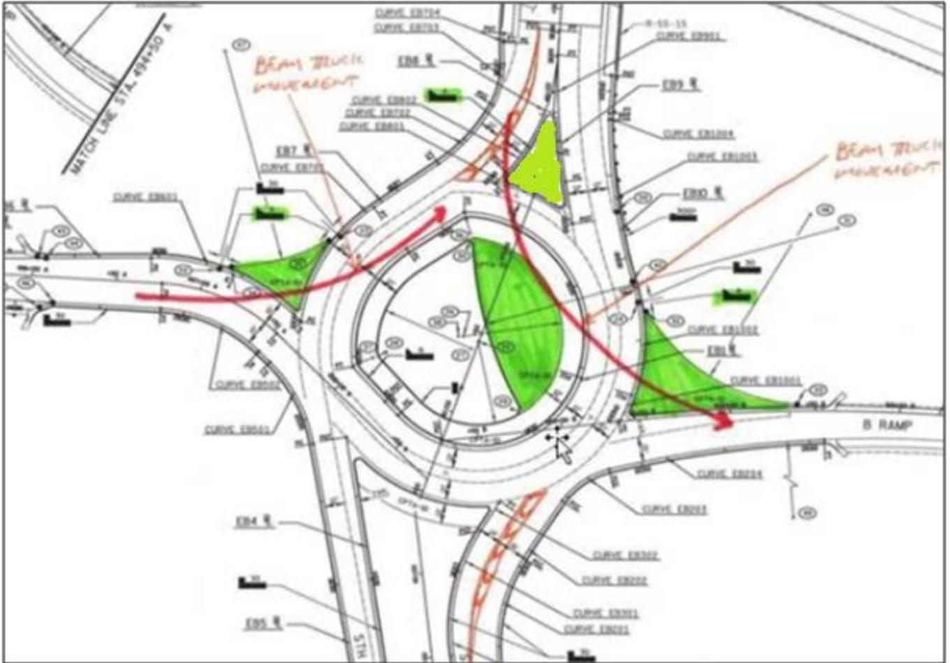
Figure 3.33 – Counter flow OSOW Tuning Movements (Source: Ourston Roundabout Engineering<sup>10</sup>)
