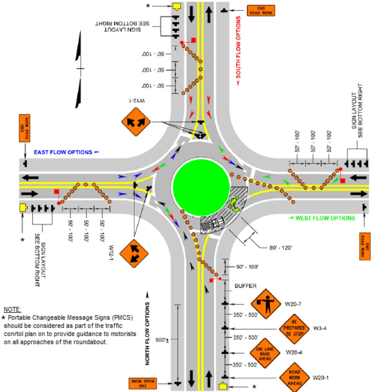
Figure 8.3 – Typical Single-Lane Roundabout Flagging Operation (Source: VDOT<sup>3</sup>)
