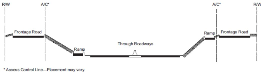
Figure 8-3. Typical Cross Section for Depressed Freeways
