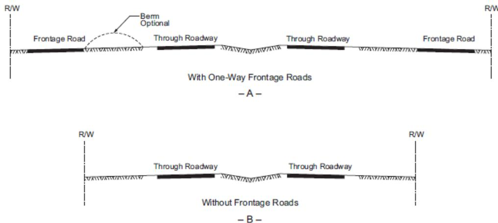
Figure 8-12. Typical Cross Sections for Ground-Level Freeways
