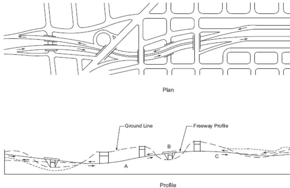
Figure 8-14. Profile Control—Combination-Type Freeway in Rolling Terrain
