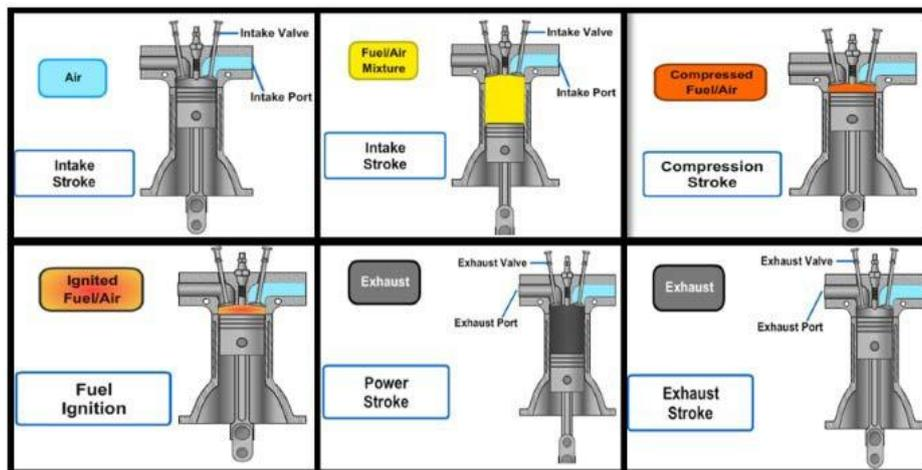
Figure 2-3 - Four-stroke cycle gasoline engine in operation.
