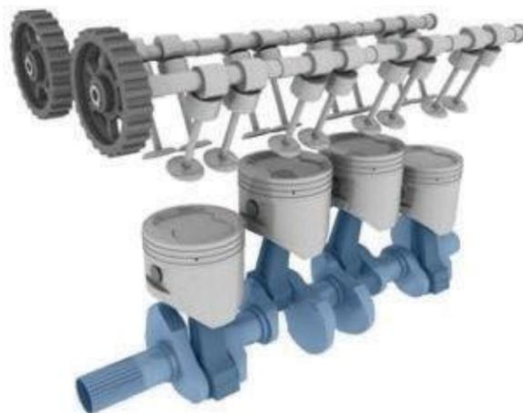
**Figure 2-24 - Dual Overhead Cam.**
