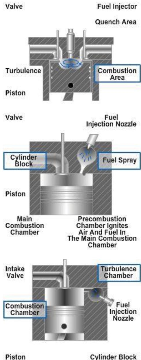
**Figure 2-6 – Direct and indirect injection.**
