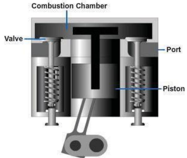
**Figure 2-22 - T-Head engine.**
