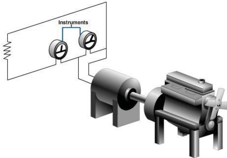
**Figure 2-16 – Engine Dynamometer.**
