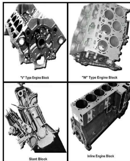
**Figure 2-11 - Cylinder arrangements.**
