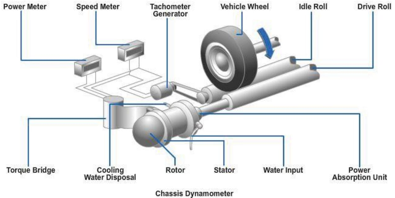
**Figure 2-15 – Chassis dynamometer.**
