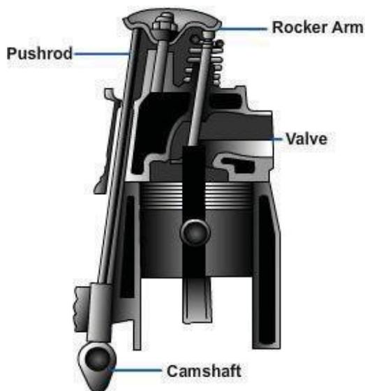
Figure 2-20 - I-Head engine.
