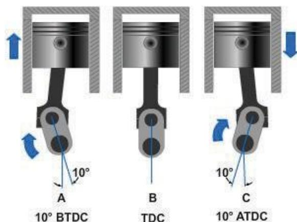
**Figure 2-25 - Engine timing.**
