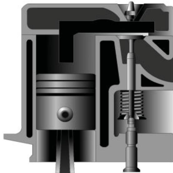
Figure 2-19- L-Head engine.
