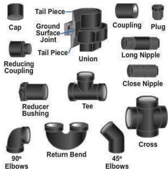
**Figure 9-27 – Threaded pipe connectors.**
