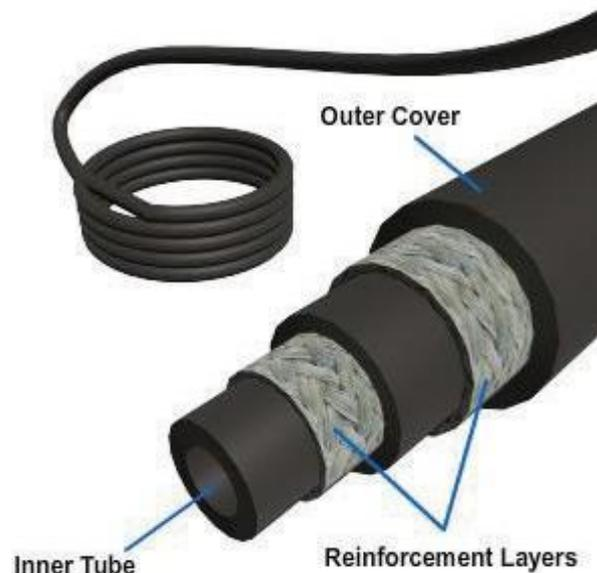
**Figure 9-25 – Flexible rubber hose construction.**
