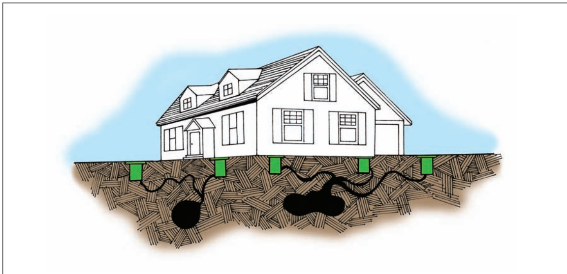
Figure 27. — Bait stations placed along the perimeter of a house (number shown is less than that typically recommended by the manufacturers).
