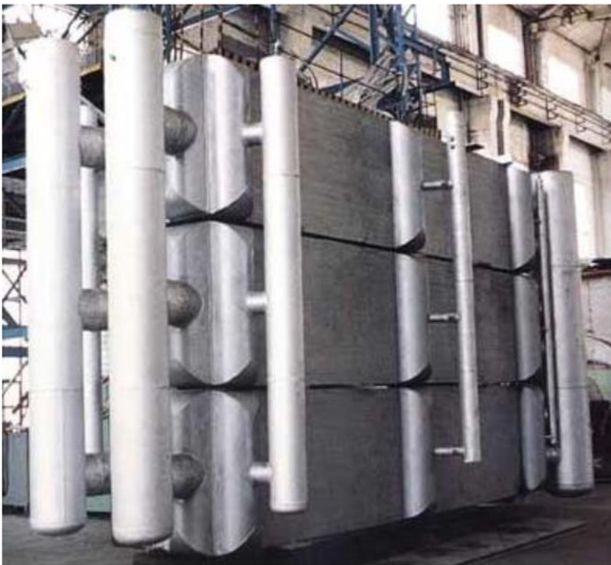
Plate fin heat exchangers typically made of aluminum and brazed together Source: http://webwormcpt.blogspot.com/2010_07_01_archive.html
