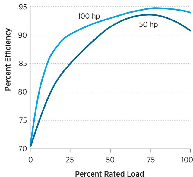
Figure 4. Typical motor part-load efficiency curve
