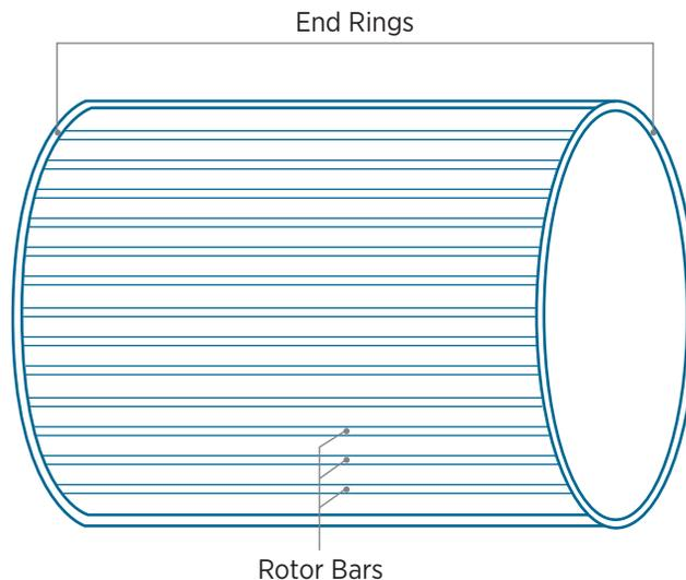
Figure 3. Squirrel-cage rotor
