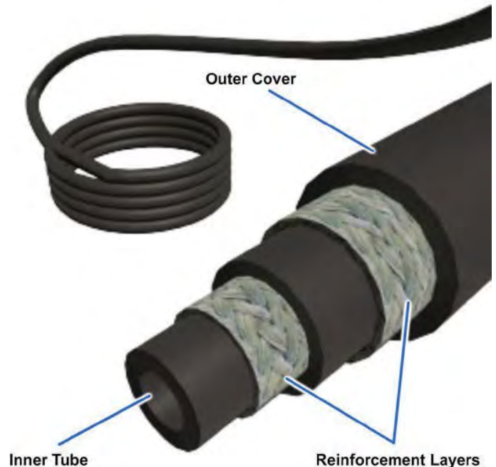
Figure 9-49 — Flexible rubber hose construction.
