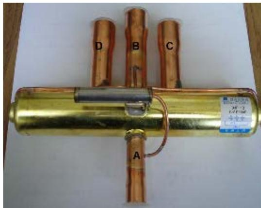
The reversing valve has four ports (A, B, C, and D):
