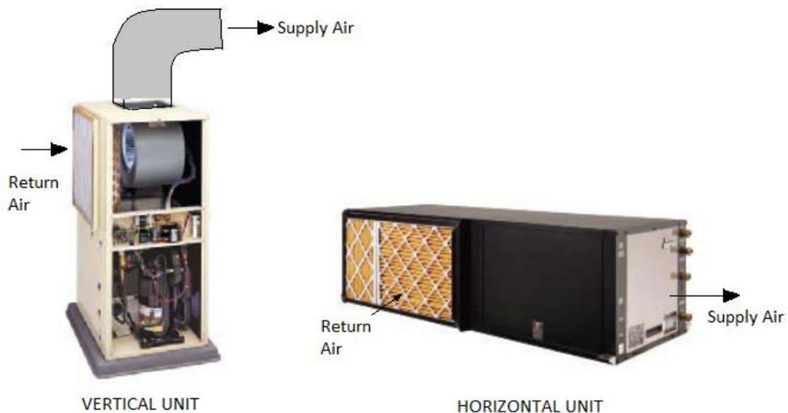
Packaged units contain an integral blower and a heat exchanger section that is connected to the air distribution system. Basic components used in the packaged equipment are the hermetic compressor, co-axial refrigerant-to-water exchanger, a finned coil refrigerant-to-air heat exchanger, a blower motor to circulate the air, and a capillary or refrigerant metering device. The system reverses from the cooling to heating cycles by means of a reversing valve.
