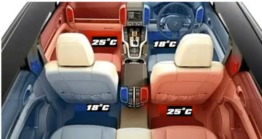
A car equipped in 4-zone system would obviously be expensive because of the presence of additional sensors and a complex electronic control unit.
