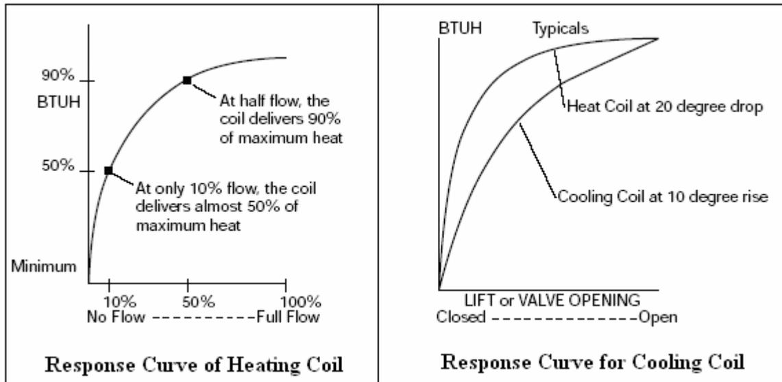
The “convex” shape of the curve means that when the flow increases from zero, the heat emission increases at a high rate in the beginning, but as the flow is increased, the rate of increase decreases. The reason being is that at small flows, the water takes a long time to pass through the coil, so the temperature drop of the water will be large (effective use). Conversely, when the flow is increased, the water spends less time inside the coil and the temperature drop of the water is less.
