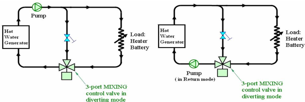
**3 - Port Mixing Valve as Diverting Valve Application**
