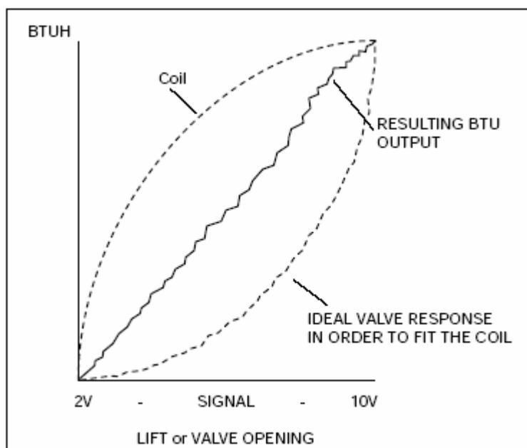
The coil characteristic is “convex” and an equal percent valve characteristic is “concave”. The two complement and counteract each other so that the relationship between the control signal and the heat output is essentially linear. This is only true as long as the valve characteristic is not distorted by a poor valve authority (A). That is, not distorted by
