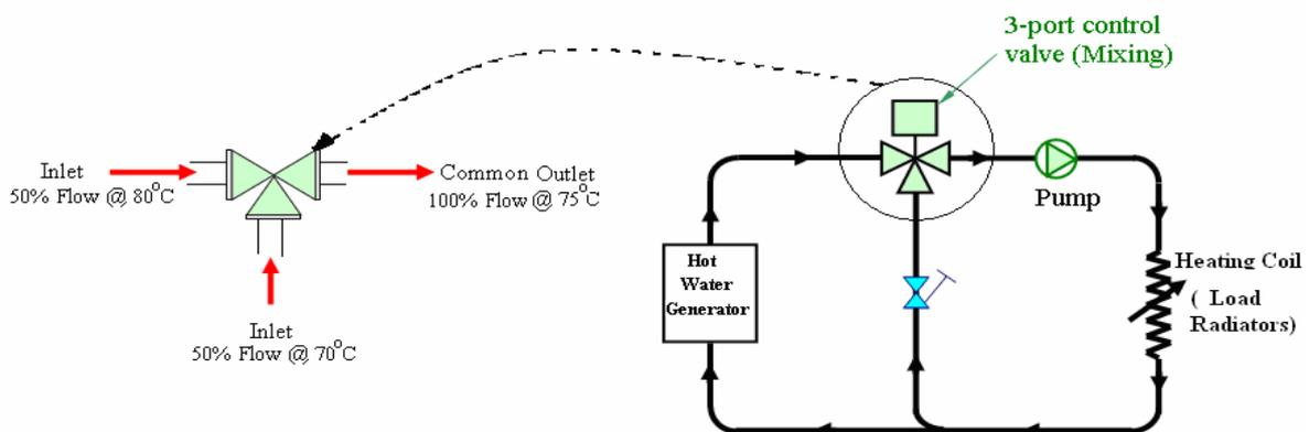
Mixing Valve in Heating Applications
