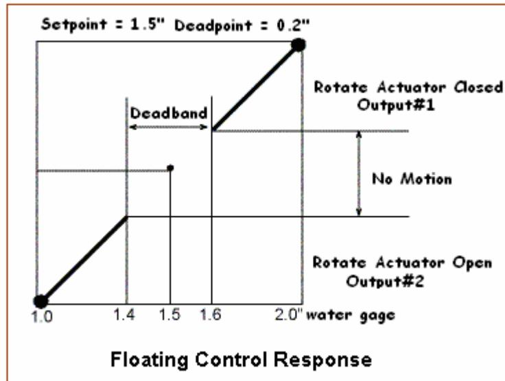
Simple floating controllers are quite satisfactory provided that the controlling thermostat in heating systems is able to sense quickly the effects of the corrective action it produces. The corrective action (movement of a valve or damper) always takes place at the same rate in simple floating control, irrespective of whether the deviation or error signal is large or small.
