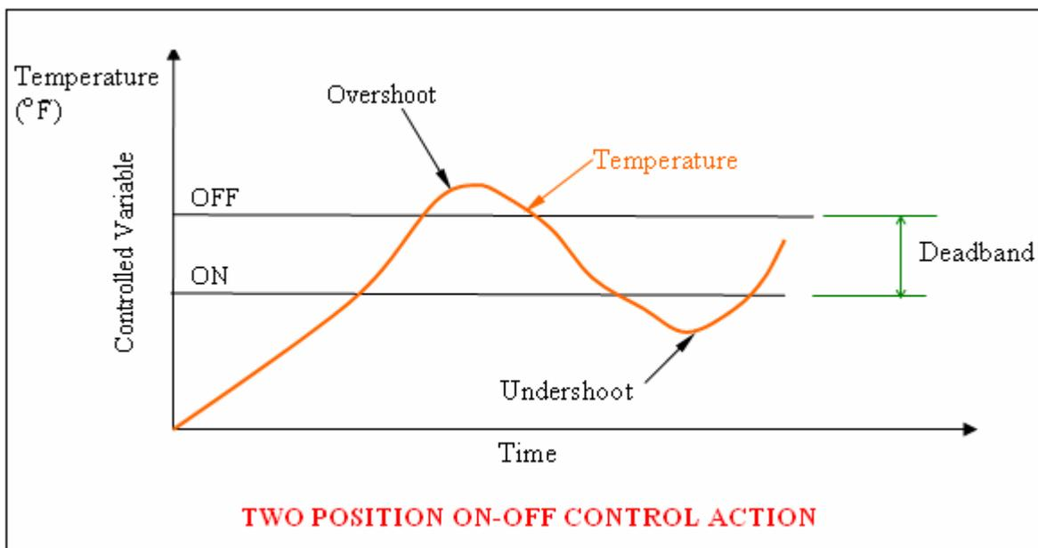
The response curve is always cycling between the two limits 'on' and 'off', and overshoot and undershoot occur in practice due to the thermal inertia of buildings and plants.
