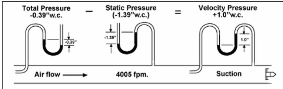
In large ducts an array of sensing devices is required to obtain an average air velocity.
