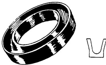
Figure 7-18.—Typical U-cup seal.
