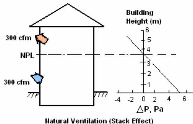
There is a level in a building where the interior and exterior pressures are equal and it is called the neutral pressure level. Below the natural pressure level air infiltration occurs
