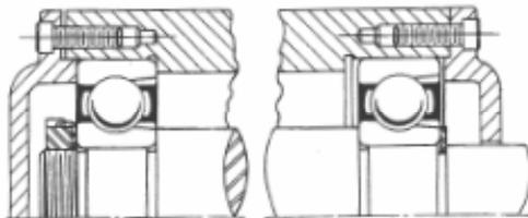
When thrust loads are low, loading groove bearings can be used to take heavy radial loads.
