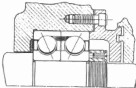
Compliance to high shaft misalignment is accommodated by using two angular contact ball bearings mounted face-to-face.
