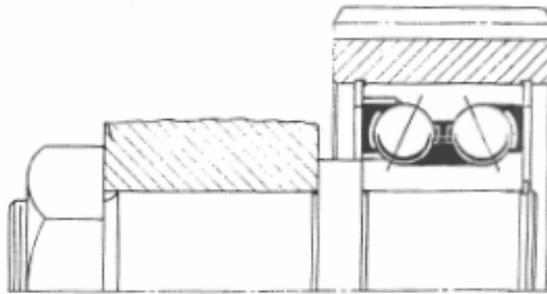
Double row ball bearings with contact angles internally divergent can take heavy overturning moment loading.
