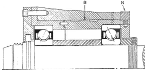
Preloaded Angular Contact Bearings
