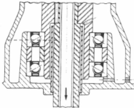
Support of high one-direction thrust loading is accomplished by using two angular contact ball bearings mounted in tandem. The thrust is downward on the shaft.
