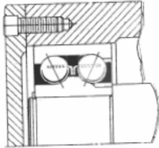
Double row ball bearings with contact angles internally convergent can take misalignment and heavy radial loads.
