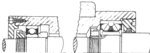
A double row ball bearing is used when reversing thrust loads are present in an application.
