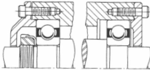
The bearing on the left is clamped to the housing and the shaft. The bearing on the right is free to accommodate shaft thermal expansion and tolerance build-up.
