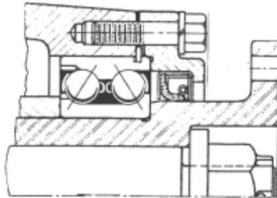
The housing can be thru-bored when a snap ring is used on the bearing outer ring.
