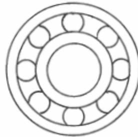
The IR is centered and the balls spaced.
