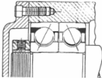
Maximum resistance to high moment loading is obtained by using two angular contact ball bearings mounted back-to-back.
