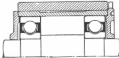
Both bearings can be made to float in the housing if shaft end play is not critical.
