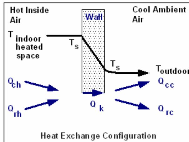
When one side of the wall is warmer than the other side, heat will conduct from the warm side into the material and gradually move through it to the colder side. A temperature gradient is established across the thickness of the wall. The temperature gradient is linear between the two surfaces for a homogenous wall and the slope of temperature gradient is proportional to the resistances of individual layers for a composite structure.
