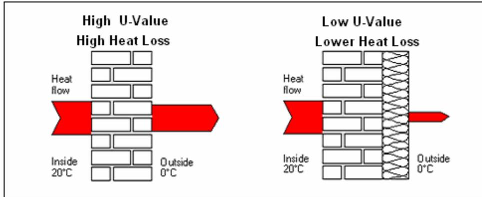
The higher the U-value the more heat flows through so a good U-value is a low one as you want to keep heat inside the building or outside depending on the climate you live in. A house built with low U-value building components will use less energy and thus the building owner saves money on the energy bill. Using less energy is good for the environment.
