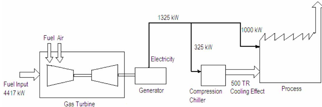
**Schematic Diagram of Power Generation and Cooling with Electricity**
