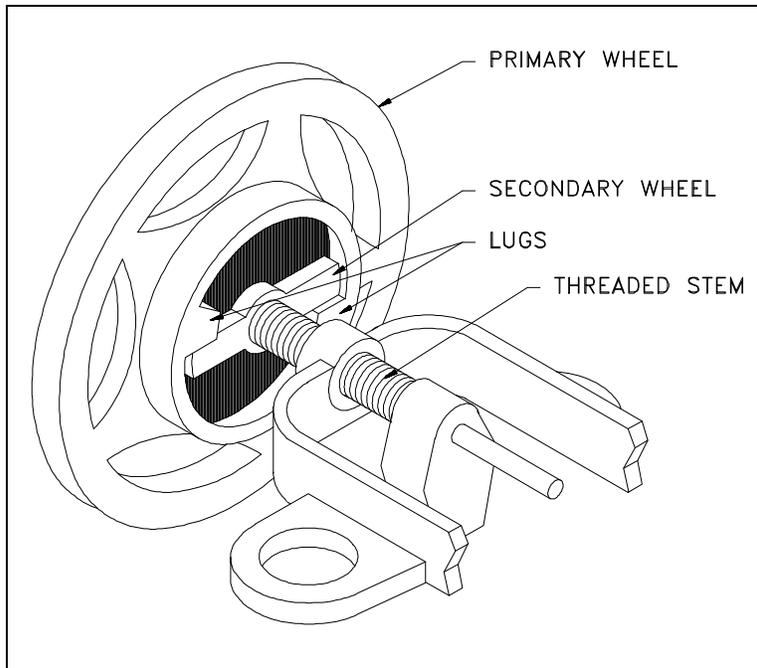
Figure 31 Hammer Handwheel
