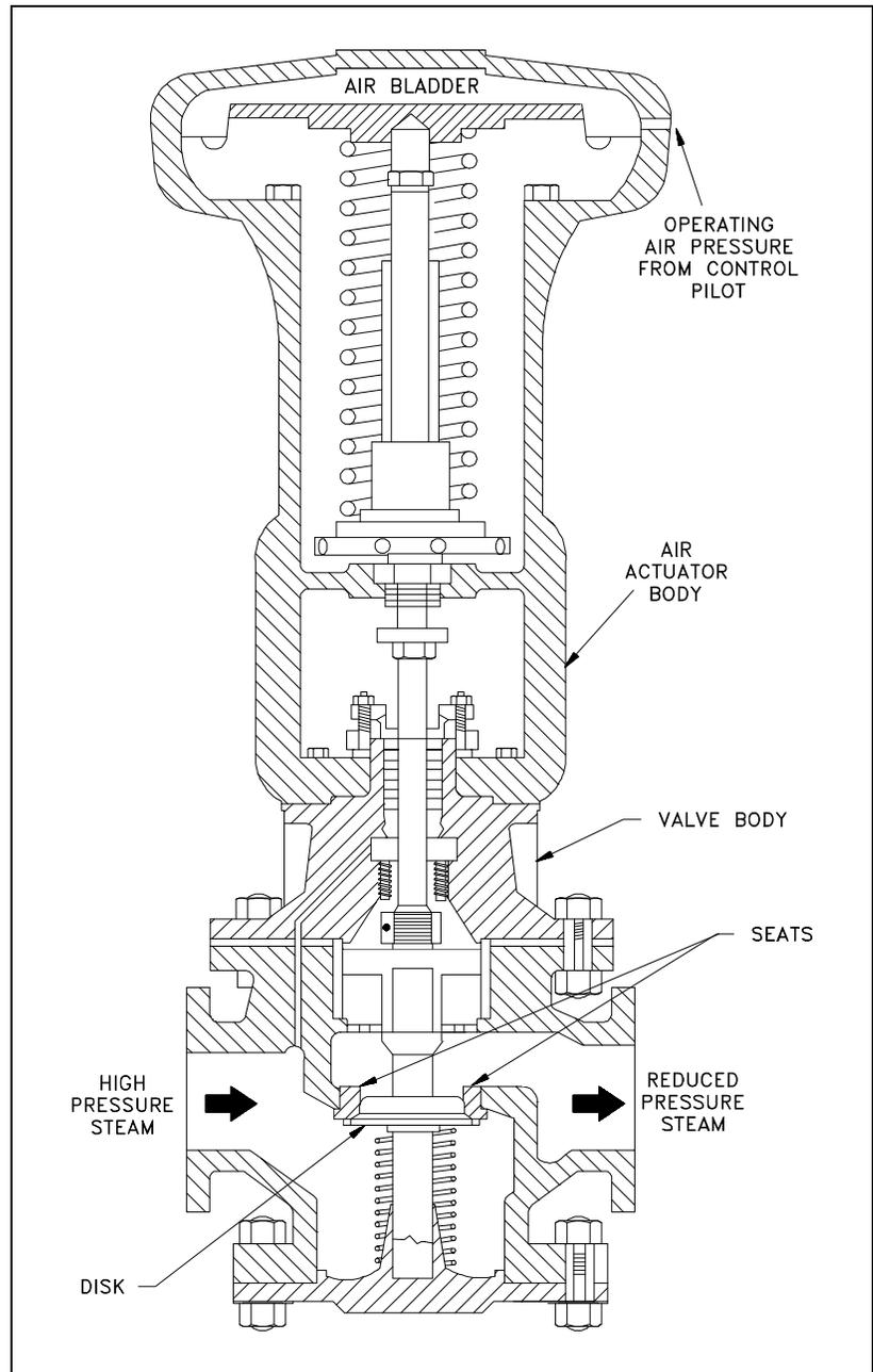
Figure 34 Pneumatic Actuator
