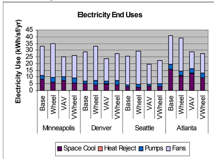
**Figure 2.13 Electricity end uses for the base case and for the base case with an enthalpy wheel (Wheel) and the variable-air-volume system without (VAV) and with an enthalpy wheel (VWheel). Lighting and plug loads are not included.**
