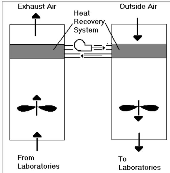
**Figure 2.12** Example of run-around loop energy recovery system.
