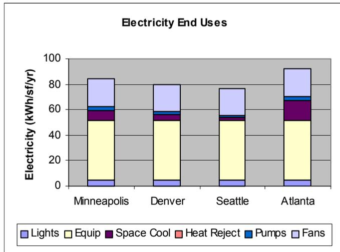
**Figure 4.3 Electricity end uses for the base case.**
