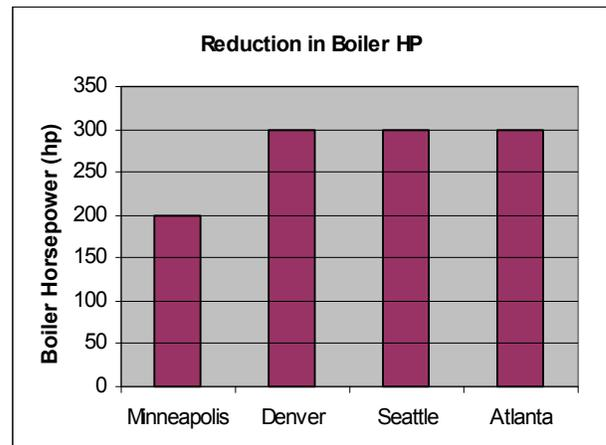
**Figures 2.38a and b Reduction in chiller tonnage and boiler horsepower for enthalpy wheel (Wheel45) with constant-volume reheat system and tighter humidity controls.**
