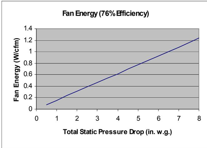
**Figure 2.8 Fan energy with respect to static pressure.**
