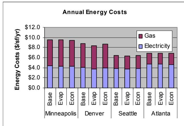
**Figure 2.30** Annual energy costs for the base case, the base case with direct evaporative cooling stage (Evap), and the base case with a water-side economizer (Econ).
