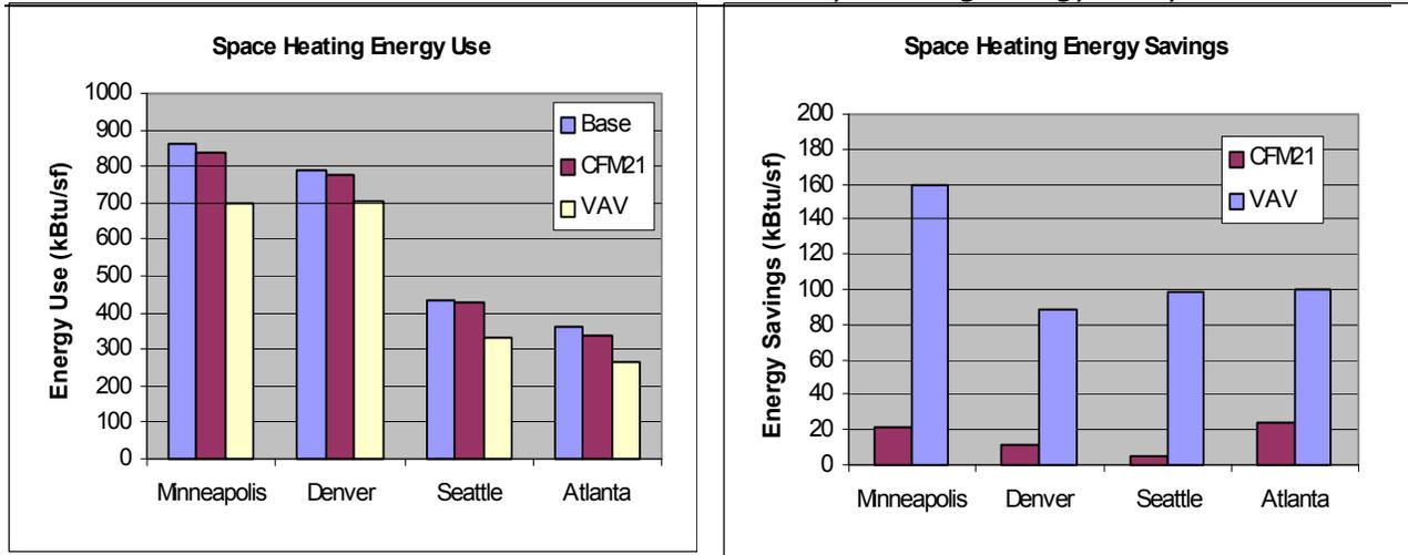
**Figure 2.4a and b Space heating energy use and annual energy savings resulting from reducing space heating energy with flow reduction strategies.**
