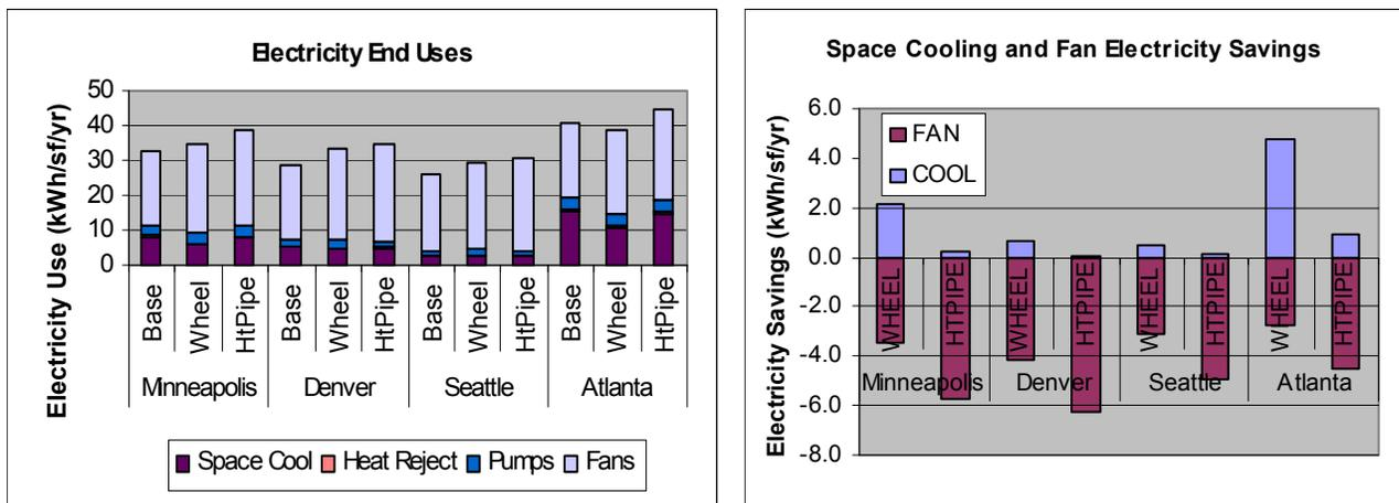
**Figure 2.18a and b Electricity end uses (a) excluding lighting and plug loads for the base case and for the base case with an enthalpy wheel (Wheel) and a heat pipe (HtPipe); space cooling and fan electricity savings (b) for the enthalpy wheel and heat pipes compared with those of the base case.**
