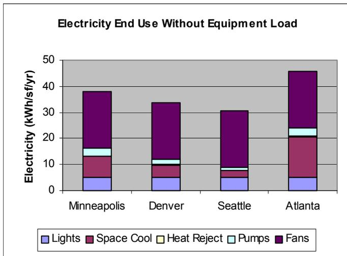
**Figure 1.7 Electricity end uses excluding equipment load.**
