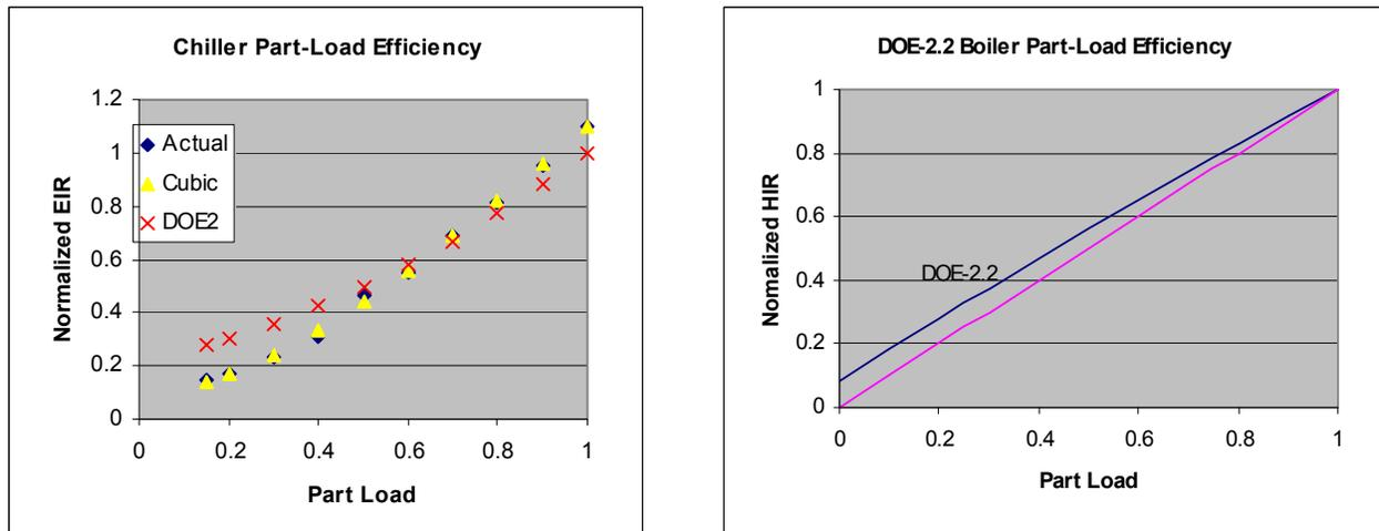
**Figure 1.4 Part-load efficiency curves for chillers and boilers.**
