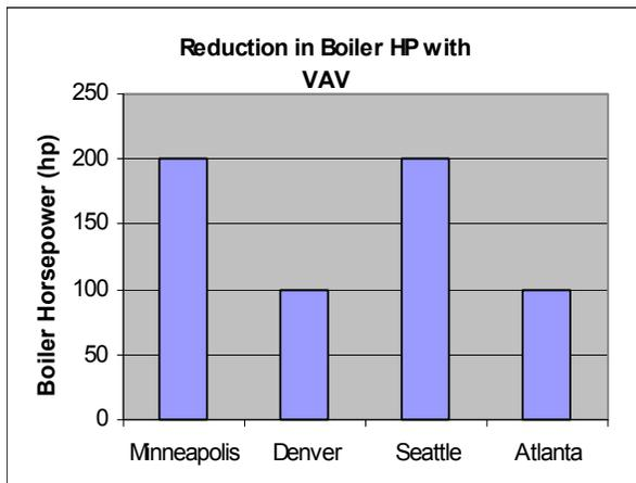
**Figure 2.7 Potential reduction in boiler size with VAV system.**
