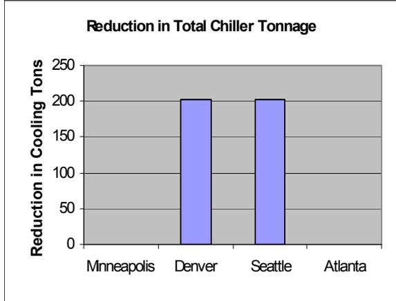
**Figure 2.31 Reduction in chiller size with direct evaporative cooling stage.**
