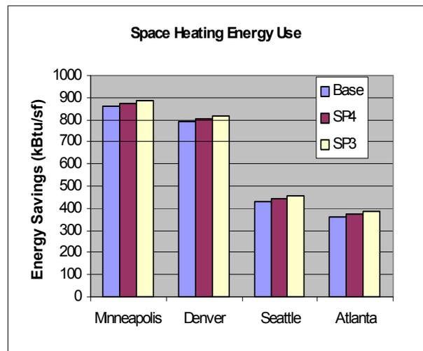
**Figure 2.10 Space heating energy use for the base case, supply static pressure of 4 in. w.g. and exhaust static pressure of 1.5 in. w.g. (SP4); supply static pressure of 3 in. w.g. and exhaust static pressure of 1 in. w.g. (SP3).**
