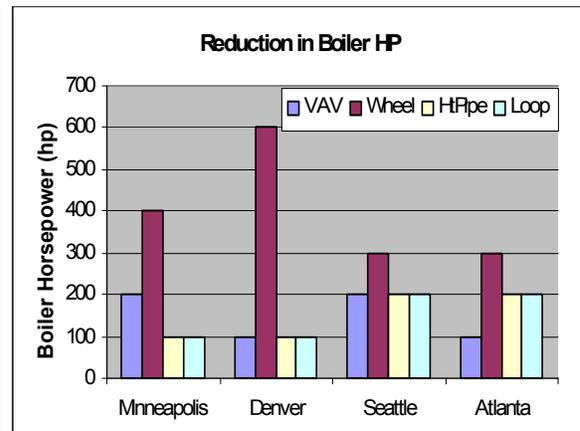
**Figures 2.25a and b Reduction in chiller tonnage (a) and boiler horsepower (b) for enthalpy wheel (Wheel) and run-around loop (Loop) with base case constant-volume reheat system. Boiler reduction with VAV is also shown.**
