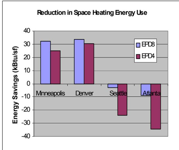
**Figure 2.42 Space heating energy savings for lower plug loads of 8 W/sf (EPD8) and 4 W/sf (EPD4).**
