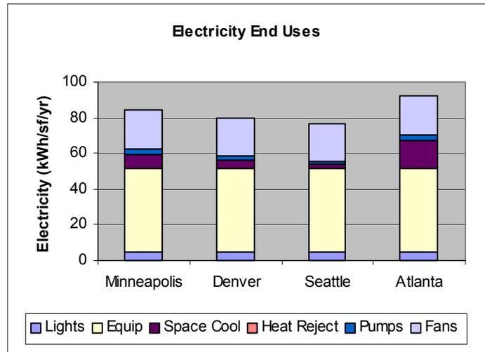
**Figure 1.6 Electricity end uses in all climates.**
