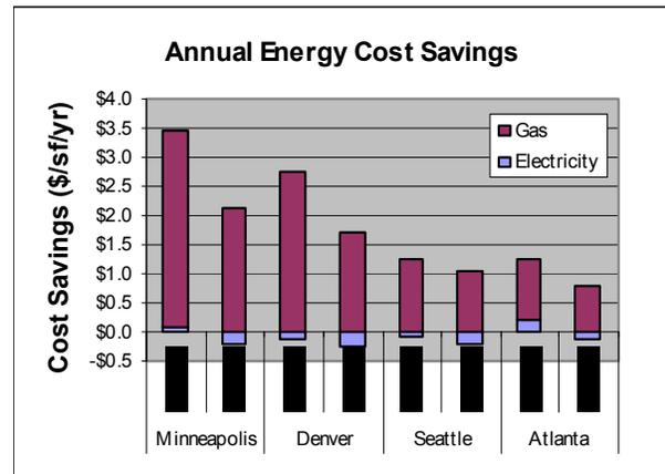
**Figure 2.20a and b Annual energy costs (a) for the base case and the base case with an enthalpy wheel (Wheel) and heat pipes (HtPipe); energy cost savings (b) for the enthalpy wheel (Wheel) and heat pipe (HtPipe) compared with those of the base case.**
