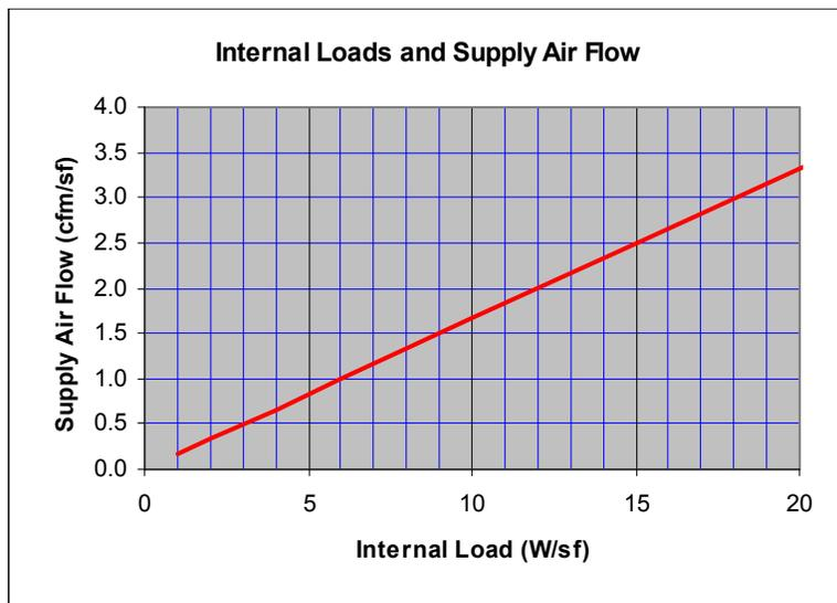
**Figure 1.13 Supply air flow at 55°F to meet internal loads.**
