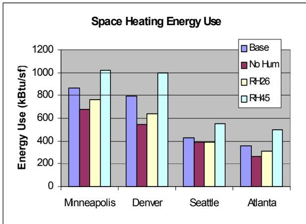
**Figure 2.33 Space heating energy use for the base case and cases with no humidity controls (NoHum), minimum of 20% and maximum of 60% (RH26), and minimum of 40% and maximum of 50% (RH45) relative humidity.**
