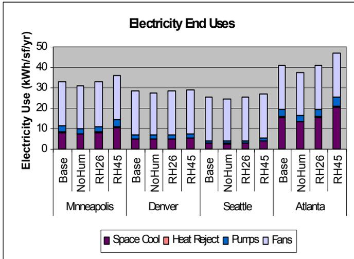
**Figure 2.32 Electricity end uses for the base case and cases with no humidity controls (NoHum), minimum of 20% and maximum of 60% (RH26), and minimum of 40% and maximum of 50% (RH45) relative humidity.**
