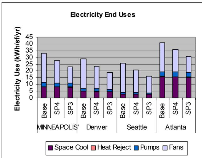
**Figure 2.9 Electricity end uses for the base case, supply static pressure of 4 in. w.g. and exhaust static pressure of 1.5 in. w.g. (SP4), and supply static pressure of 3 in. w.g. and exhaust static pressure of 1.0 in. w.g. (SP3).**
