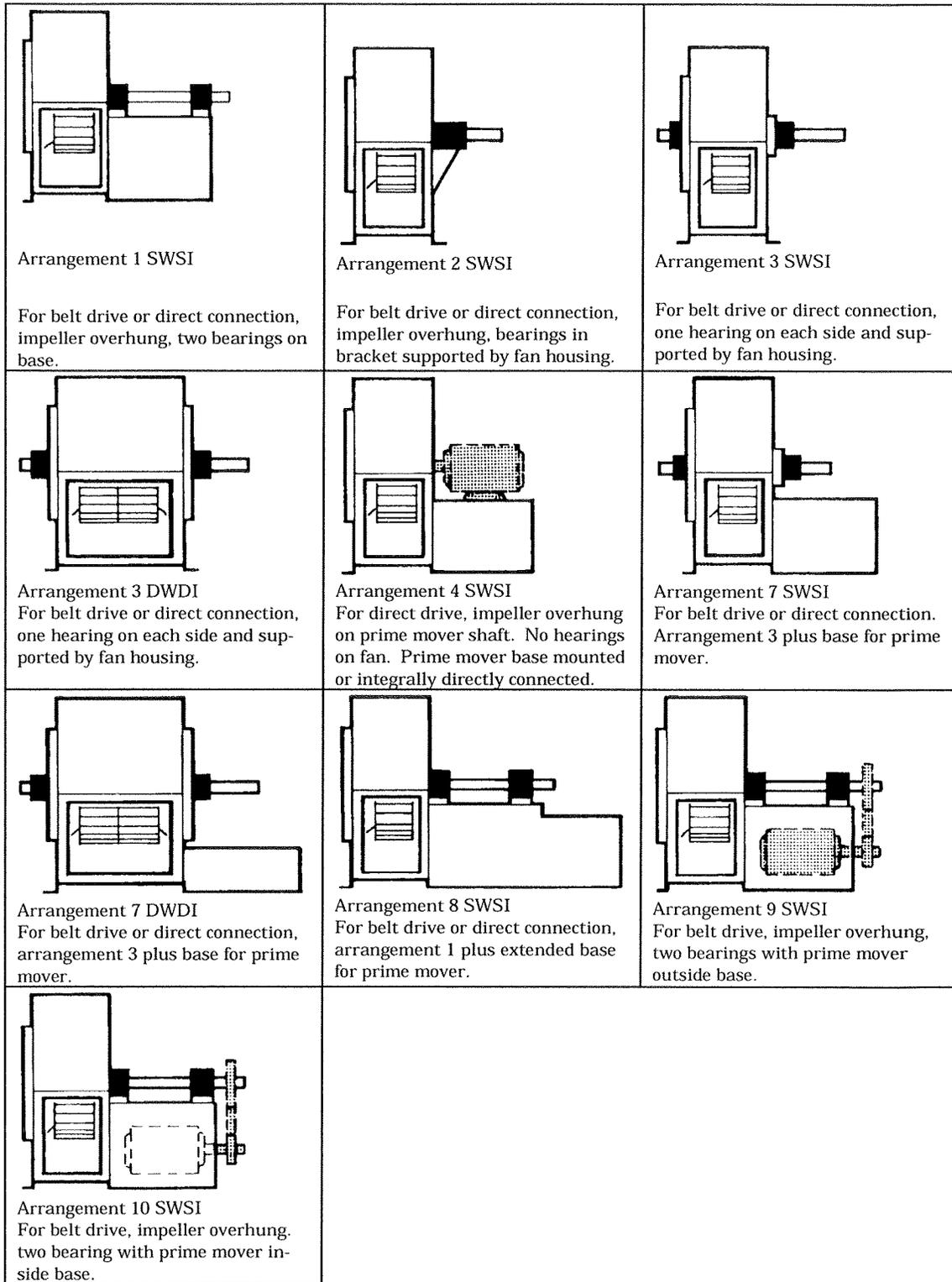
SW - Single Width DW - Double Width SI - Single Inlet DI - Double Inlet
