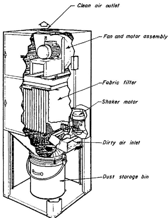
**Figure D-32. Unit Collector.**
