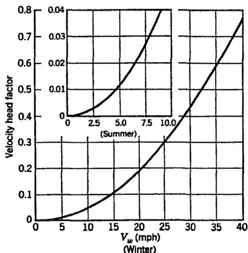
**Part B. Infiltration Rates for Velocity Head Factors**
