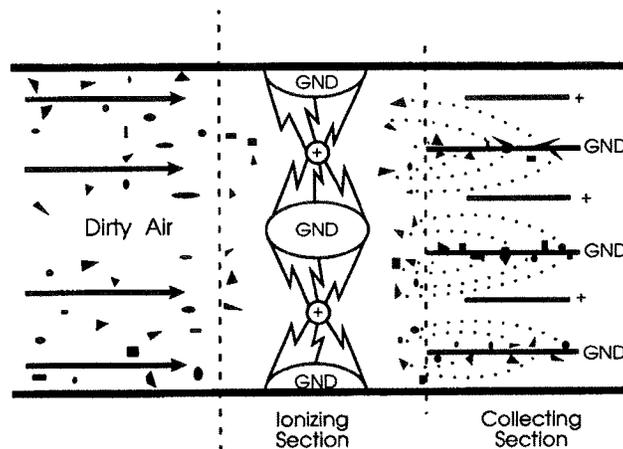
**Figure D-30. Electrostatic Precipitator.**
