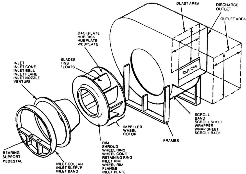
Figure D-10. Centrifugal Fan Components.
