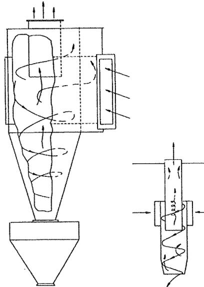
**Figure D-36. High Efficiency Centrifugal Collector.**
