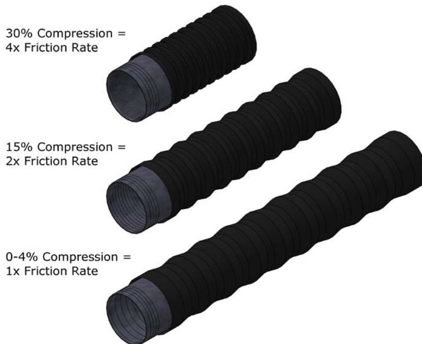
Figure 3. Increased friction rate in compressed flexible duct
