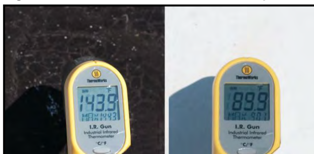
Figure 1: Dark vs. Cool Roof Surface Temperatures
