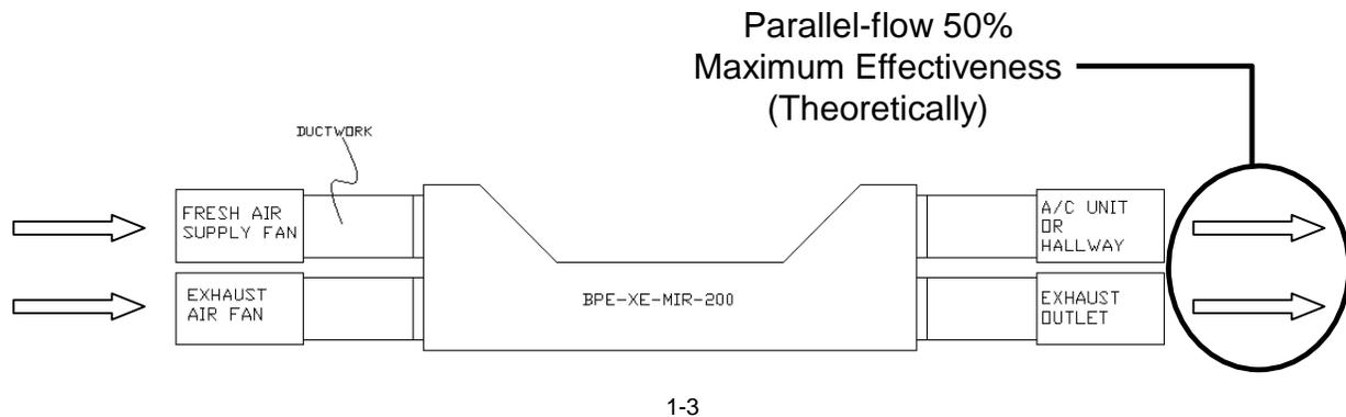
**\*\*\*NOTE:** This is an example of **WHAT NOT TO DO**. If the airflows are headed in the same direction, it will work, but not nearly as efficiently.
