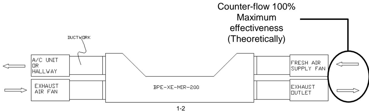
**\*\*Note:** Exhaust and supply airflows should be counter flow for maximum efficiency.
