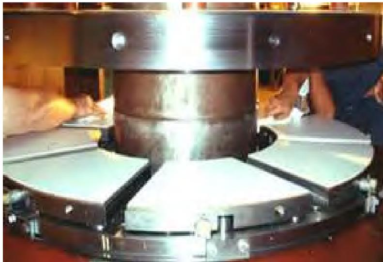
Figure 3-5. Hydropower Tilting Pad Bearings.
