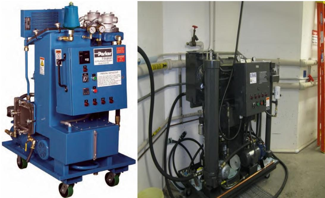
Figure 6-3. Vacuum Dehydrator.
