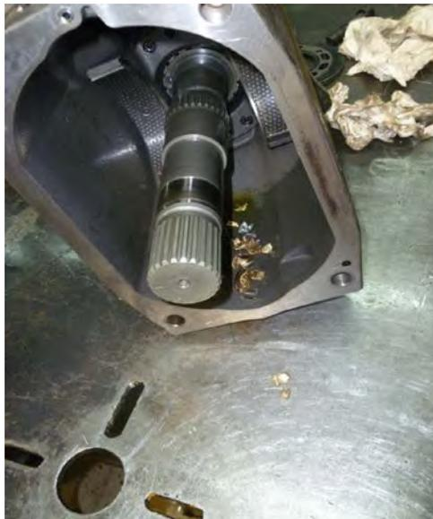
Figure 6-5. Cavitation Damage on a Hydraulic Pump.
