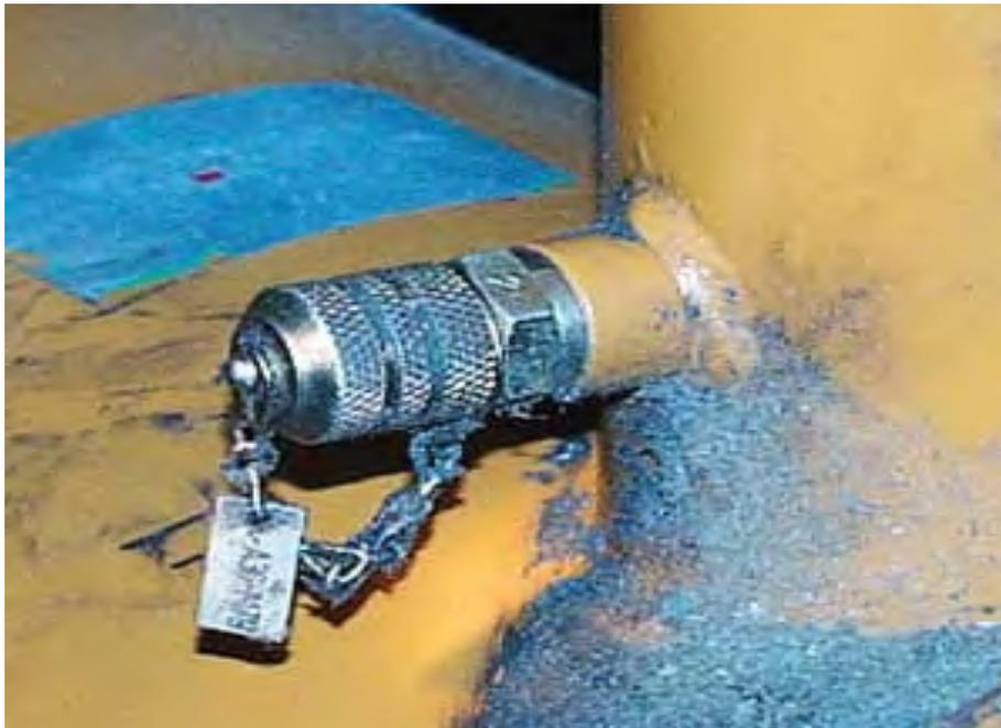
Figure 7-4. Minimesse sample Valve.
