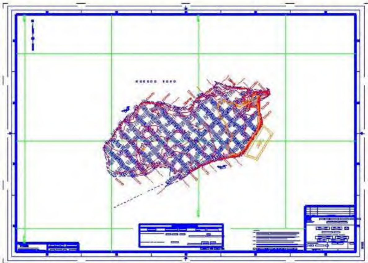
Figure L-3 Line spacing and alignment layout for hydrographic surveys of Almond reservoir. (TVGA, Inc.)
