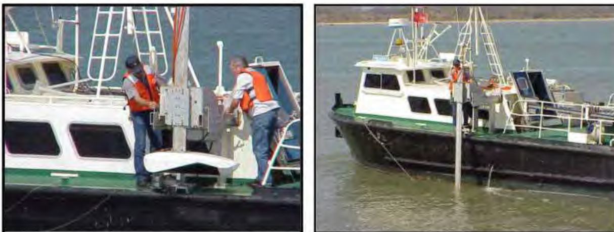
Figure 6-14. Side mounted multibeam transducer on S/V Vollert. (Galveston District)
