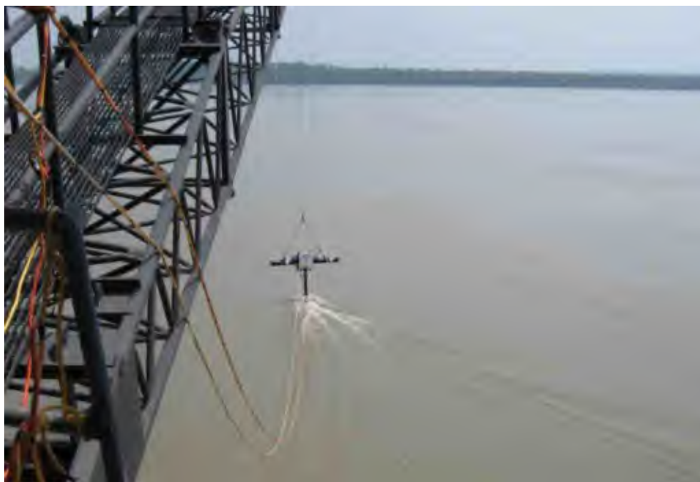
Figure N-19. Multibeam transducer deployed from crane on Low Sill Structure.
