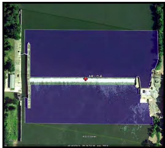
AR Lock & Dam # 6 Survey Coverage Area
