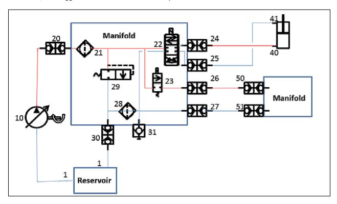
Begin with 1 at the reservoir. Assign a number to each valve or component in sequence in a manifold. It is suggested that you leave a block of numbers unused at the end of each manifold or end device for later addition of components you don't yet know you need. I have found it very helpful to build a spread sheet or data base sheet identifying each component by number, manufacturer and part number, and rated or expected performance.
