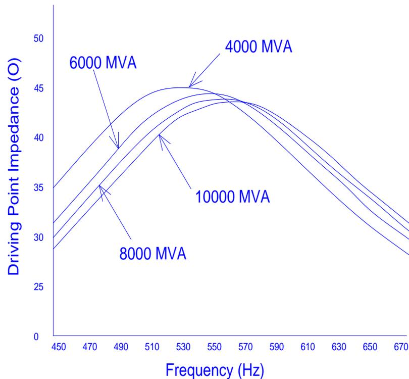
Figure 20. Variations in frequency response at 33 kV bus as a function of capacitor bank size
