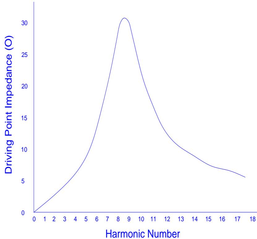
Figure 11. Driving point impedance at 33 kV bus
