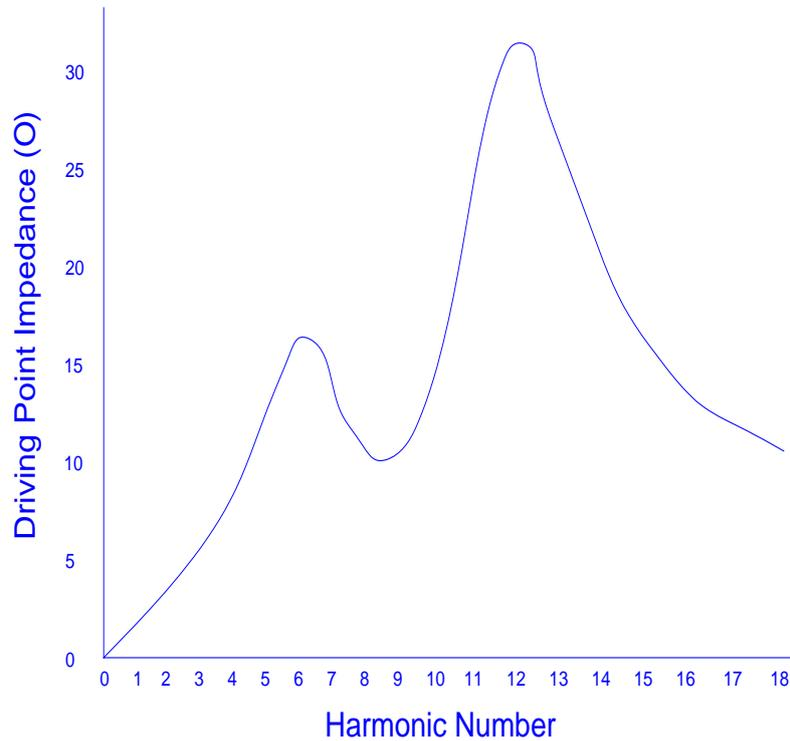
Figure 16. Driving point impedance at 33 kV bus
