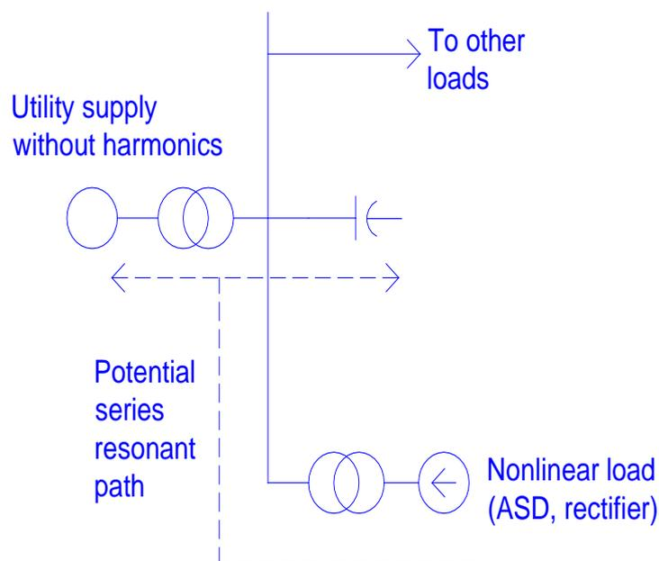
Figure 7. Possible parallel resonant circuit: Plant harmonics
