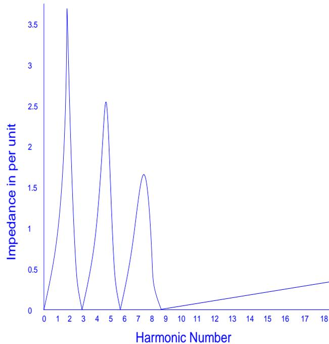
Figure 8. Impedance characteristic of multiple tuned filters
