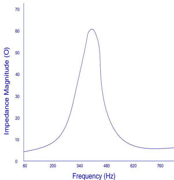
Figure 6. Impedance magnitude vs. frequency for parallel circuits
