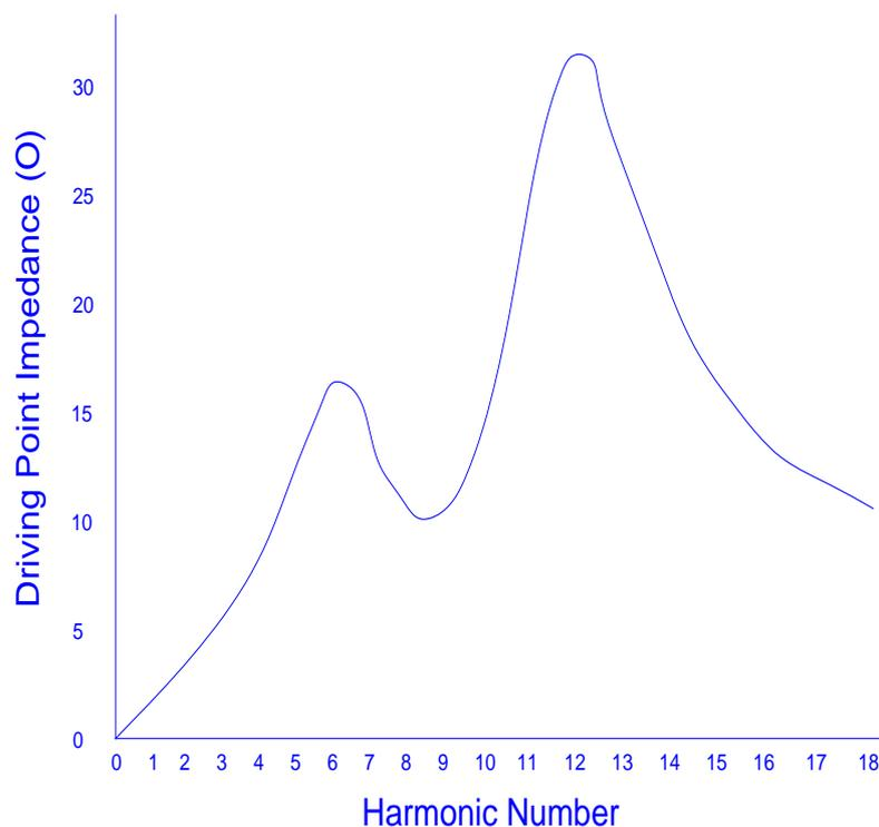
Figure 17. Driving point impedance at 6.6 kV bus7
