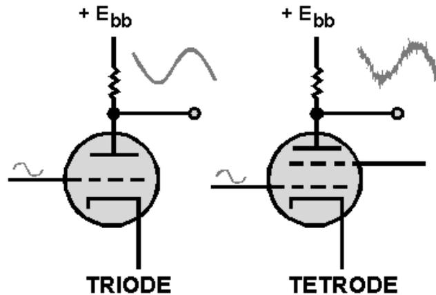
**SECONDARY EMISSION** of electrons from the plate is caused by the acceleration of electrons by the screen grid. This causes the performance of a tetrode to be degraded. In addition to reduced amplitude, the output signals become noisy.
