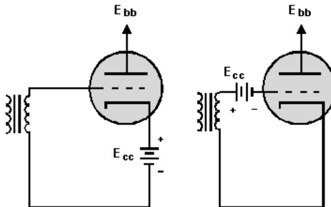
The **OPERATION OF A TRIODE** depends on the ability of the control grid to either increase or decrease conduction through the tube in response to an ac input signal. The output voltage is developed across the tube between the cathode and plate because of the voltage drop across the plate-load resistor changing as the plate current responds to the input signal.
