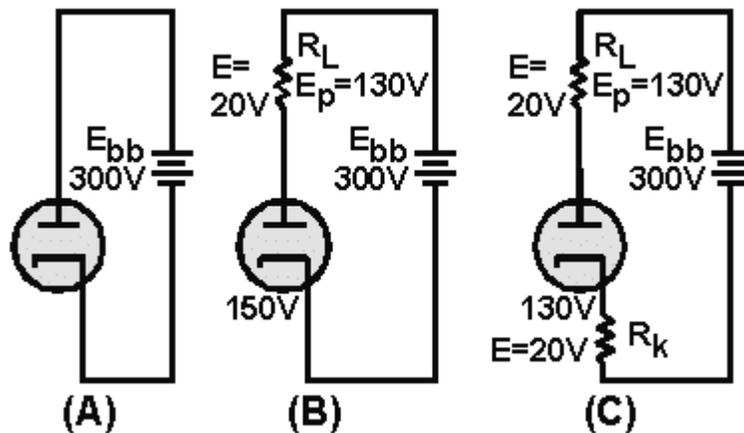
Figure 1-24.—Loss due to cathode biasing.
