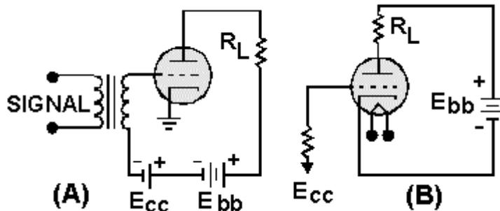
Figure 1-21.—Fixed bias: A. Battery B. Conductor
