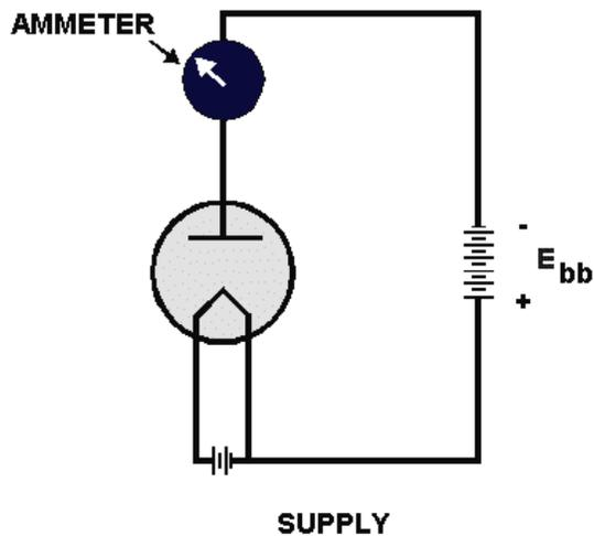
The **CHARACTERISTIC CURVE** for an electron tube is a graphic plot of plate current ( $I_p$ ) versus plate voltage ( $E_p$ ). From this, dc plate resistance can be computed by the formula:
