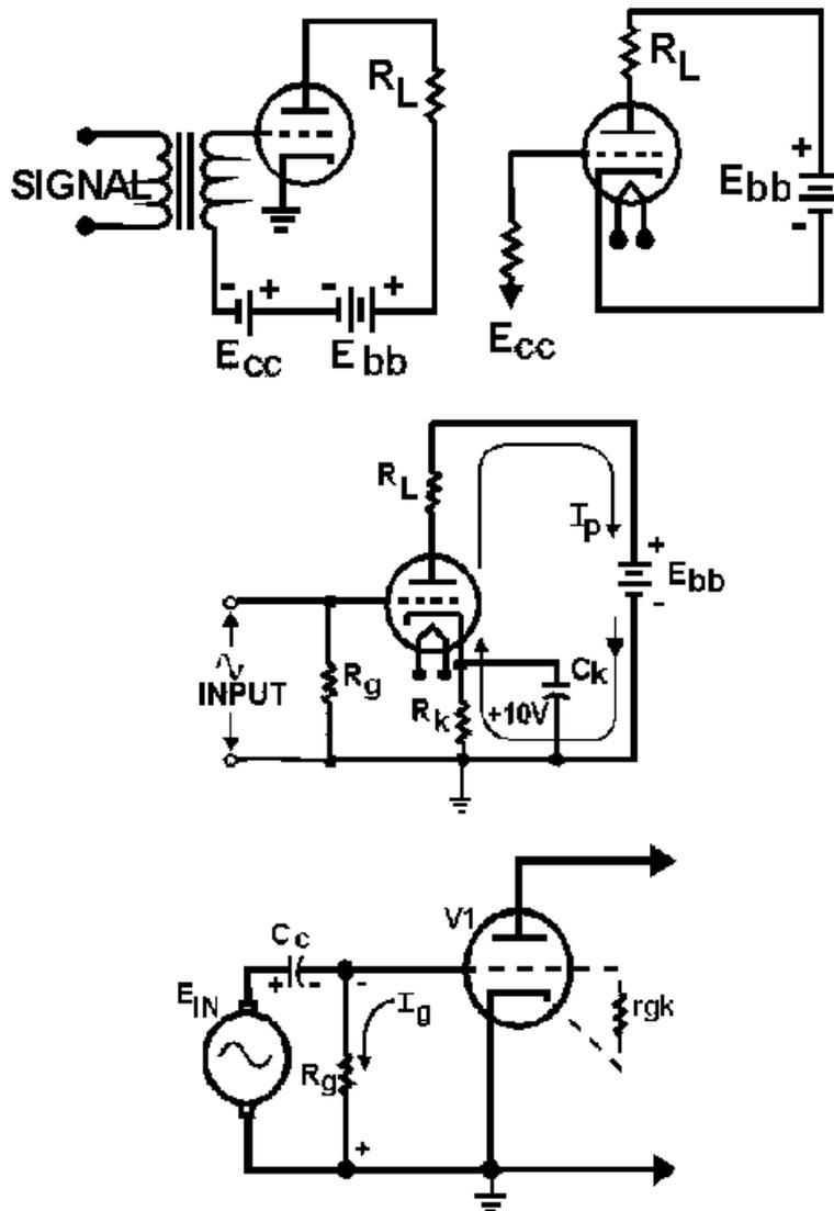
The **CLASS OF OPERATION OF AN AMPLIFIER** is determined by the bias applied to a triode. An amplifier operating as class A conducts continually through the duration of the input cycle. Class AB operation occurs when the amplifier conducts for more than half but less than the entire duration of the input cycle. A class B amplifier conducts for only 50% of the input cycle. The class C amplifier conducts for less than half of the input cycle.
