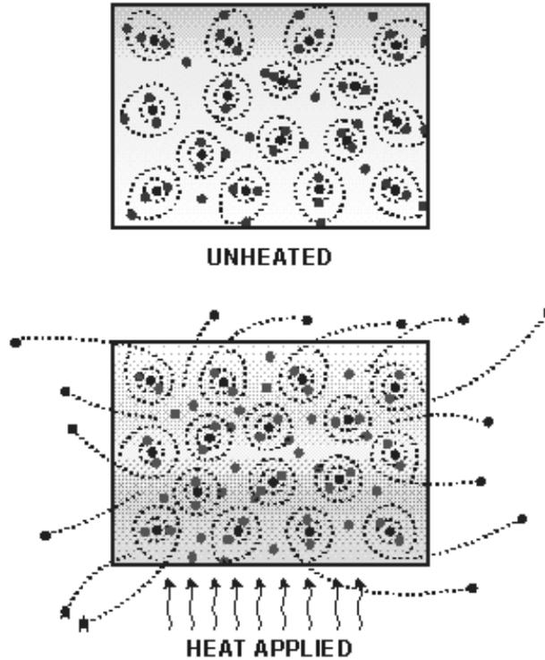
Figure 1-1.—Thermionic emission.
