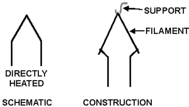
**DIODE OPERATION** depends upon current flow through the tube. Because the cathode is the only electron-emitting element in the tube, current can only flow in one direction, from the cathode to the plate. For current to flow, the plate must be positive relative to the cathode. When the plate is negative relative to the cathode, current cannot flow within the tube.
