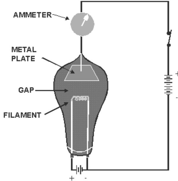
The **CATHODE** is the electron-emitting element of a tube. Cathodes are usually composed of special materials that are heated either directly or indirectly.
