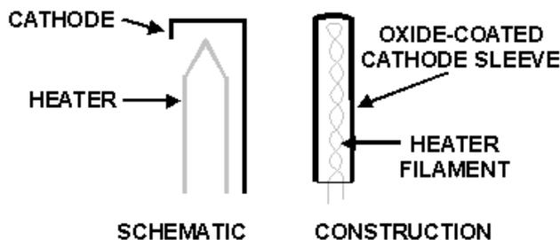
Figure 1-7.—Indirectly heated cathode schematic.
