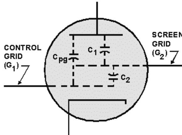
Figure 1-30.—Effect of the screen-grid on Interelectrode capacitance.
