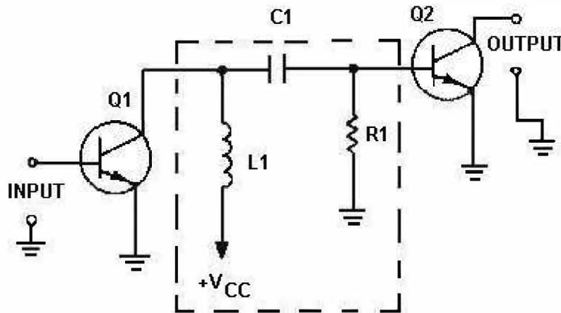
Figure 1-11.—Impedance-coupled transistor amplifier.
