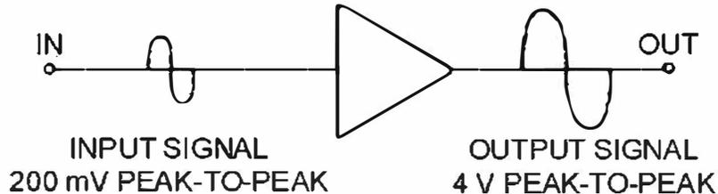
Figure 1-3A.—Block diagram of voltage and power amplifiers.
