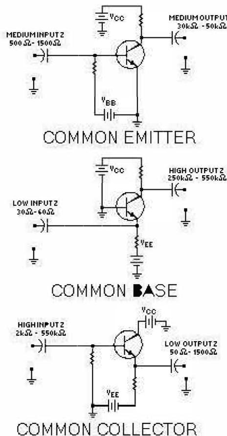
Figure 1-14.—Transistor amplifier configurations and their impedance characteristics.
