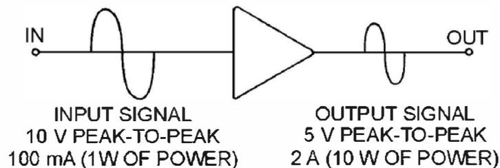
Figure 1-3B.—Block diagram of voltage and power amplifiers.
