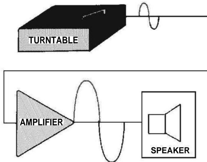
**Figure 1-1.—Amplifier as used with turntable and speaker.**
