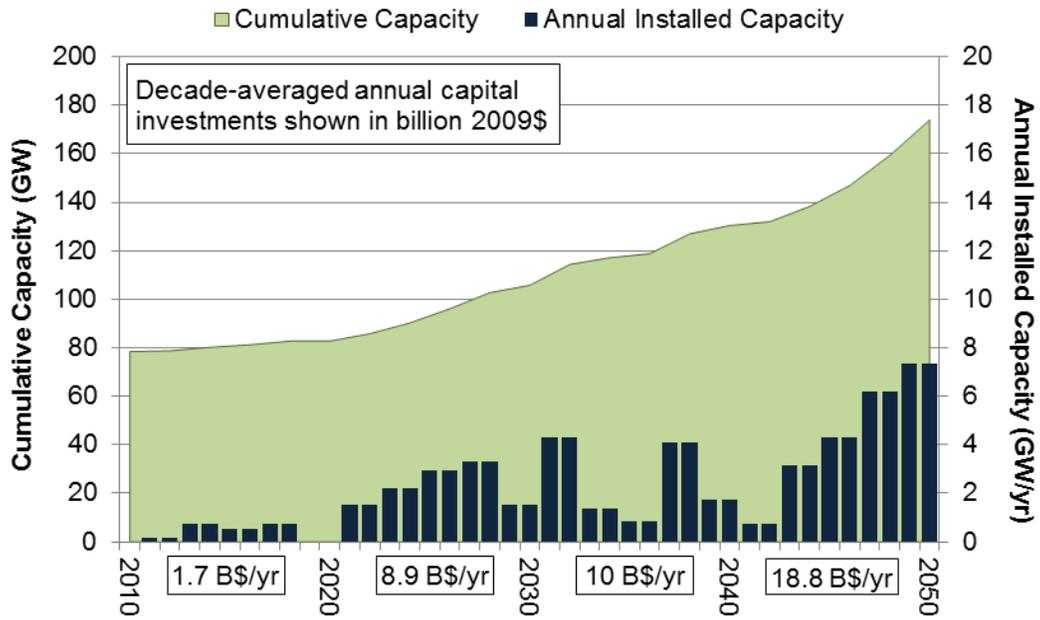
Figure 8-13. Deployment of hydropower in the 80% RE-NTI scenario
