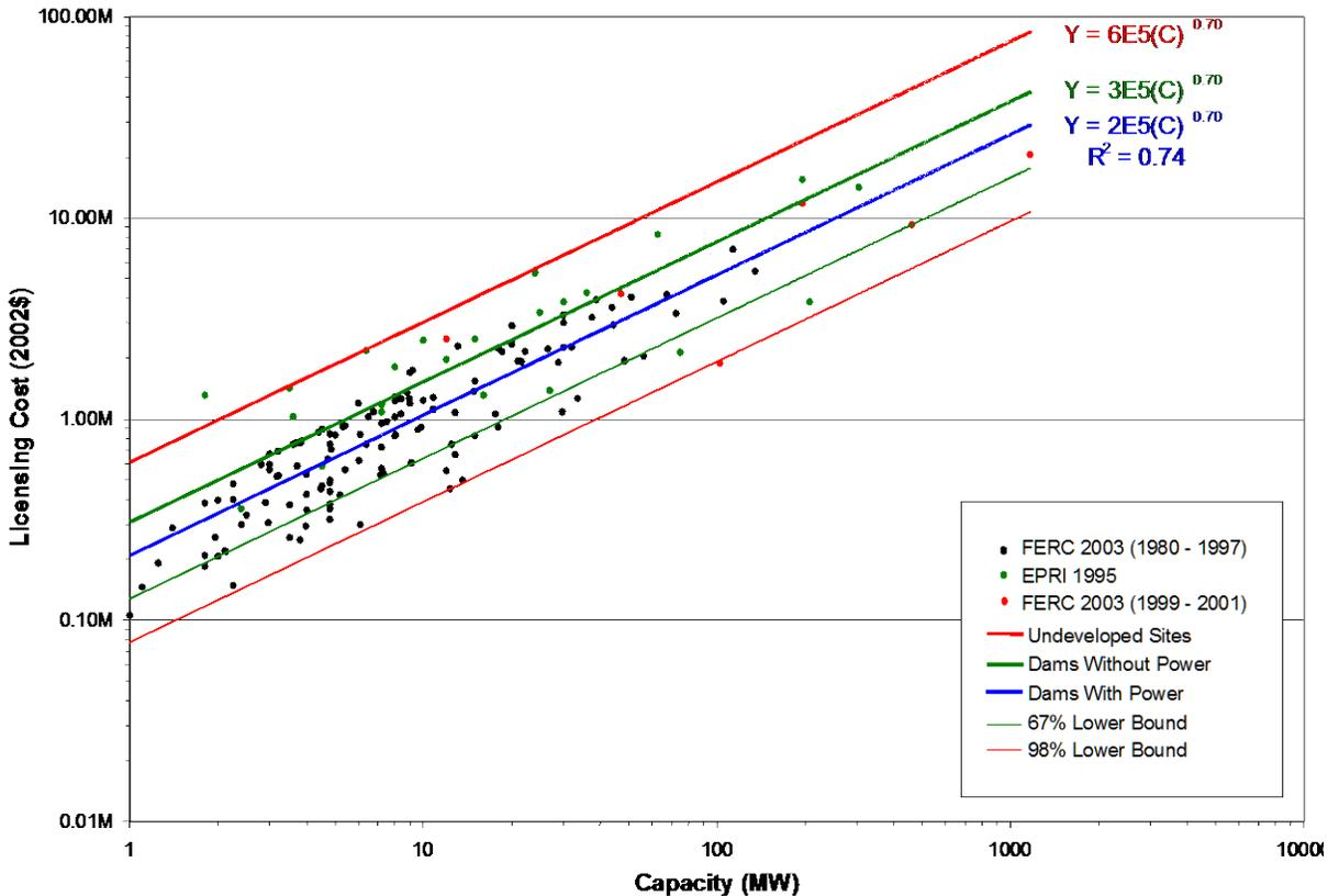
**Figure 8-9. Original operating license cost-estimating curve (2002\$)**
