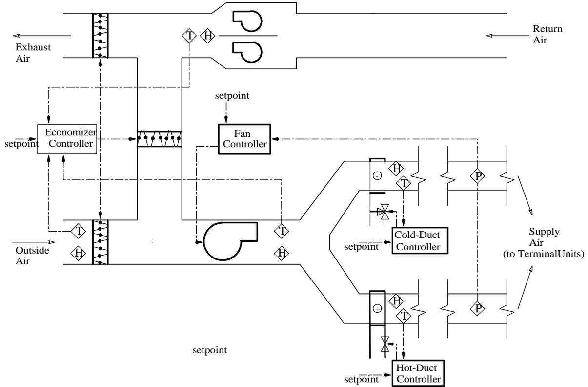
Figure 2: Schematic of the dual-duct air-handling unit.
