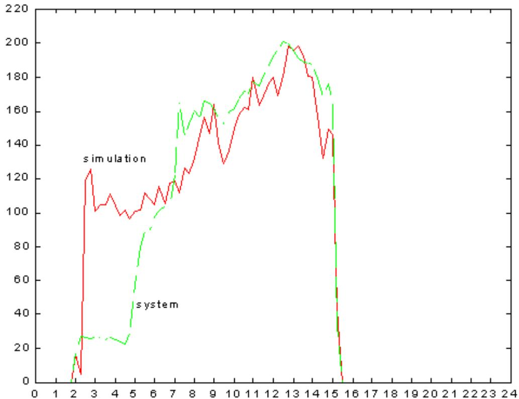
Figure 5: Heat-transfer rate day profile of the cooling coil subsystem.
