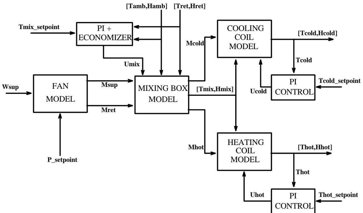
Figure 3: Block diagram of simulated dual-duct air-handling unit.
