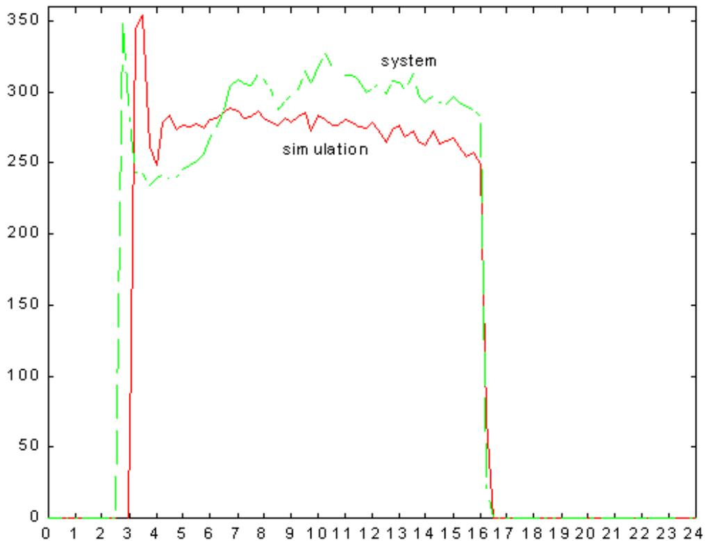
Figure 6: Heat-transfer rate day profile of the heating coil subsystem.
