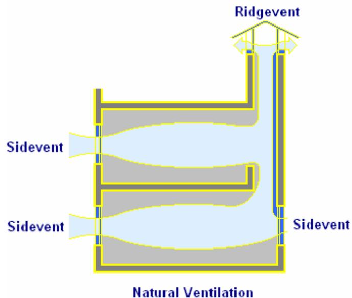
*Natural ventilation and infiltration rates are governed by wind pressure on the building and by internal temperature differences which create an upward movement of warm, buoyant air. Natural ventilation will vary according to the weather conditions, and the ventilation rates are not always predictable or reliable. Natural ventilation may fail altogether in unfavorable conditions of wind and weather, and thus cannot be regarded as a suitable method for all applications.*
