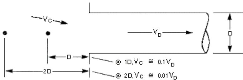
3) **Maximum Capture distance should not be more than 1.5 times the duct diameter.**
