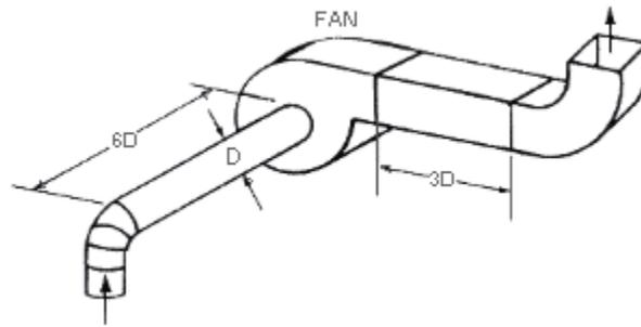
System effect loss is significant if any elbows are connected to the fan at the inlet or outlet. For each  $2\frac{1}{2}$  diameters of straight duct between the fan inlet and any elbow, CFM loss will be 20%.
