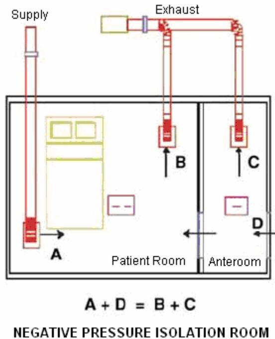
The schematic above shows HVAC air flow arrangement for class N rooms. An anteroom designed to provide an “air-lock” (no mix of air) between the infectious patient and the common space is placed adjacent to the patient room. The air would flow from the ante room to the isolation room. Pressure control is maintained by modulating the main supply and exhaust dampers based on a signal from a pressure transducer located inside the isolation room.
