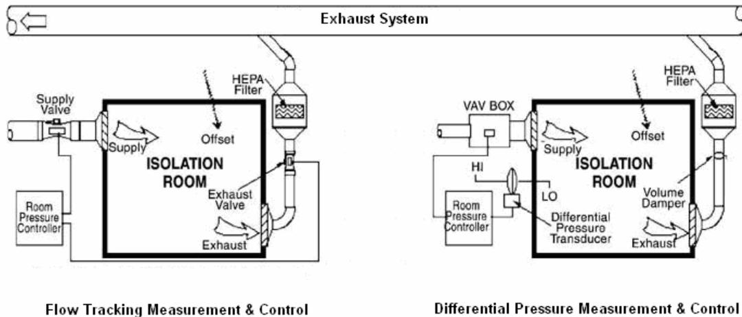
In flow tracking system, the exhaust and supply flow rates “from” and “to” space are measured and controlled to produce a desired infiltration or exfiltration.
